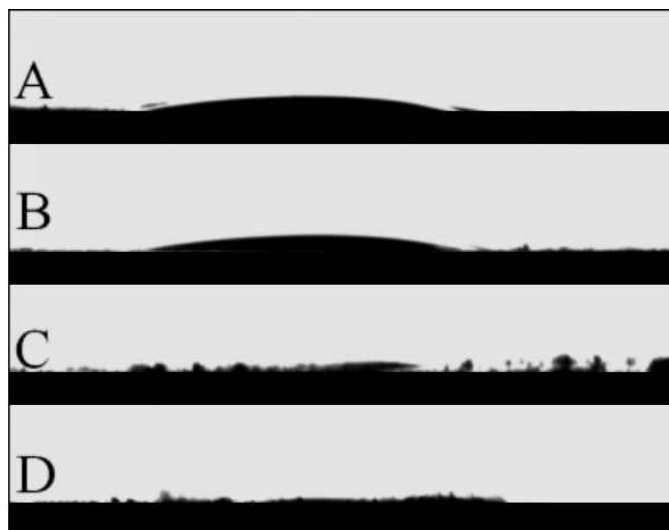
Fig. S5. (A), (B), (C) and (D) are the water contact angle photographs of \text{TiO}_2 , \text{TiO}_2/\text{CNFs} , \text{H-TiO}_2/\text{CNFs} , and \text{NiS/H-TiO}_2/\text{CNFs} after AM 1.5 irradiation, respectively.
