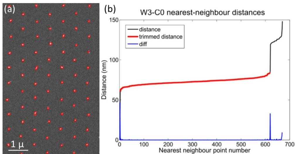
**Figure S1: (a) SEM image of hexagonal CNT array (Wafer 3 C0) viewed from above. The overlaid red ellipses have been generated by particle analysis and their centroids used for the nearest neighbour analysis. (b) Nearest neighbour distances, showing**
