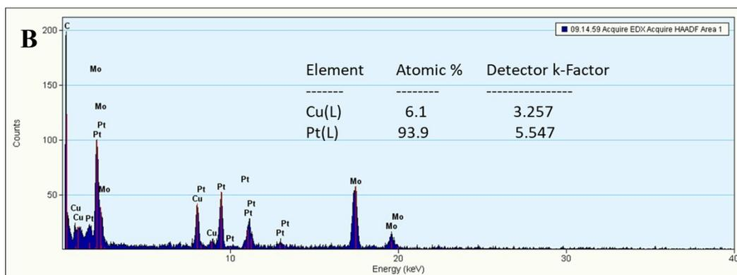
Fig. S6 The EDS spectra of Pt<sub>34.5</sub>Cu<sub>65.5</sub> octahedrons after current-time test (A) and 5000 cycles accelerated durability test (B). (The signals of MO came from Mo grids.)
