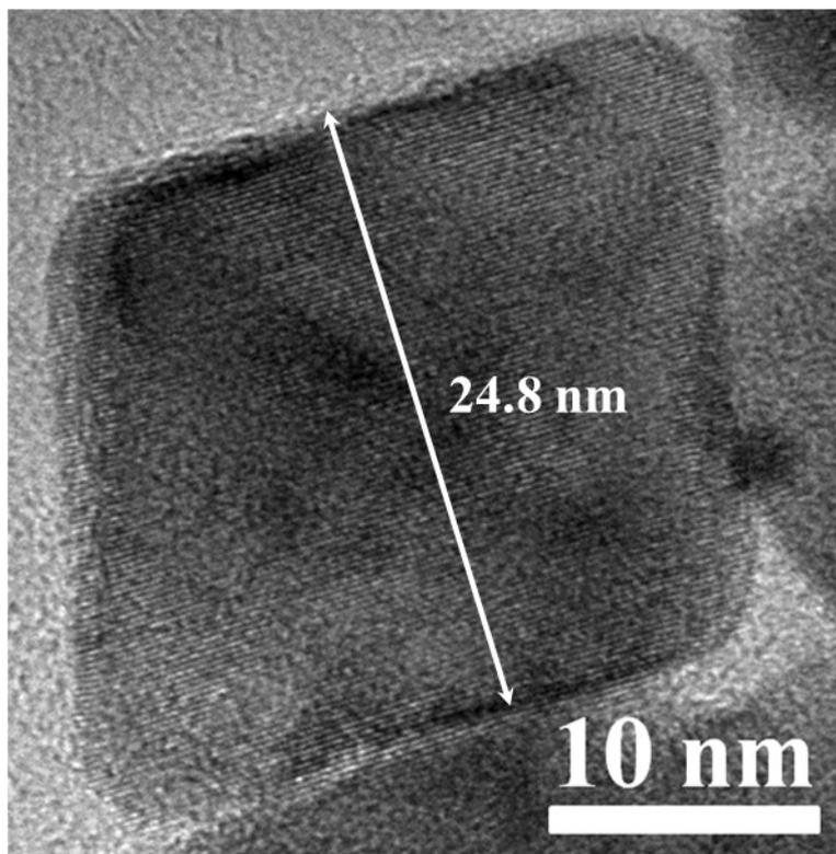
Fig. S2 HRTEM images of the as-synthesized  $\text{Pt}_{34.5}\text{Cu}_{65.5}$  octahedrons.
