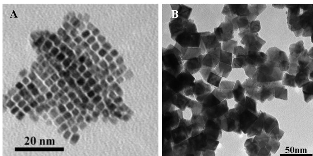
Fig. S1 TEM images of the as-synthesized Pt cubes (A) and Pt<sub>34.5</sub>Cu<sub>65.5</sub> octahedrons (B).
