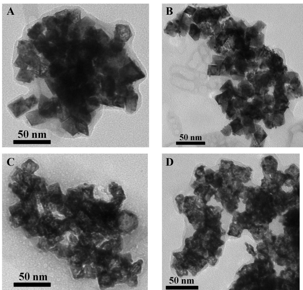
Fig. S5 The TEM images of  $\text{Pt}_{34.5}\text{Cu}_{65.5}$  octahedrons after current-time test (A, B) and ORR after 5000 cycles of ADTs test (C, D).
