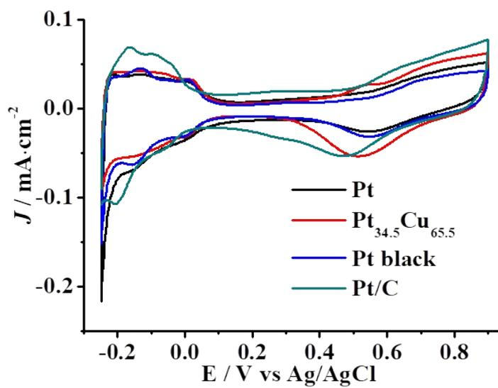
Fig. S3 The cyclic voltammetric curves (CVs) of the as-synthesized Pt Cubes,  $\text{Pt}_{34.5}\text{Cu}_{65.5}$  octahedrons, commercial Pt black and Pt/C in 0.1M  $\text{H}_2\text{SO}_4$  solution.
