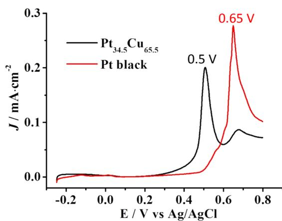
Fig. S4 LSV curves of electrochemical CO stripping on  $\text{Pt}_{34.5}\text{Cu}_{65.5}$  octahedrons and commercial Pt black in 0.1 M  $\text{H}_2\text{SO}_4$  saturated with CO at scan rate of  $50 \text{ mV s}^{-1}$ .
