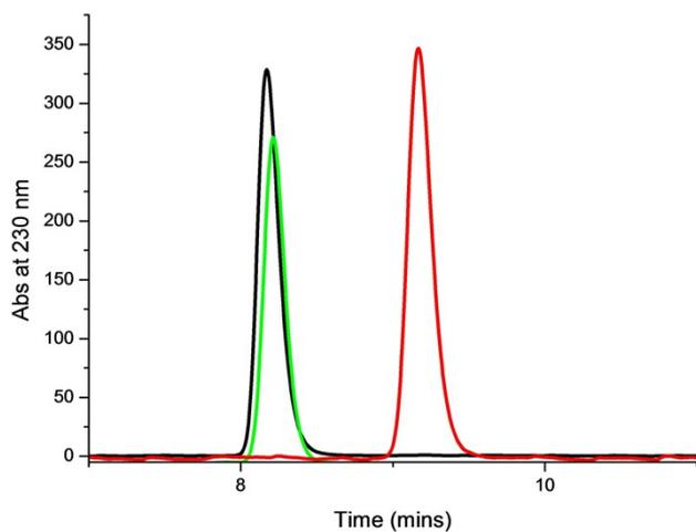
**Figure S9.** Chiral HPLC analysis of enantiomers of **1b** generated by the reaction of **5b** with XenA. Samples were run on an Agilent 1100 HPLC system with a Chiralpak AS-RH reverse phase column (150 x 4.6 mm ID) using a diode array detector (220 nm). Mobile phase was composed of acetonitrile/H<sub>2</sub>O 40:60 and with a flow rate of 0.8 mL/min run at 20 °C. Black, red and green traces show the (*R*)-**1b** and (*S*)-**1b** standards and XenA reaction products, respectively.
