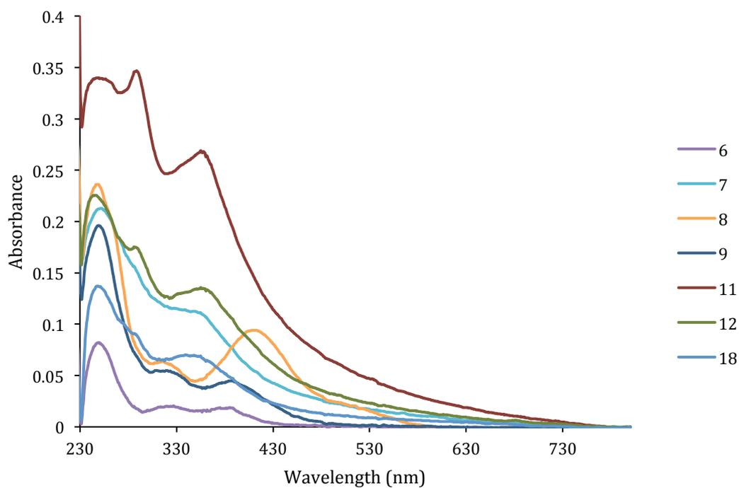
UV Vis absorption spectra of the selected molecules used in the CD experiments. Absorbance of 16  $\mu\text{M}$  compounds was measured in 10 mM Tris (pH 7.5) and 100 mM KCl. Concentration of DMSO was 1.25% (v/v) in all samples. Absorption spectra were recorded on a CARY 50 UV-vis spectrometer (Varian, USA). The optical path length was 1.0 cm.
