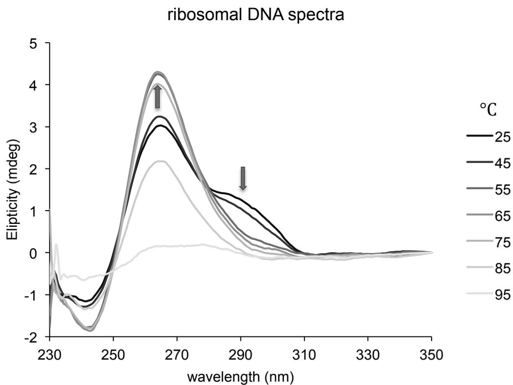
CD spectra of 5  $\mu$ M ribosomal DNA treated with 80  $\mu$ M compound **8** recorded at different temperatures (25, 45, 55, 65, 75, 85 and 95  $^{\circ}$ C). The peak at 295 nm (represents antiparallel folding) is quickly decreasing with increasing temperature while the peak at 264 nm (represents parallel folding) initially is increasing and has its maximum at 75  $^{\circ}$ C (arrows).
