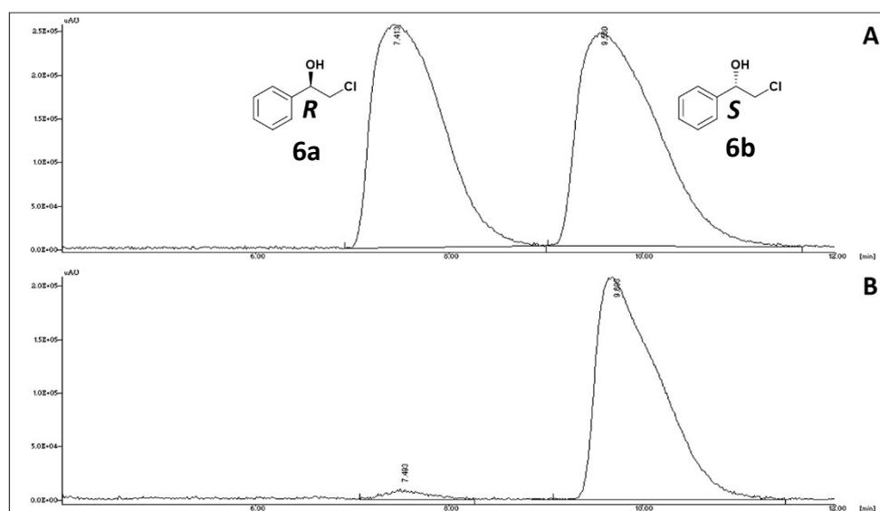
**Fig. 7** HPLC chromatogram for reduction of 2-chloroacetophenone (**2**) to (*S*)-2-chloro-1-phenylethan-1-ol (**6b**); A: racemic mixture of 2-chloro-1-phenylethan-1-ol (RT of *R*- 7.4 min and *S*- 9.6 min); B: reaction mixture (ee 99% of *S*).
