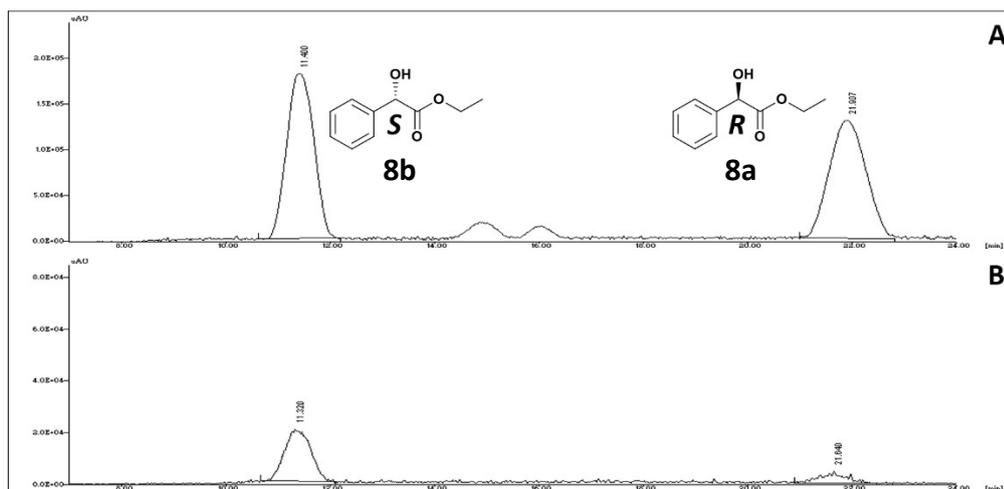
**Fig. 9** HPLC chromatogram for reduction of ethyl-2-oxo-2-phenylacetate (**4**) to (S)-ethyl-2-hydroxy-2-phenylacetate (**8b**); A: racemic mixture of ethyl-2-hydroxy-2-phenylacetate (RT of S- 11.4 min and R- 21.9 min); B: reaction mixture (ee 70% of S).
