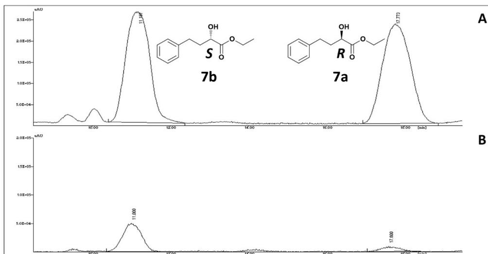
**Fig. 8** HPLC chromatogram for reduction of ethyl-2-oxo-4-phenylbutanoate (**3**) to (S)-ethyl-2-hydroxy-4-phenylbutanoate (**7b**); A: racemic mixture of ethyl-2-hydroxy-4-phenylbutanoate (RT of S- 11.2 min and R- 17.7 min); B: reaction mixture (ee 70% of S).
