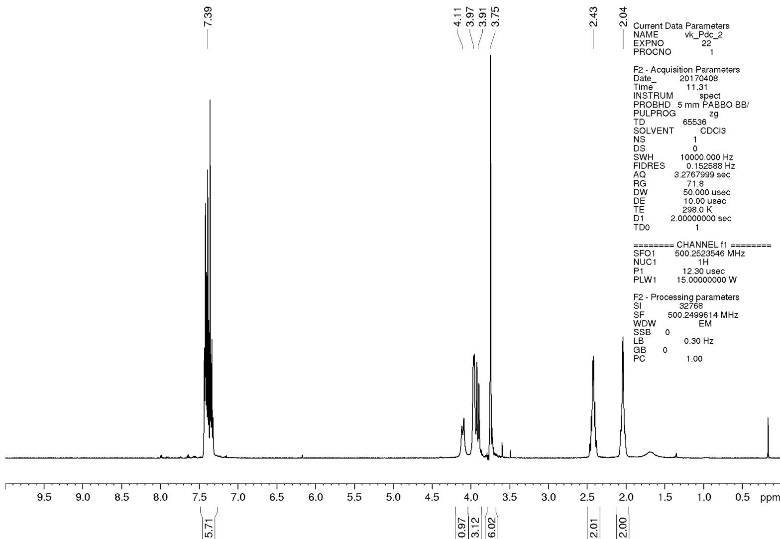
HCl·H-(MeO)mPdc-OMe in methanol-d<sub>4</sub>
