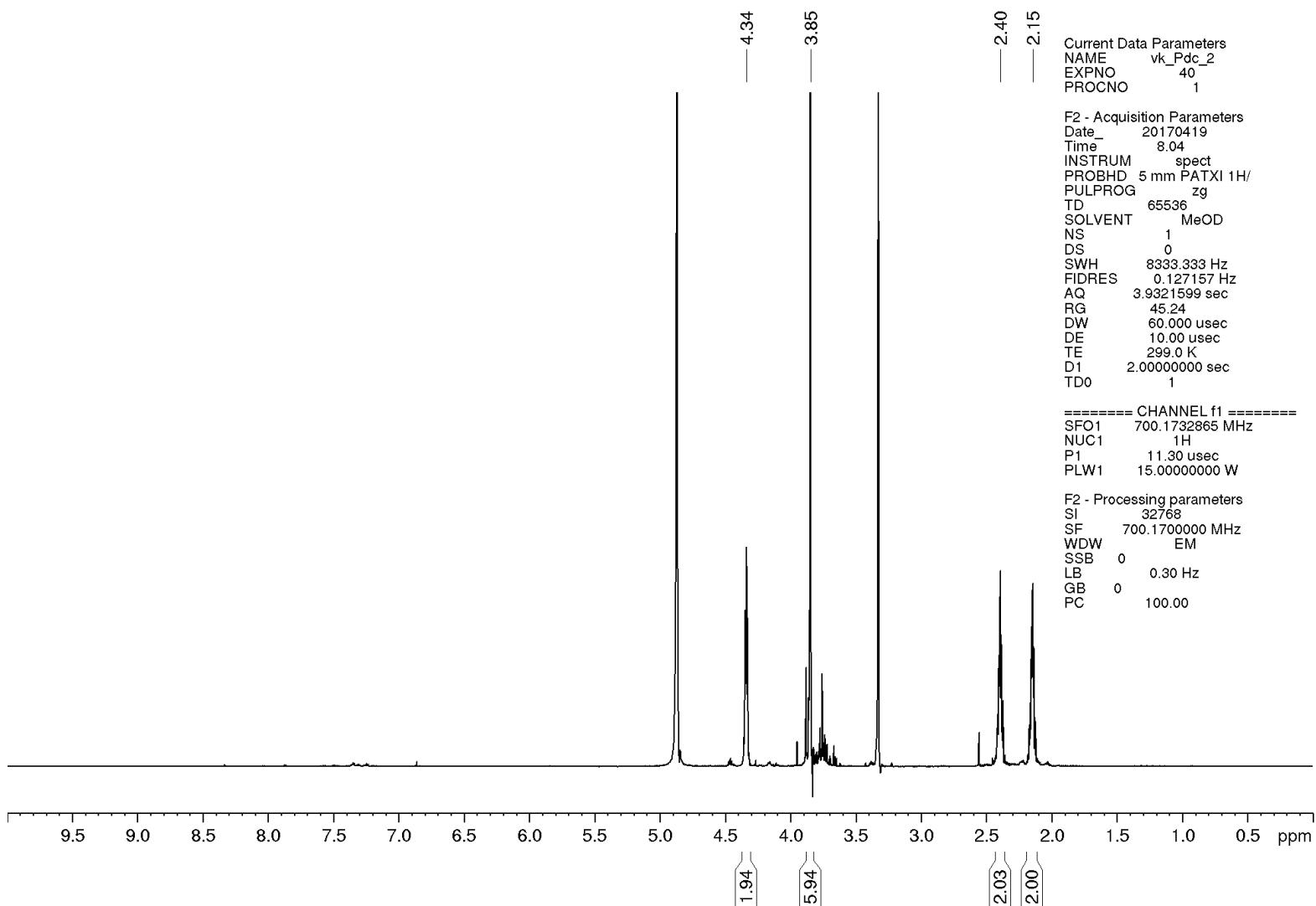
HCl·H-(MeO)rPdc-OMe in methanol-d<sub>4</sub>
