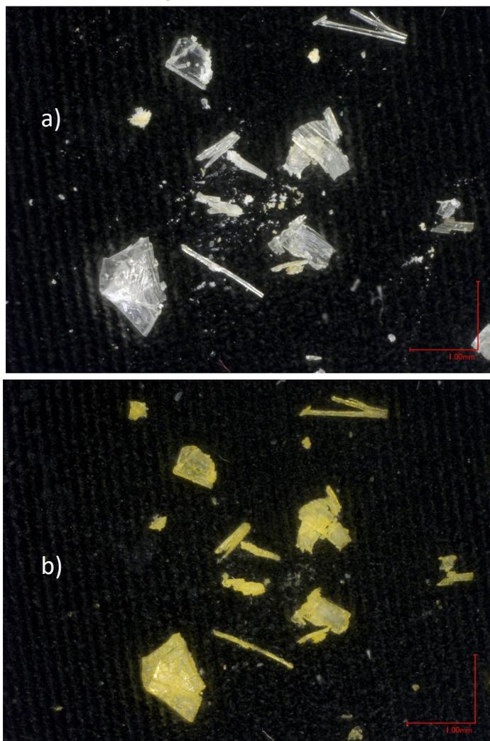
Figure S3. Crystals of azide 1 1a) before and b) after irradiation with mercury arc lamp through Pyrex filter.
