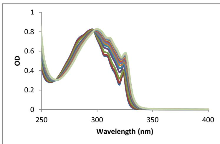
Graph S1. UV/vis spectra of titration of phosphine oxide with 1-naphthol in chloroform.
