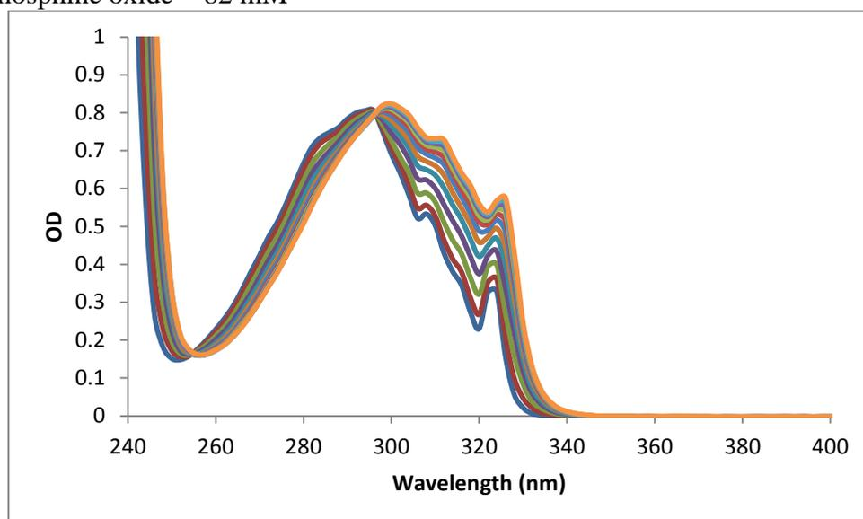
Graph S5. UV/vis spectra of titration of phosphine oxide with 1-naphthol in dichloromethane.
