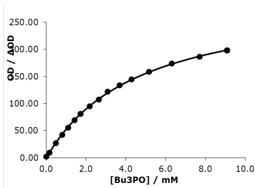
Graph S18. Binding isotherm for titration using 1:1 fitting program for titration of phosphine oxide against 1-naphthol in dichloromethane. [1-naphthol] = 0.055 mM and [phosphine oxide] = 126 mM.
