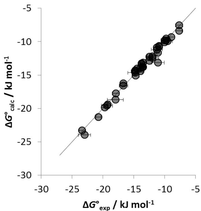
*Graph S21.* Graph showing comparison of experimental free energy on complexation ( $\Delta G^{\circ}_{exp}$ ) with the values calculated using eq 2 ( $\Delta G^{\circ}_{calc}$ ) for the H-bonded complexes (**1·X**, **2·X** and **3·X**) in the different solvents. The line represents  $\Delta G^{\circ}_{calc} = \Delta G^{\circ}_{exp}$ .
