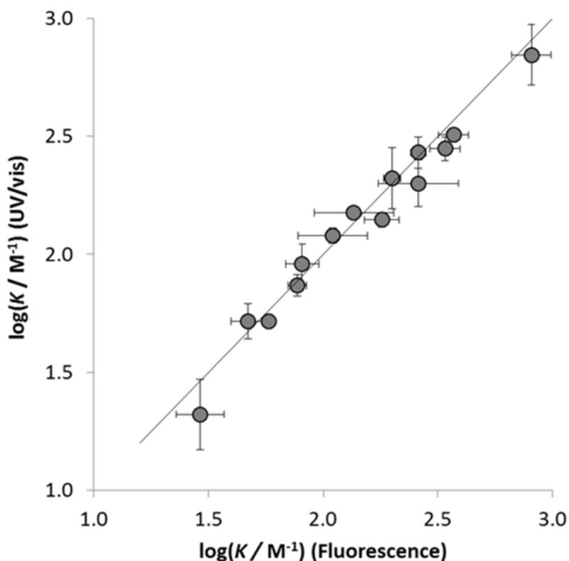
*Graph S22.* Comparison of the  $\log(K / M^{-1})$  obtained for the H-bonded complexes **1·X** when calculated from the experimental data obtained using fluorescence emission spectroscopy and UV/vis absorption spectroscopy. The line represents  $\log(K / M^{-1})$  (fluorescence emission spectroscopy) =  $\log(K / M^{-1})$  (UV/vis absorption spectroscopy).
