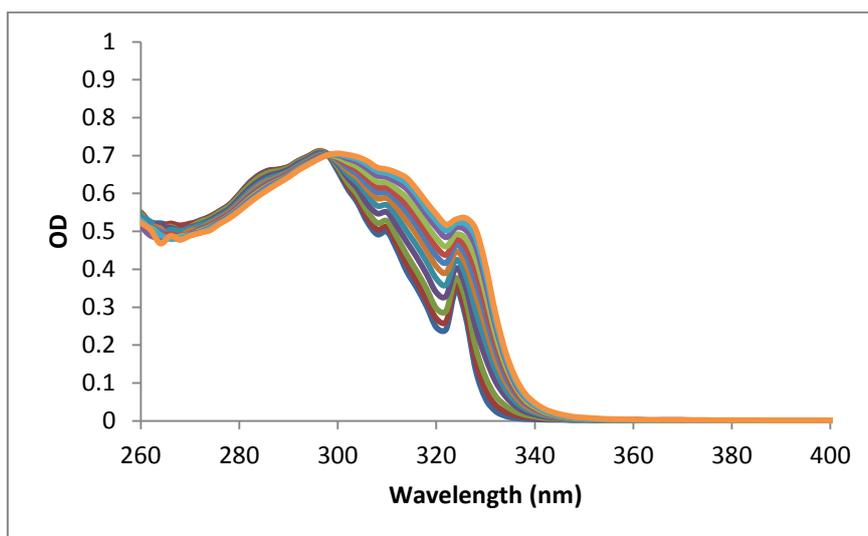
Graph S9. UV/vis spectra of titration of Bu<sub>3</sub>P(O) with 1-naphthol in CCl<sub>4</sub>.
