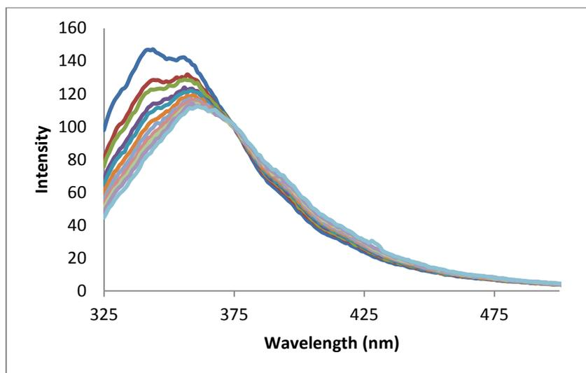
Graph S15. Fluorescence spectra of titration of TBACl with 1-naphthol in chloroform.
