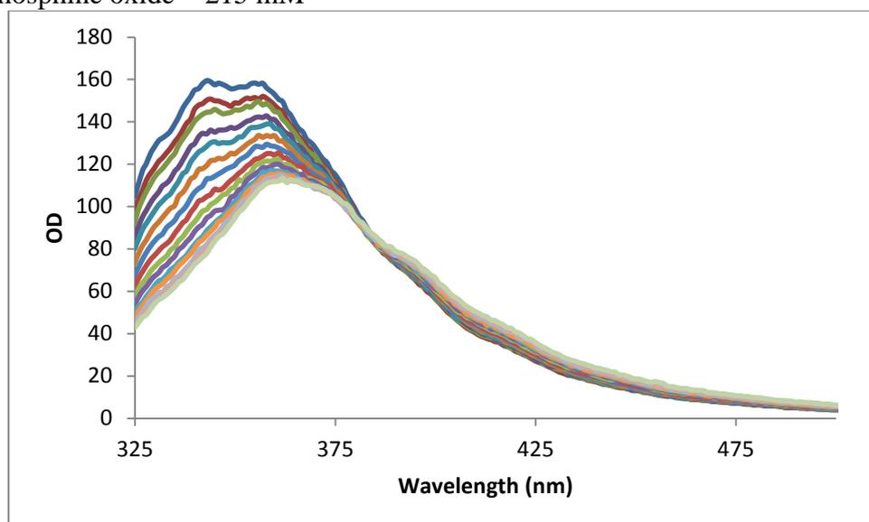
Graph S13. Fluorescence spectra of titration of phosphine oxide with 1-naphthol in chloroform.
