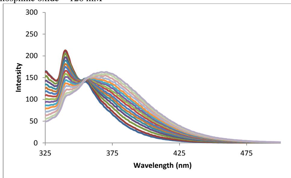
Graph S17. Fluorescence spectra of titration of phosphine oxide with 1-naphthol in dichloromethane.
