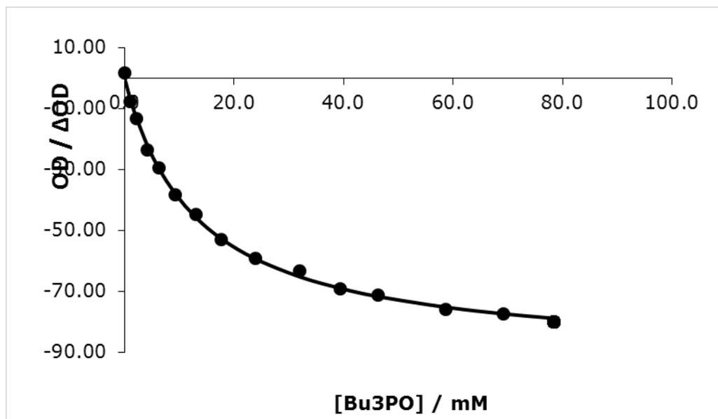
Graph S14. Binding isotherm for titration using 1:1 fitting program for titration of phosphine oxide against 1-naphthol in chloroform. [1-naphthol] = 0.041 mM and [phosphine oxide] = 215 mM.
