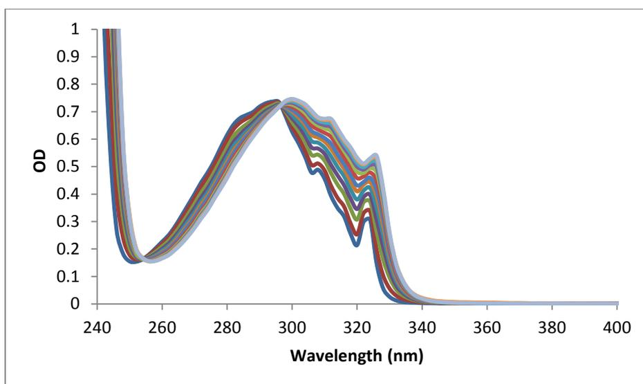
Graph S7. UV/vis spectra of titration of TBACl with 1-naphthol in dichloromethane.
