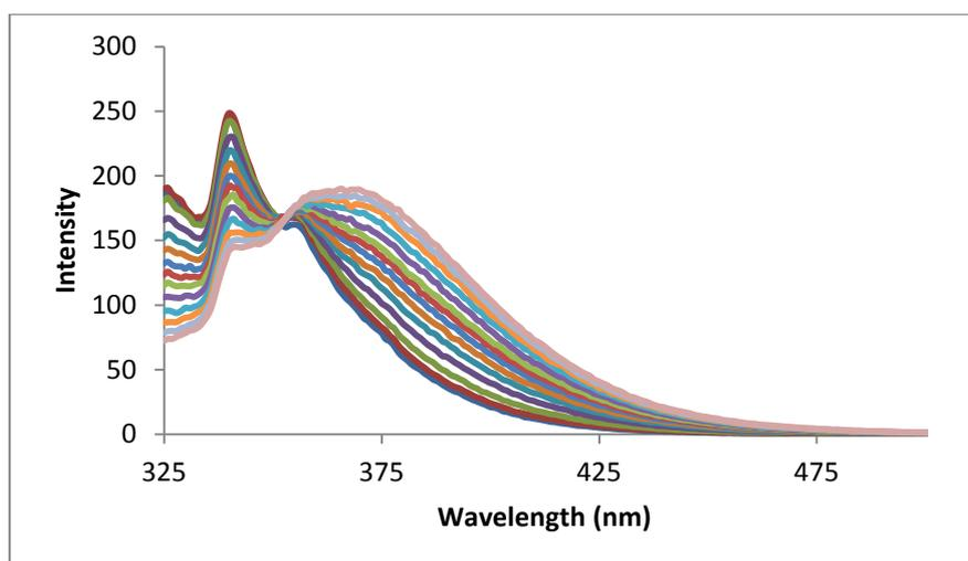
Graph S19. Fluorescence spectra of titration of TBACl with 1-naphthol in dichloromethane.
