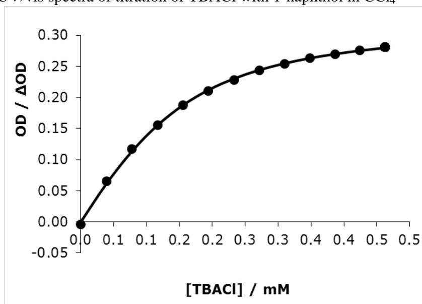
Graph S12. Binding isotherm for titration using 1:1 fitting program for titration of TBACl against 1-naphthol in CCl<sub>4</sub>. [1-naphthol] = 0.14 mM and [TBACl] = 39 mM,  $\Delta\lambda = 22$  nm,  $\Delta OD = 0.325$ .
