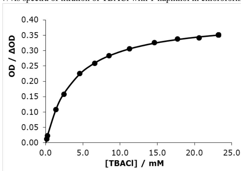
Graph S4. Binding isotherm for titration using 1:1 fitting program for titration of TBACl against 1-naphthol in chloroform. [1-naphthol] = 0.16 mM and [TBACl] = 92 mM,  $\Delta\lambda = 22$  nm,  $\Delta OD = 0.351$ .
