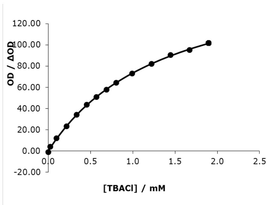
Graph S20. Binding isotherm for titration using 1:1 fitting program for titration of TBACl against 1-naphthol in dichloromethane. [1-naphthol] = 0.062 mM and [TBACl] = 48 mM.
