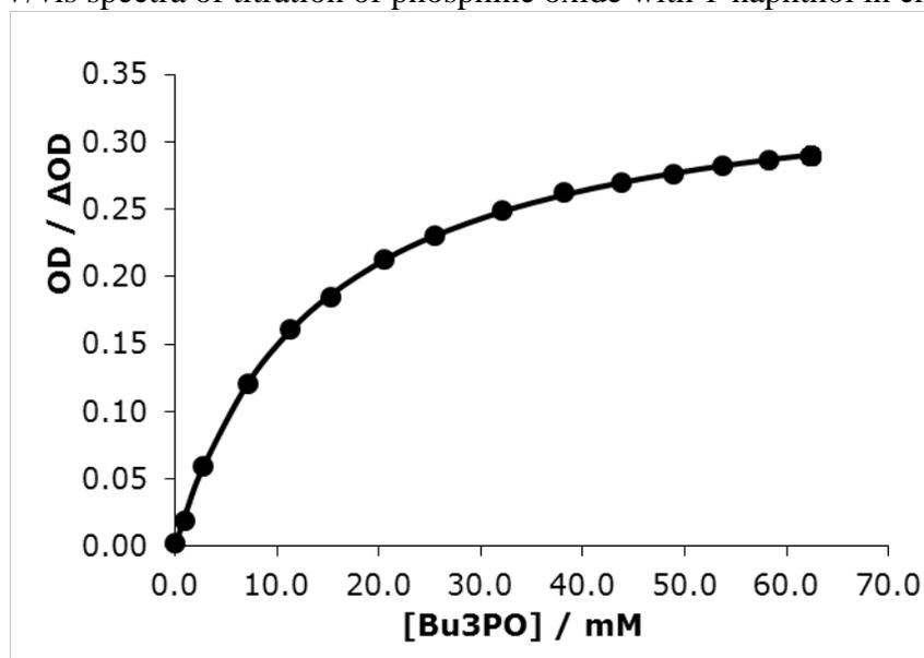
Graph S2. Binding isotherm for titration using 1:1 fitting program for titration of phosphine oxide against 1-naphthol in chloroform. [1-naphthol] = 0.16 mM and [phosphine oxide] = 184 mM,  $\Delta\lambda = 14$  nm,  $\Delta$ OD = 0.354.
