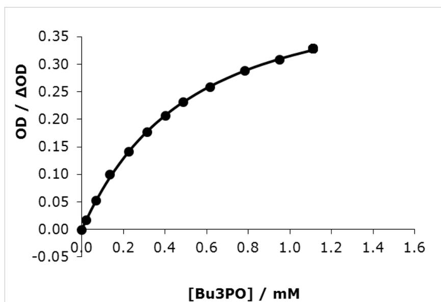
Graph S10. Binding isotherm for titration using 1:1 fitting program interaction for titration of Bu<sub>3</sub>P(O) against 1-naphthol in CCl<sub>4</sub>. [1-naphthol] = 0.14 mM and [Bu<sub>3</sub>P(O)] = 18 mM,  $\Delta\lambda = 34$  nm,  $\Delta OD = 0.458$ .
