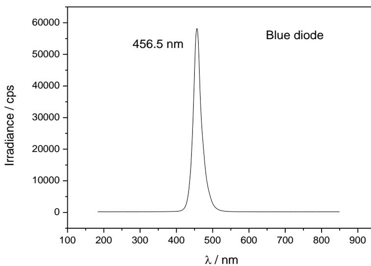
**Figure S7.** Emission spectrum of the blue light emitting diodes (LEDs) used in the reactions.
