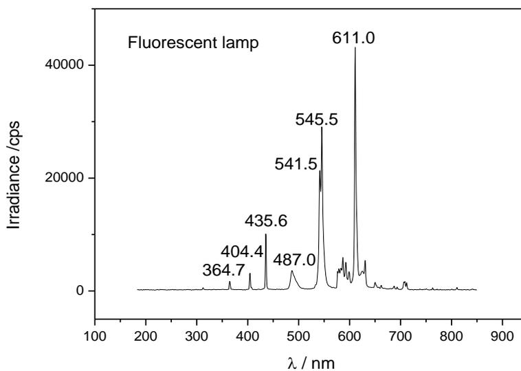
**Figure S8.** Emission spectrum of the compact fluorescence lamp (CFL).
