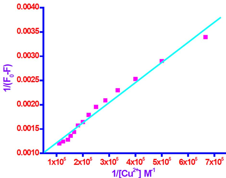
**Figure S29.** Benesi-Hildebrand plot  $1 / (F_0 - F)$  vs.  $1/[Cu^{2+}]$  for complexation between **5d** and  $Cu^{2+}$  derived from emission titration curve.
