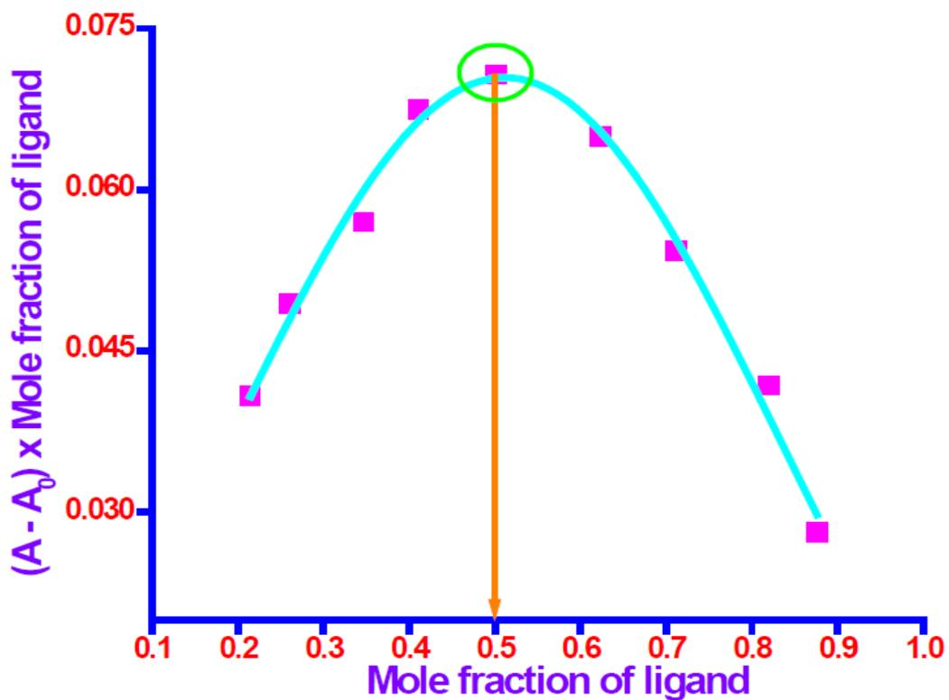
Figure S20. Job's plot for determination of stoichiometry of  $\text{Cu}^{2+} : 5\text{c}$  complex in solution.
