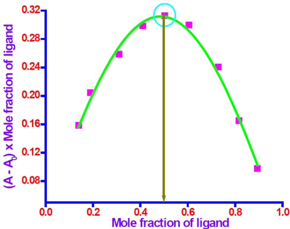
Figure S19. Job's plot for determination of stoichiometry of  $\text{Cu}^{2+}$ : **5b** complex in solution.
