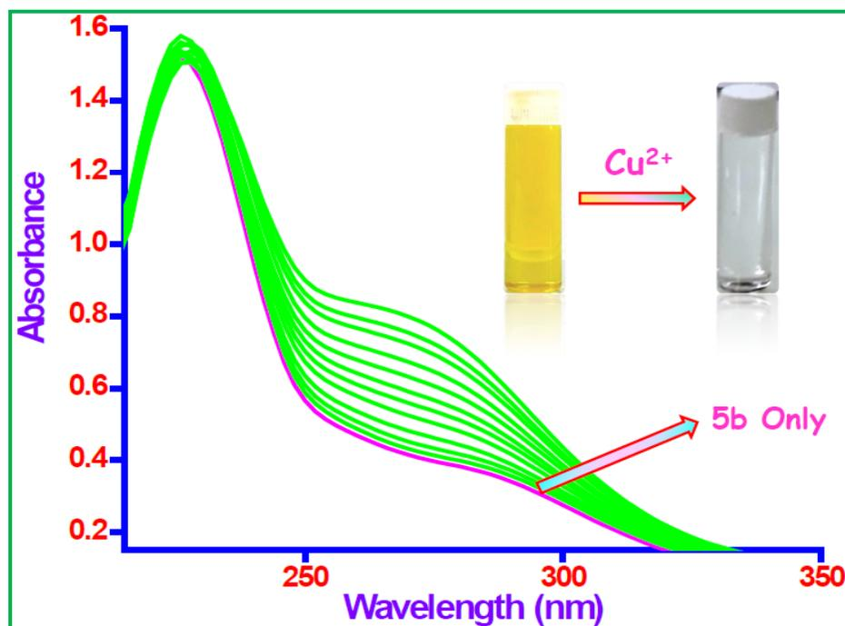
**Figure S3.** UV-vis spectra of **5b** ( $5 \times 10^{-6}$  M) in DMSO/H<sub>2</sub>O (1:9, v/v) HEPES buffer (pH = 7.4) solution in the presence of various concentrations of Cu<sup>2+</sup> (0, 0.5, 1, 2, 3, 4, 5, 6, 7, 8, 9 and 10) × 10<sup>-6</sup> M. **Inset:** visual color change (yellow to colorless) observed with addition of Cu<sup>2+</sup> ion to **5b** solution.
