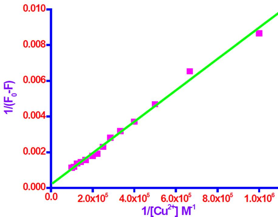
**Figure S30.** Benesi-Hildebrand plot  $1 / (F_0 - F)$  vs.  $1/[Cu^{2+}]$  for complexation between **5f** and  $Cu^{2+}$  derived from emission titration curve.
