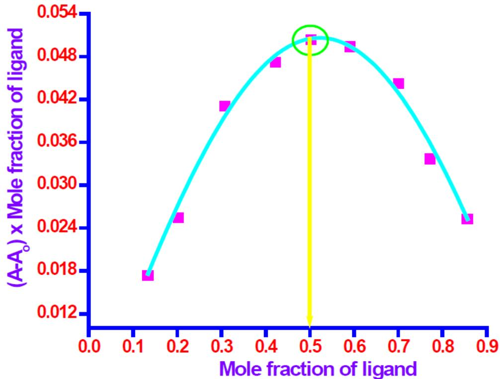
Figure S21. Job's plot for determination of stoichiometry of  $\text{Cu}^{2+} : 5\text{d}$  complex in solution.
