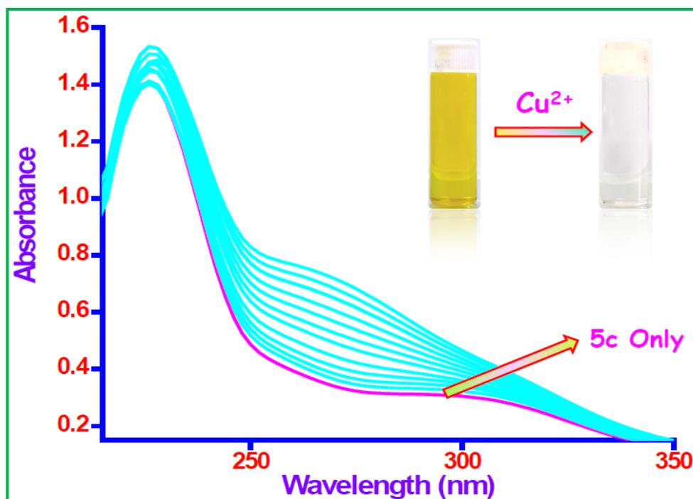
**Figure S4.** UV-vis spectra of **5c** ( $5 \times 10^{-6}$  M) in DMSO/H<sub>2</sub>O (1:9, v/v) HEPES buffer (pH = 7.4) solution in the presence of various concentrations of Cu<sup>2+</sup> (0, 0.5, 1, 2, 3, 4, 5, 6, 7, 8, 9 and 10)  $\times 10^{-6}$  M. **Inset:** visual color change (yellow to colorless) observed with addition of Cu<sup>2+</sup> ion to **5c** solution.
