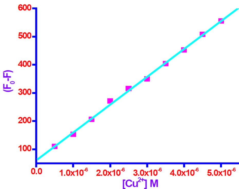
**Figure S37.** The limit of detection (LOD) of **5j** for Cu<sup>2+</sup> as a function of [Cu<sup>2+</sup>].
