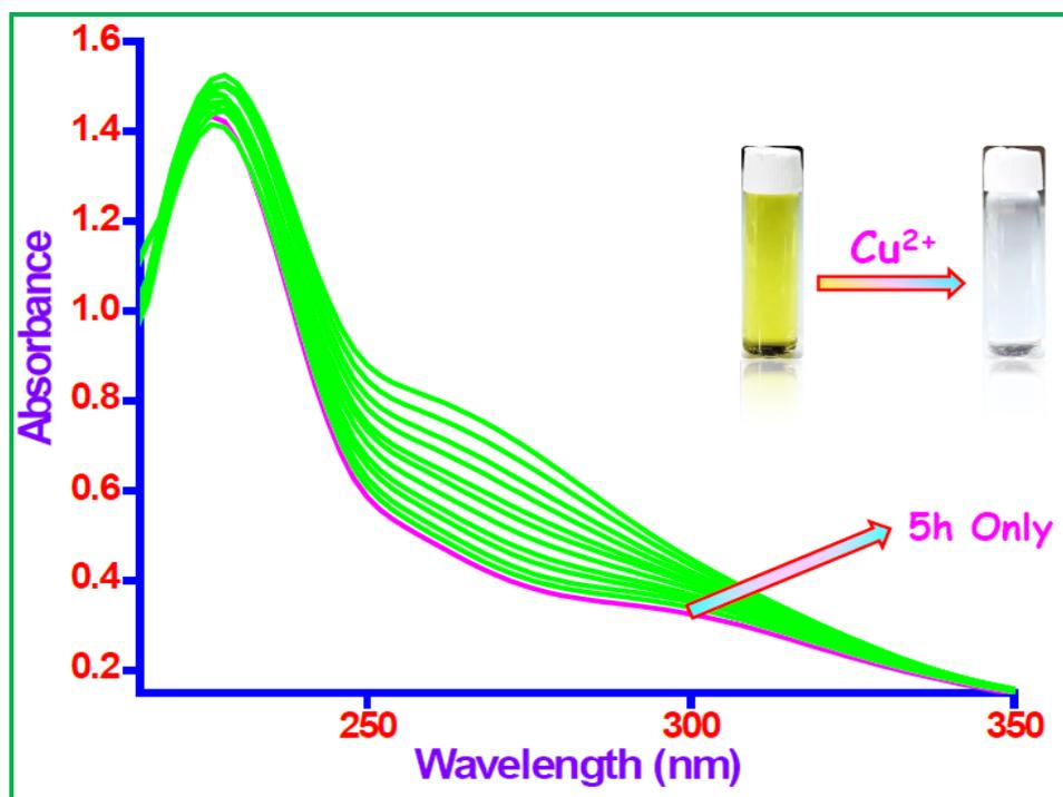
**Figure S8.** UV-vis spectra of **5h** ( $5 \times 10^{-6}$  M) in DMSO/H<sub>2</sub>O (1:9, v/v) HEPES buffer (pH = 7.4) solution in the presence of various concentrations of Cu<sup>2+</sup> (0, 0.5, 1, 2, 3, 4, 5, 6, 7, 8, 9 and 10) × 10<sup>-6</sup> M. **Inset:** visual color change (yellow to colorless) observed with addition of Cu<sup>2+</sup> ion to **5h** solution.
