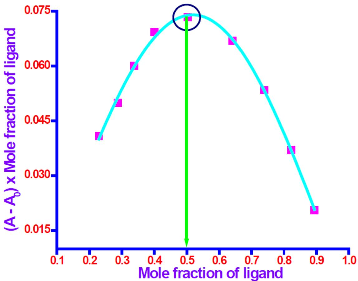
Figure S28. Job's plot for determination of stoichiometry of  $\text{Cu}^{2+} : 5\text{I}$  complex in solution.
