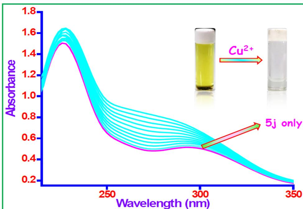
**Figure S10.** UV-vis spectra of **5j** ( $5 \times 10^{-6}$  M) in DMSO/H<sub>2</sub>O (1:9, v/v) HEPES buffer (pH = 7.4) solution in the presence of various concentrations of Cu<sup>2+</sup> (0, 1, 2, 3, 4, 5, 6, 7, 8, 9 and 10)  $\times 10^{-6}$  M. **Inset:** visual color change (yellow to colorless) observed with addition of Cu<sup>2+</sup> ion to **5j** solution.
