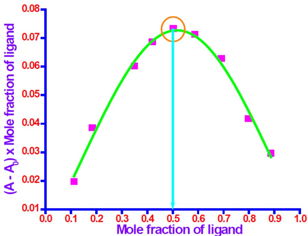
Figure S24. Job's plot for determination of stoichiometry of  $\text{Cu}^{2+} : \mathbf{5h}$  complex in solution.
