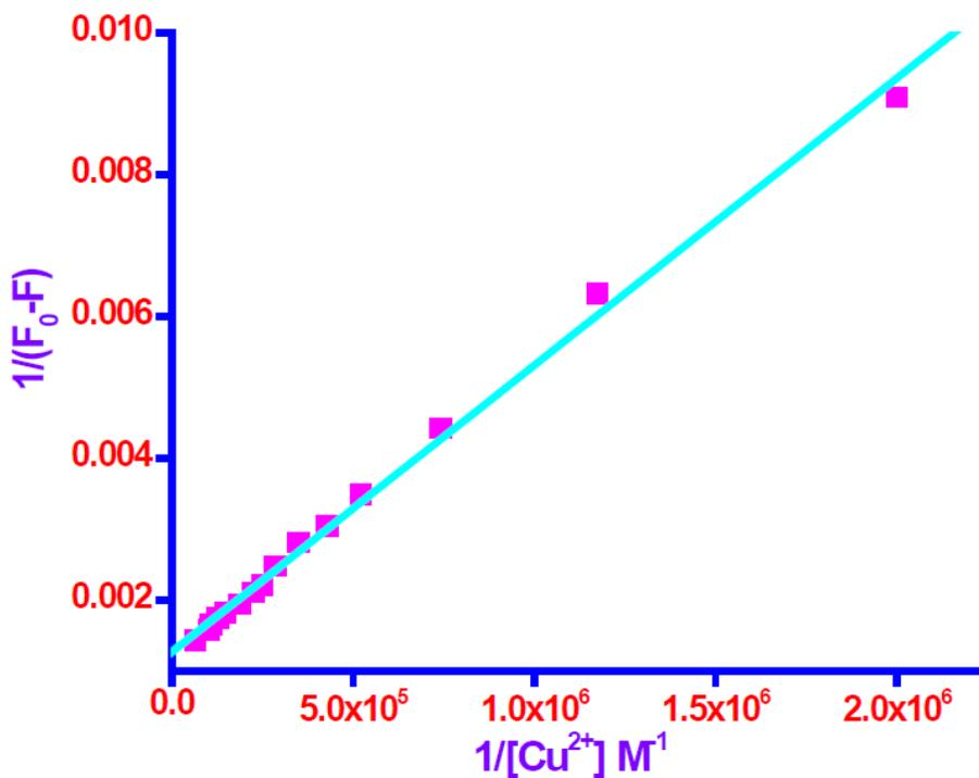
**Figure S32.** Benesi-Hildebrand plot  $I / (F_0 - F)$  vs.  $1/[Cu^{2+}]$  for complexation between **5j** and  $Cu^{2+}$  derived from emission titration curve.
