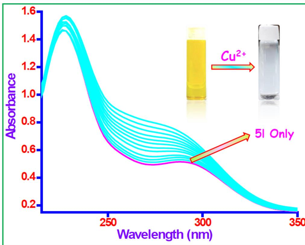
**Figure S12.** UV-vis spectra of **5I** ( $5 \times 10^{-6}$  M) in DMSO/H<sub>2</sub>O (1:9, v/v) HEPES buffer (pH = 7.4) solution in the presence of various concentrations of Cu<sup>2+</sup> (0, 0.5, 1, 2, 3, 4, 5, 6, 7, 8, 9 and 10)  $\times 10^{-6}$  M. **Inset:** visual color change (yellow to colorless) observed with addition of Cu<sup>2+</sup> ion to **5I** solution.
