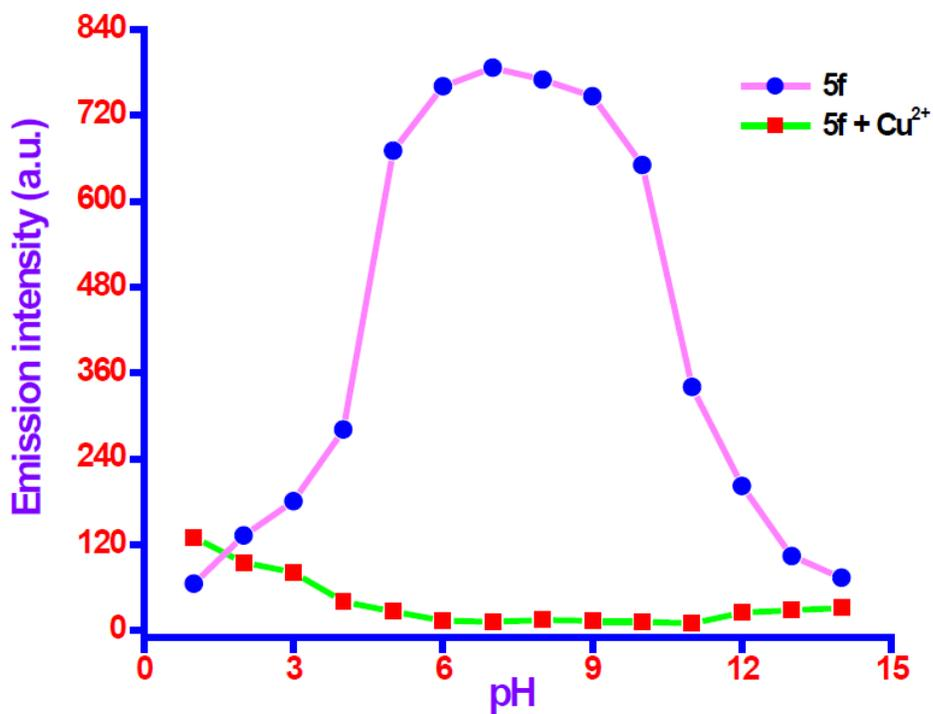
**Figure S45.** Emission intensity of **5f** ( $5 \times 10^{-6}$  M) in absence and in presence of  $\text{Cu}^{2+}$  as a function of pH values in aqueous DMSO solution at 491.7 nm.
