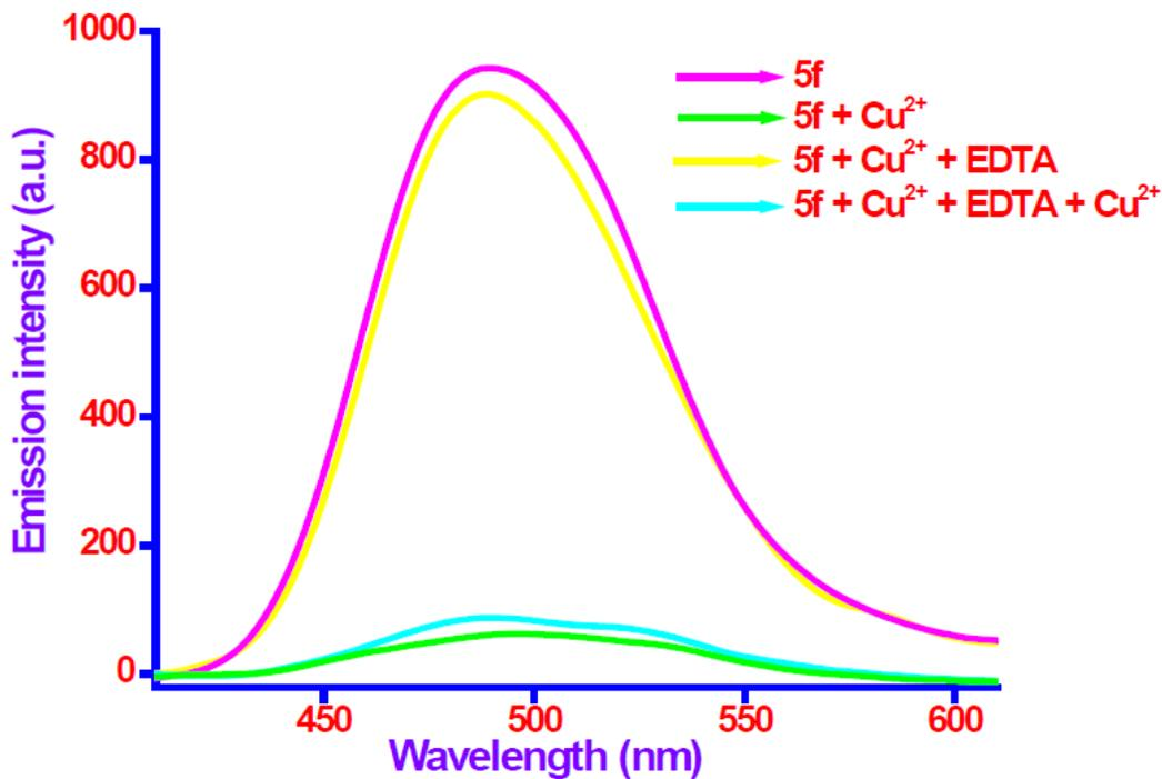
**Figure S40.** Fluorescence emission spectra of chemosensor (**5f**) in the presence of Cu<sup>2+</sup> ion followed by addition of EDTA.
