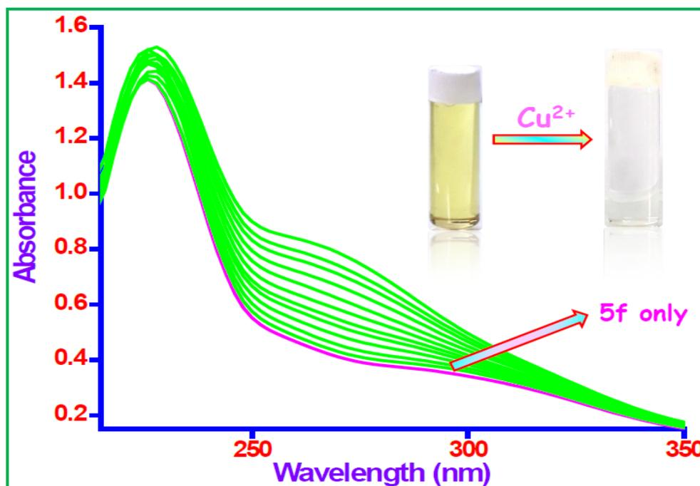
**Figure S7.** UV-vis spectra of **5f** ( $5 \times 10^{-6}$  M) in DMSO/H<sub>2</sub>O (1:9, v/v) HEPES buffer (pH = 7.4) solution in the presence of various concentrations of Cu<sup>2+</sup> (0, 0.5, 1, 2, 3, 4, 5, 6, 7, 8, 9 and 10) × 10<sup>-6</sup> M. **Inset:** visual color change (yellow to colorless) observed with addition of Cu<sup>2+</sup> ion to **5f** solution.
