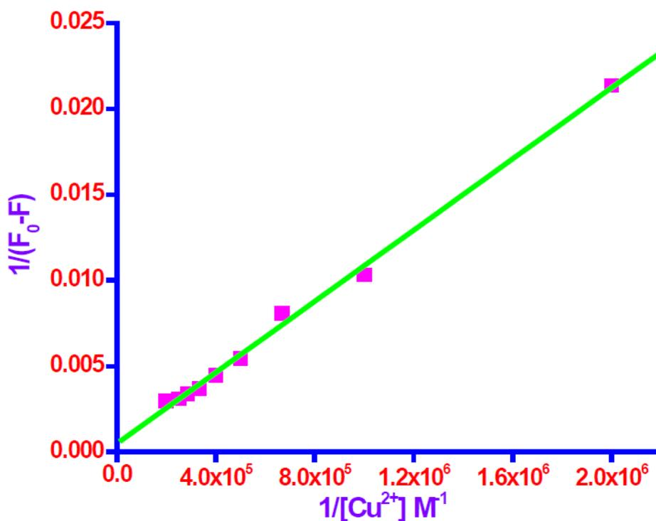
**Figure S31.** Benesi-Hildebrand plot  $I / (F_0 - F)$  vs.  $1/[Cu^{2+}]$  for complexation between **5h** and  $Cu^{2+}$  derived from emission titration curve.
