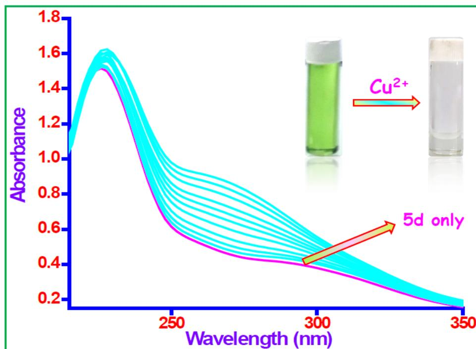
**Figure S5.** UV-vis spectra of **5d** ( $5 \times 10^{-6}$  M) in DMSO/H<sub>2</sub>O (1:9, v/v) HEPES buffer (pH = 7.4) solution in the presence of various concentrations of Cu<sup>2+</sup> (0, 1, 2, 3, 4, 5, 6, 7, 8, 9 and 10)  $\times 10^{-6}$  M. **Inset:** visual color change (green to colorless) observed with addition of Cu<sup>2+</sup> ion to **5d** solution.
