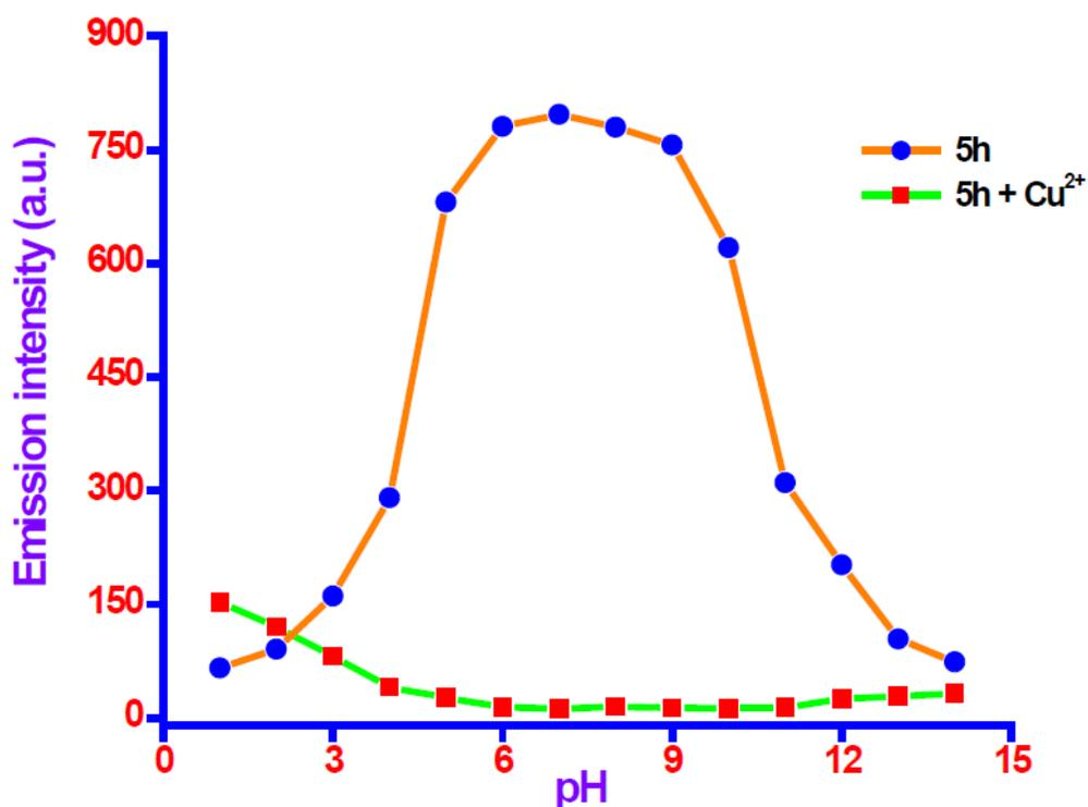
**Figure S46.** Emission intensity of **5h** ( $5 \times 10^{-6}$  M) in absence and in presence of  $\text{Cu}^{2+}$  as a function of pH values in aqueous DMSO solution at 498.7 nm.
