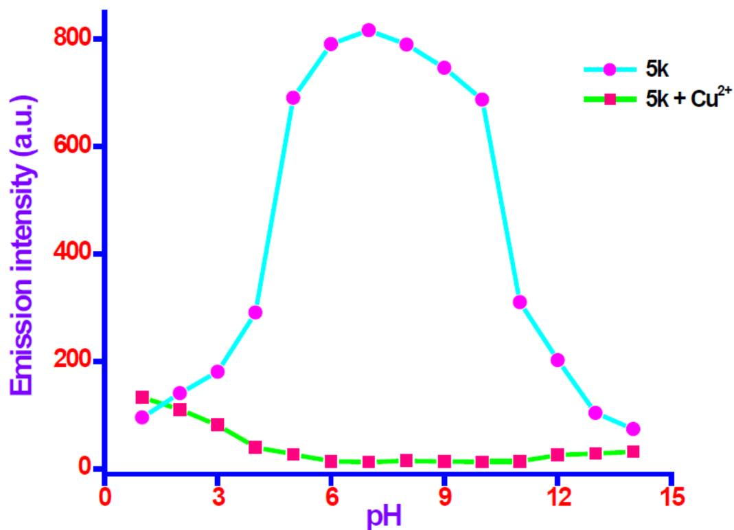
**Figure S48.** Emission intensity of **5k** ( $5 \times 10^{-6}$  M) in absence and in presence of  $\text{Cu}^{2+}$  as a function of pH values in aqueous DMSO solution at 503.5 nm.
