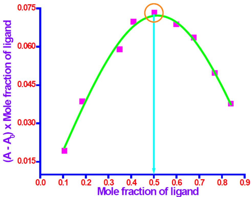
Figure S22. Job's plot for determination of stoichiometry of  $\text{Cu}^{2+} : 5\text{e}$  complex in solution.
