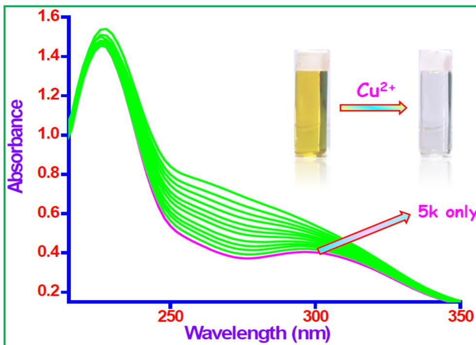
**Figure S11.** UV-vis spectra of **5k** ( $5 \times 10^{-6}$  M) in DMSO/H<sub>2</sub>O (1:9, v/v) HEPES buffer (pH = 7.4) solution in the presence of various concentrations of Cu<sup>2+</sup> (0, 0.5, 1, 2, 3, 4, 5, 6, 7, 8, 9 and 10)  $\times 10^{-6}$  M. **Inset:** visual color change (yellow to colorless) observed with addition of Cu<sup>2+</sup> ion to **5k** solution.
