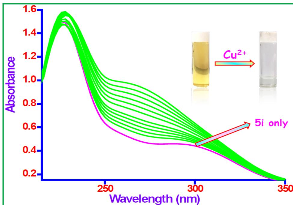
**Figure S9.** UV-vis spectra of **5i** ( $5 \times 10^{-6}$  M) in DMSO/H<sub>2</sub>O (1:9, v/v) HEPES buffer (pH = 7.4) solution in the presence of various concentrations of Cu<sup>2+</sup> (0, 0.5, 1, 2, 3, 4, 5, 6, 7, 8, 9 and 10) × 10<sup>-6</sup> M. **Inset:** visual color change (yellow to colorless) observed with addition of Cu<sup>2+</sup> ion to **5i** solution.
