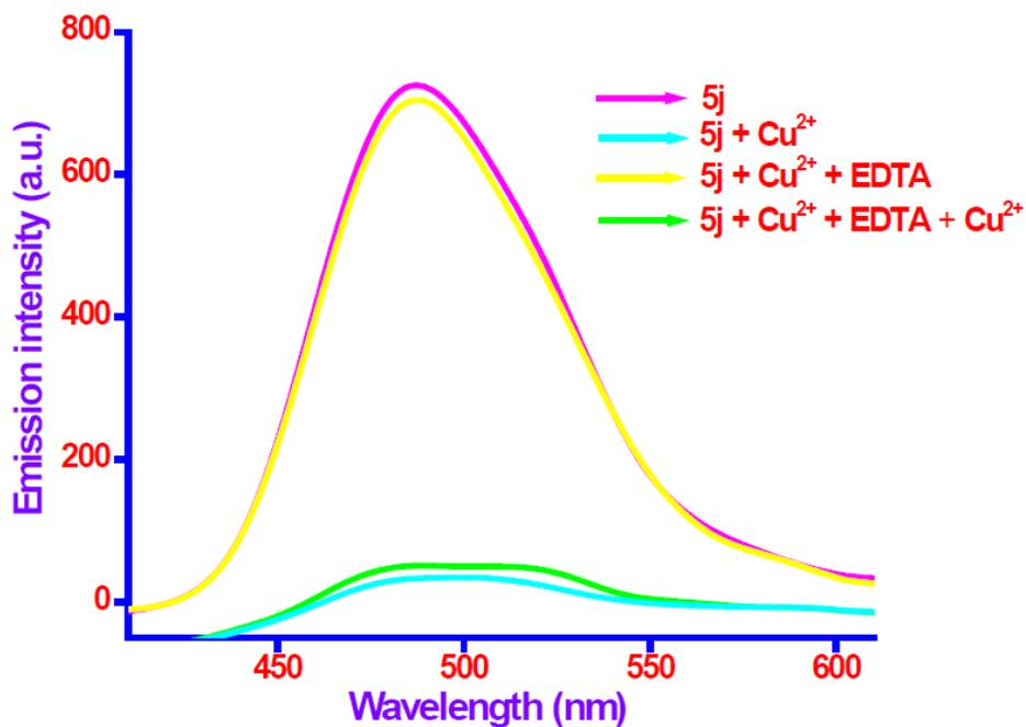
**Figure S42.** Fluorescence emission spectra of chemosensor (**5j**) in the presence of Cu<sup>2+</sup> ion followed by addition of EDTA.
