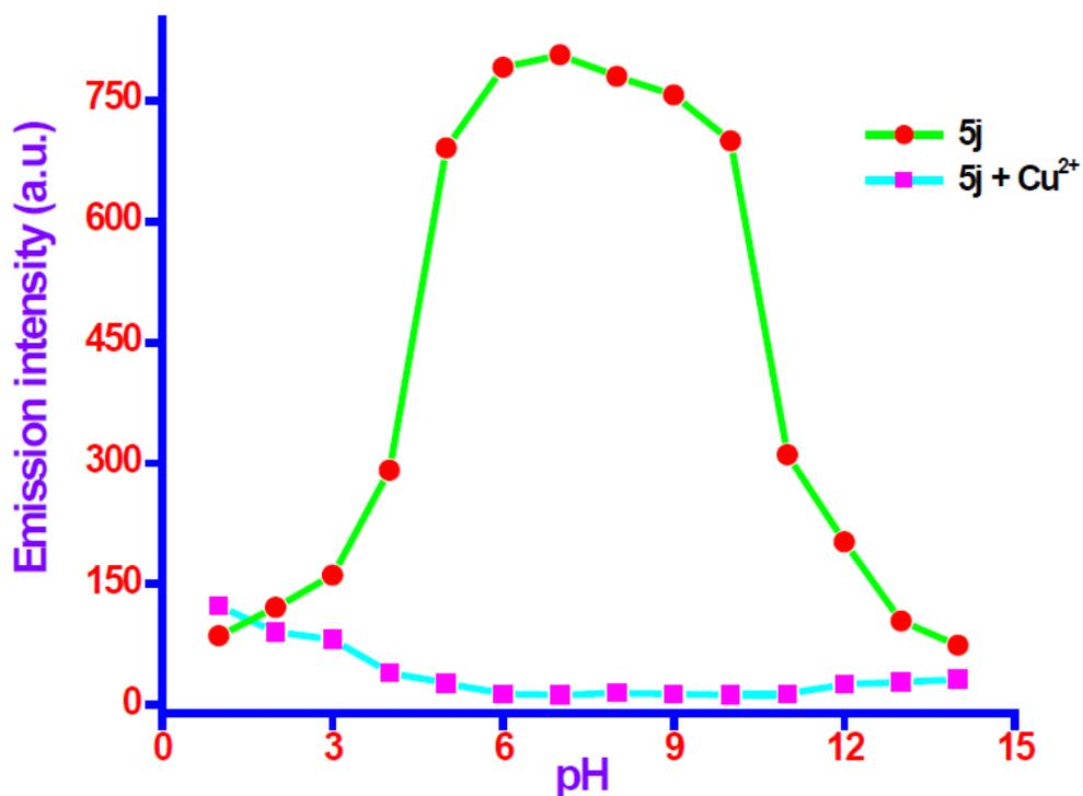
**Figure S47.** Emission intensity of **5j** ( $5 \times 10^{-6}$  M) in absence and in presence of  $\text{Cu}^{2+}$  as a function of pH values in aqueous DMSO solution at 497.8 nm.
