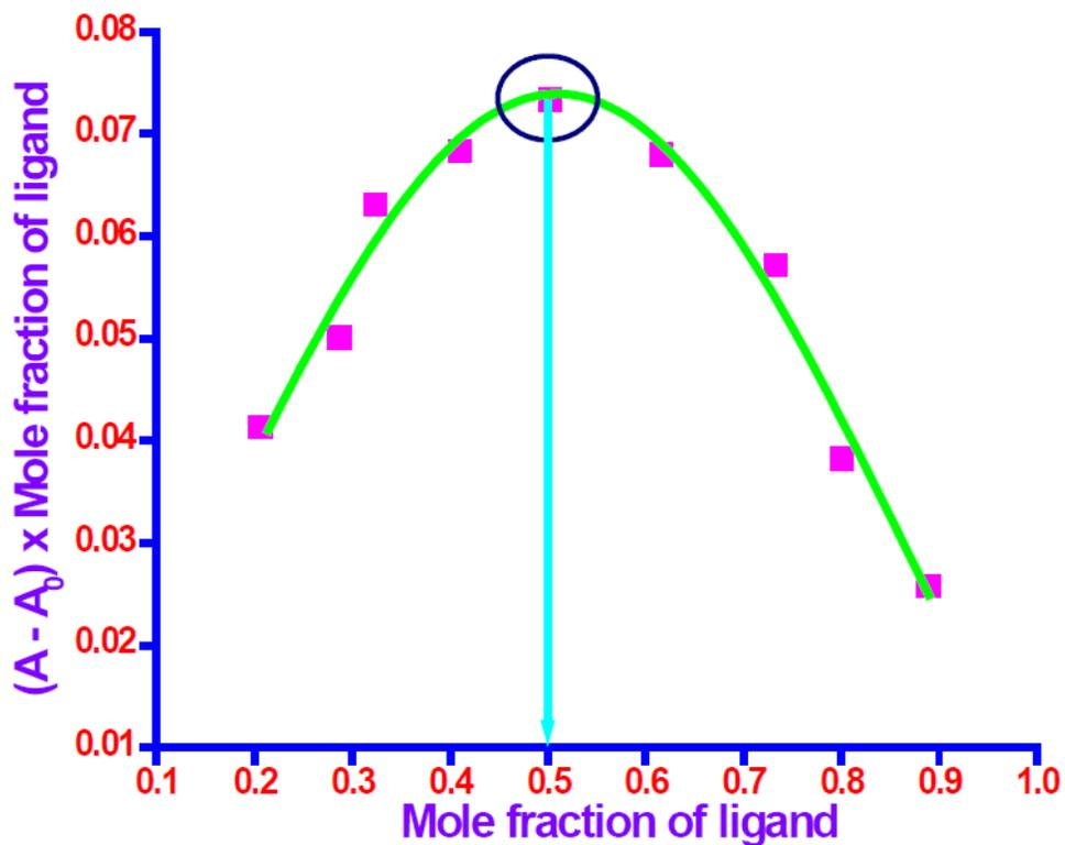
Figure S23. Job's plot for determination of stoichiometry of  $\text{Cu}^{2+} : 5\text{f}$  complex in solution.
