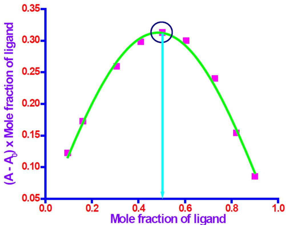
**Figure S27.** Job's plot for determination of stoichiometry of  $\text{Cu}^{2+} : \mathbf{5k}$  complex in solution.
