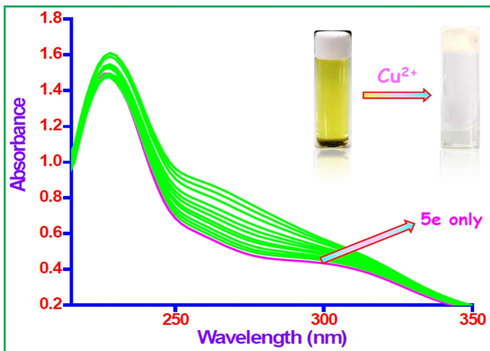
**Figure S6.** UV-vis spectra of **5e** ( $5 \times 10^{-6}$  M) in DMSO/H<sub>2</sub>O (1:9, v/v) HEPES buffer (pH = 7.4) solution in the presence of various concentrations of Cu<sup>2+</sup> (0, 0.5, 1, 2, 3, 4, 5, 6, 7, 8, 9 and 10) × 10<sup>-6</sup> M. **Inset:** visual color change (yellow to colorless) observed with addition of Cu<sup>2+</sup> ion to **5e** solution.
