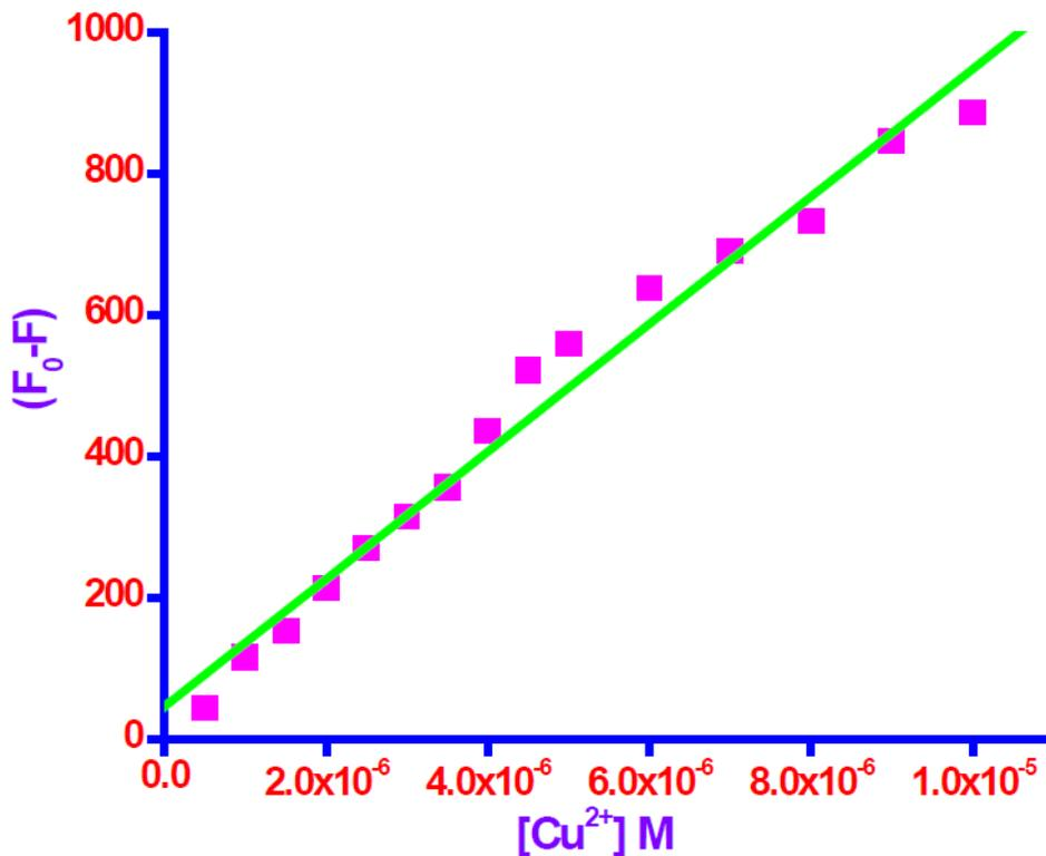
Figure S35. The limit of detection (LOD) of **5f** for Cu<sup>2+</sup> as a function of [Cu<sup>2+</sup>].
