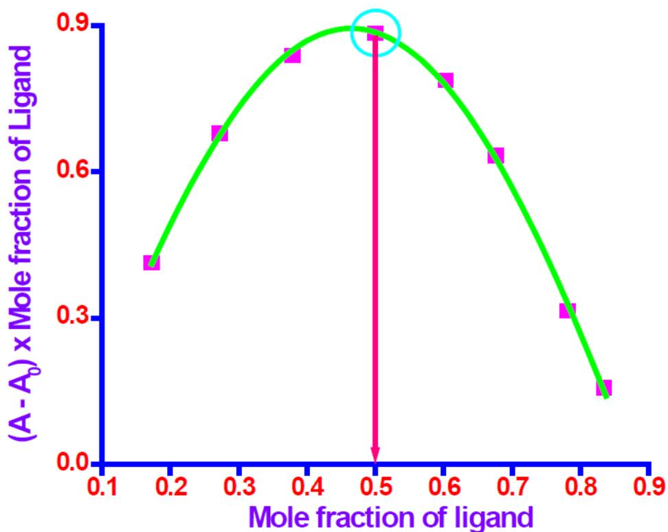
Figure S25. Job's plot for determination of stoichiometry of  $\text{Cu}^{2+} : \mathbf{5i}$  complex in solution.
