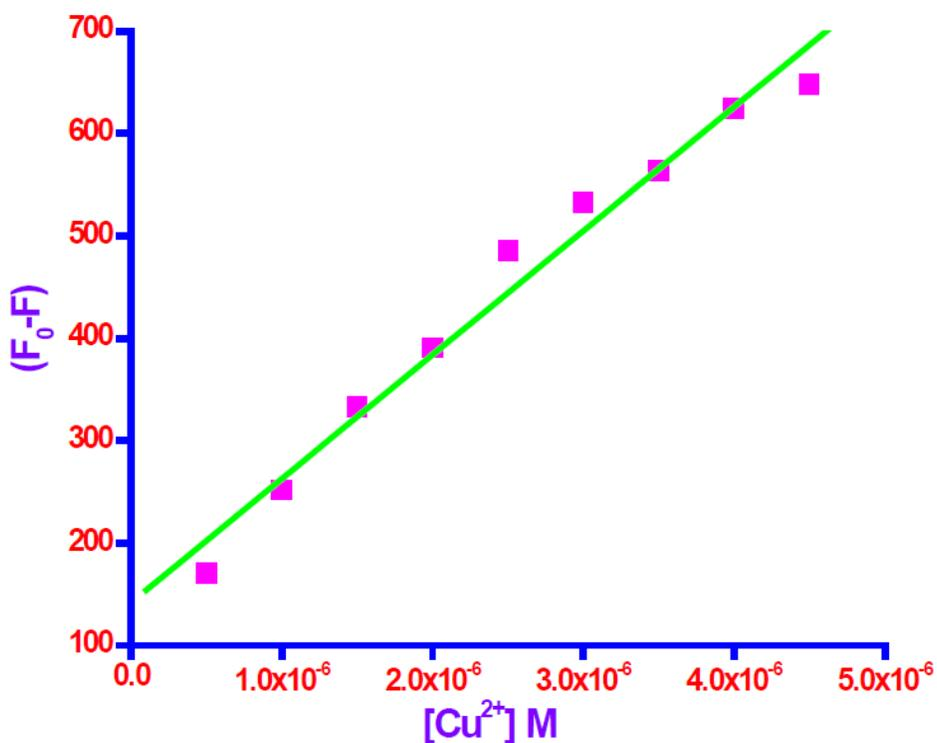
**Figure S38.** The limit of detection (LOD) of **5k** for Cu<sup>2+</sup> as a function of [Cu<sup>2+</sup>].
