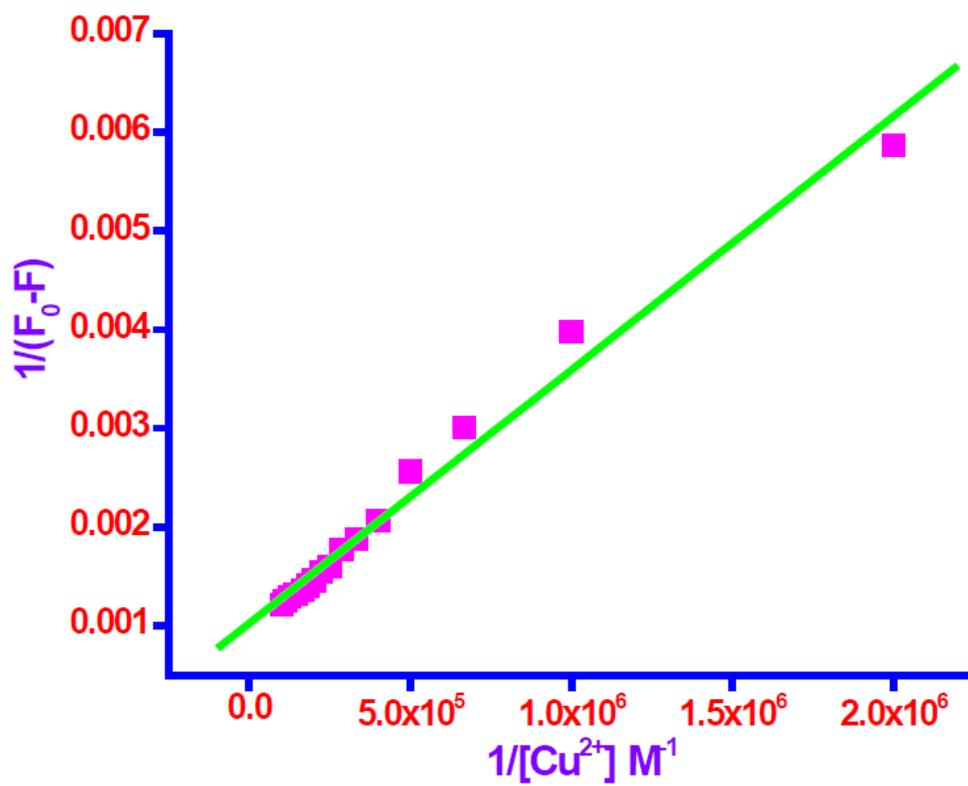
**Figure S33.** Benesi-Hildebrand plot  $1 / (F_0 - F)$  vs.  $1/[Cu^{2+}]$  for complexation between **5k** and  $Cu^{2+}$  derived from emission titration curve.
