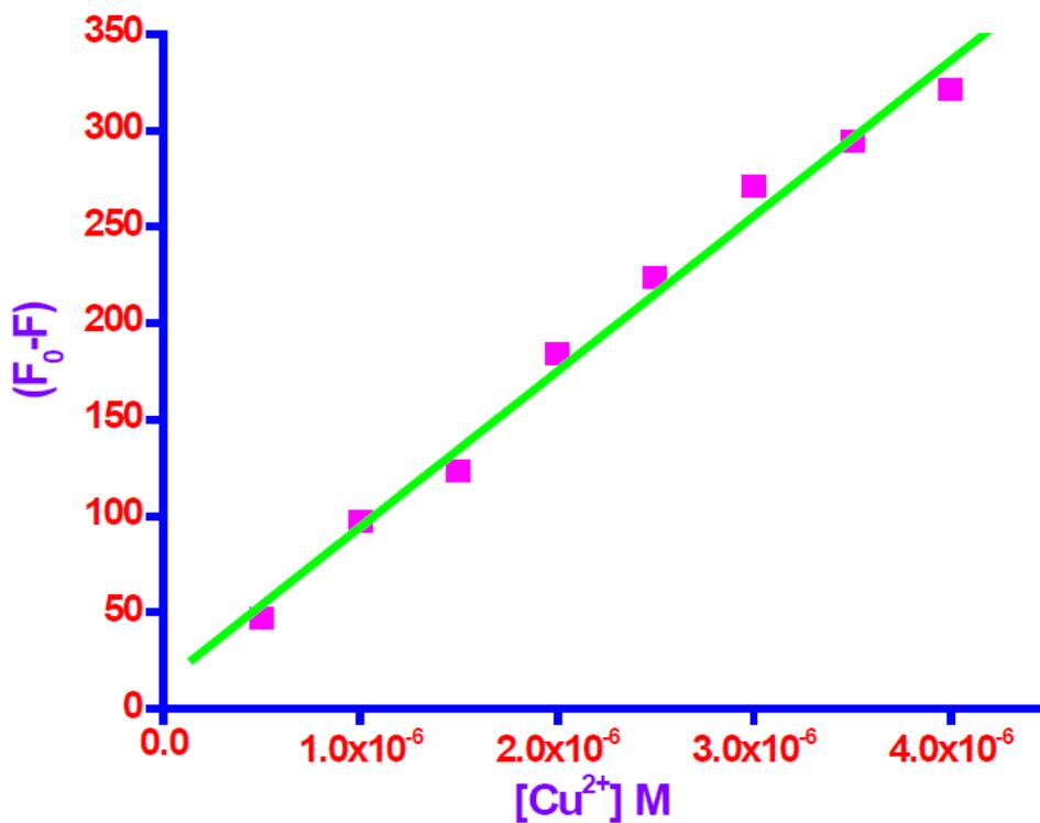
Figure S36. The limit of detection (LOD) of **5h** for Cu<sup>2+</sup> as a function of [Cu<sup>2+</sup>].
