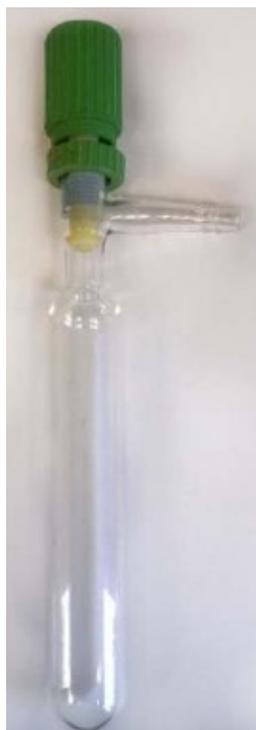
Fig. 1. High pressure Schlenk tube used for reductive amination reaction.
