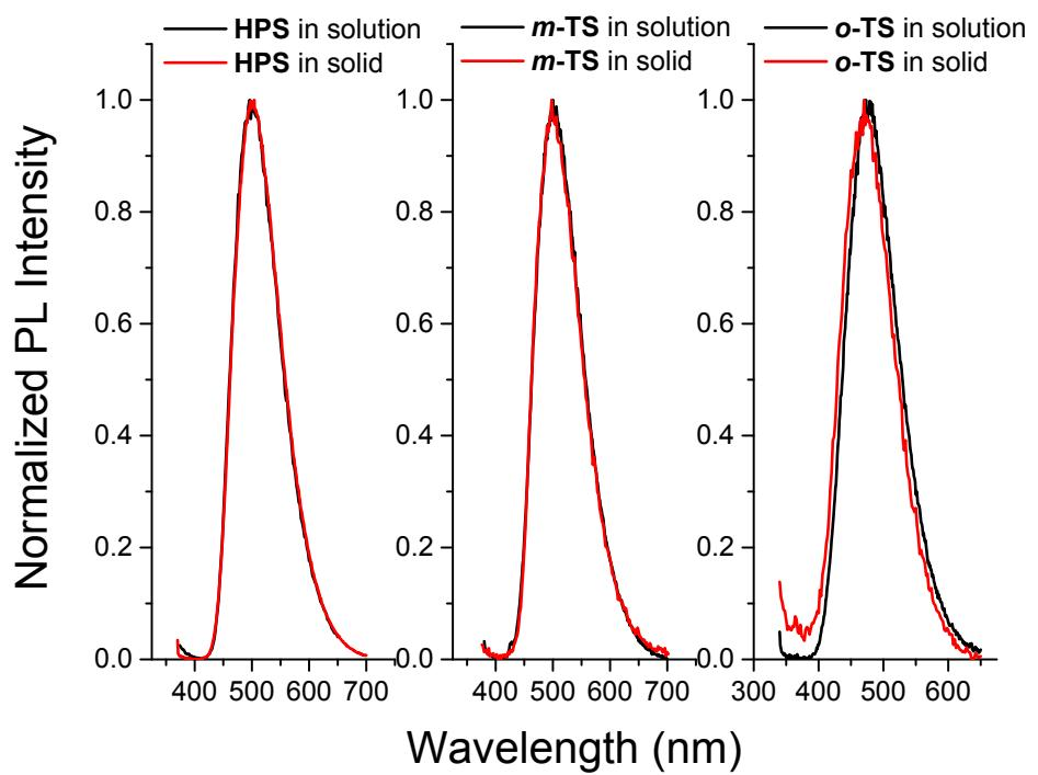
**Figure S4.** Photoluminescence spectra of **HPS**, ***m*-TS**, and ***o*-TS** in acetone/water ( $f_w = 90\%$ ) and solid-state thin layers absorbed on the TLC plates.
