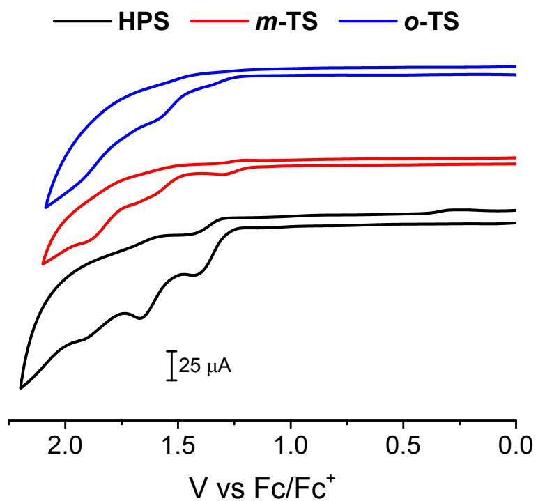
**Figure S3.** Cyclic voltammograms of **HPS**, ***m*-TS**, and ***o*-TS** in dichloromethane solution containing 0.1 M  $n\text{-Bu}_4\text{NPF}_6$  as electrolyte, at a scan rate of  $0.1 \text{ V s}^{-1}$ .
