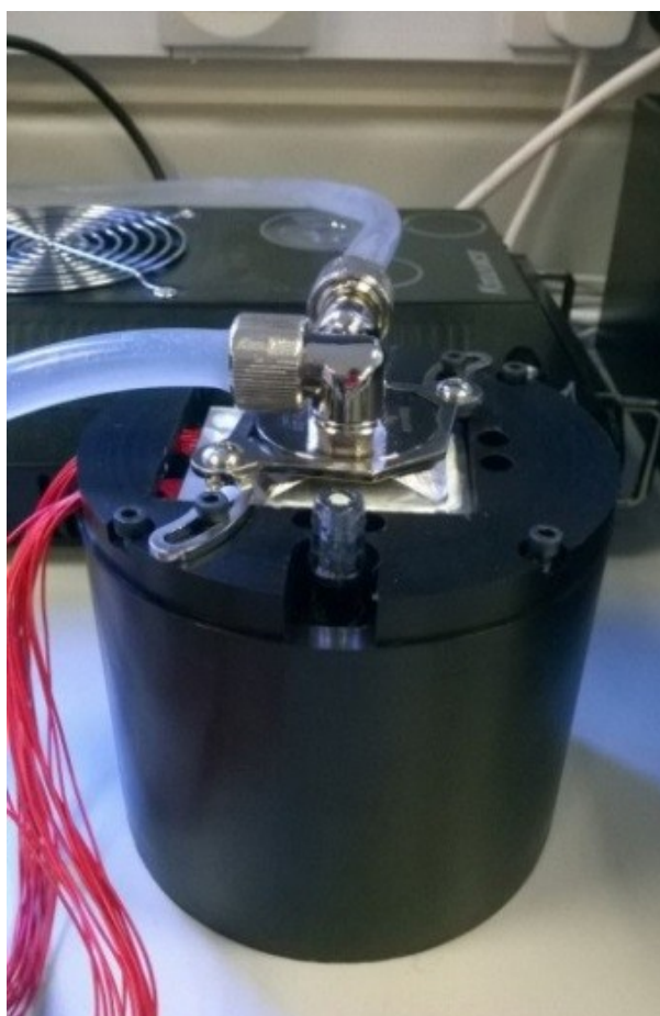
Figure S1. Image of reactor in Fig. 2a. UV-LEDs are located at top.
