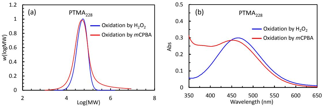
**Figure S5.** Comparison of two different oxidation methods to convert PTMPM<sub>228</sub> to PTMA<sub>228</sub>, (a) SEC traces and (b) the UV-Vis spectra of PTMA<sub>228</sub> oxidised by  $H_2O_2$  in methanol and  $mCPBA$  in dichloromethane.
