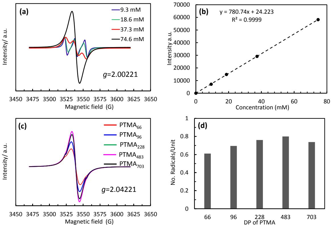
**Figure S7.** Oxidation efficiency determined by EPR: (a) EPR spectra of 4-hydroxyl TEMPO with different concentration in DCM, (b) Calibration curve based on integration of EPR spectra (c) EPR spectra of PTMA with different DPs oxidised from PTMPM by H<sub>2</sub>O<sub>2</sub> and (d) Number of radicals per unit vs DP of PTMA determined by EPR.
