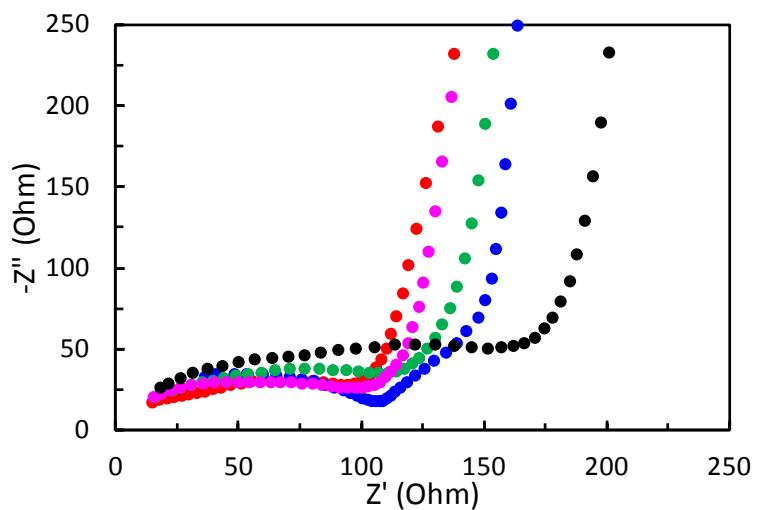
**Figure S11.** Nyquist plot of PTMA with different DPs as cathode at mass ratio of PTMA/SP carbon/PVdF=0.25/0.65/0.1, and 0.1 M LiPF<sub>6</sub> in DMC as electrolyte.
