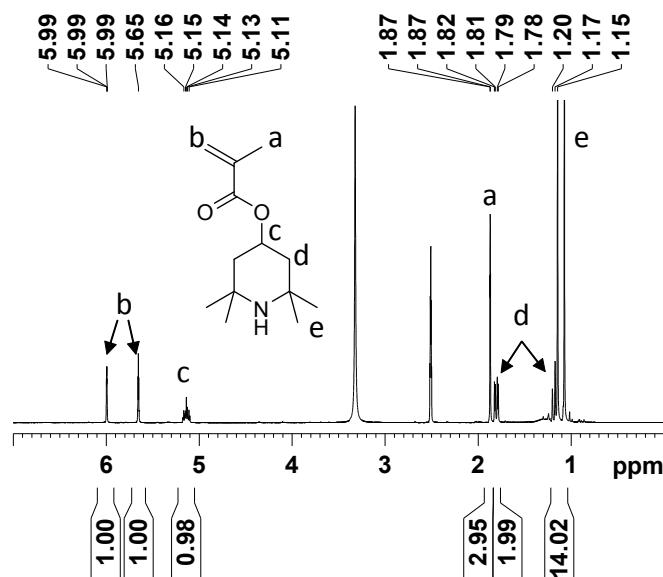
**Figure S1.**  $^1\text{H}$  NMR spectrum (400MHz) of 2,2,6,6-tetramethylpiperidin-4-yl methacrylate (TMMPM) in  $\text{DMSO}-d_6$ .
