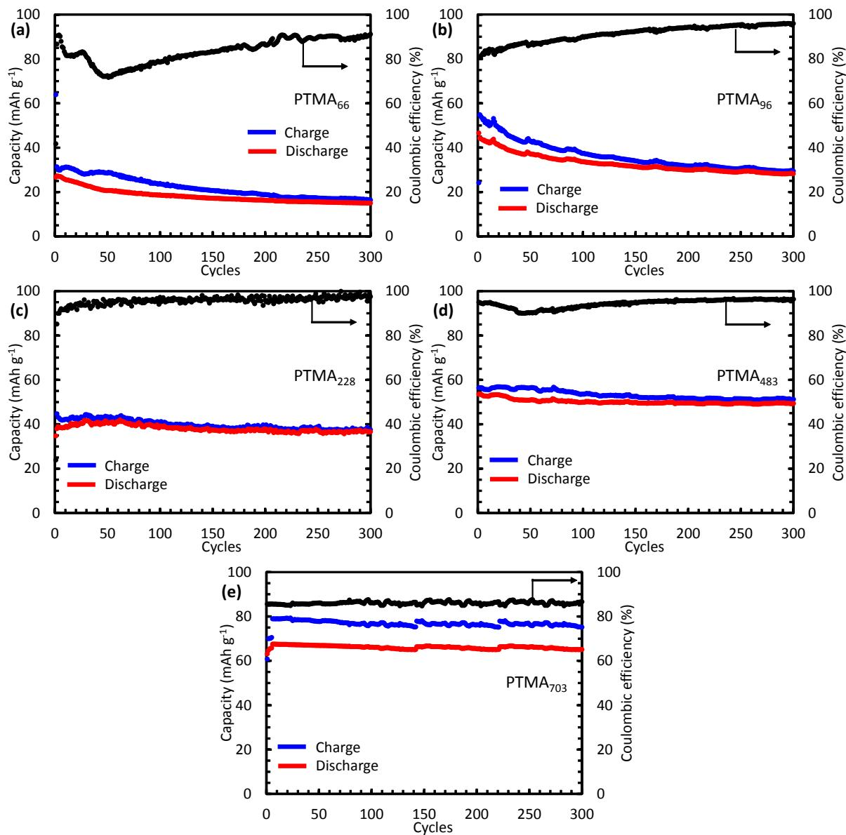
**Figure S10.** Cycling property and coulombic efficiency of (a) PTMA<sub>66</sub>, (b) PTMA<sub>96</sub>, (c) PTMA<sub>228</sub>, (d) PTMA<sub>483</sub>, and (e) PTMA<sub>703</sub> as cathode with mass ratio of PTMA/SP carbon/PVdF=0.25/0.65/0.1, charging/discharging at 1C over 300 cycles.
