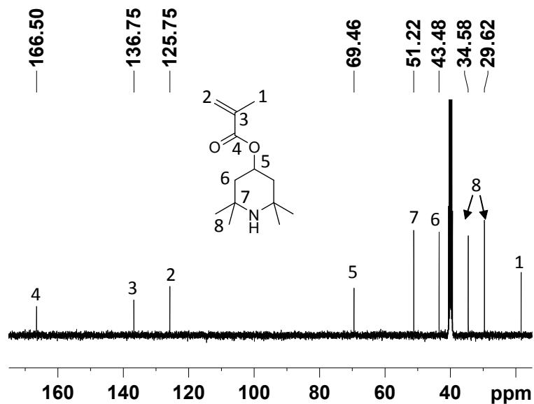
**Figure S2.**  $^{13}\text{C}$  NMR spectrum (100MHz) of 2,2,6,6-tetramethylpiperidin-4-yl methacrylate (TMMPM) in  $\text{DMSO}-d_6$ .
