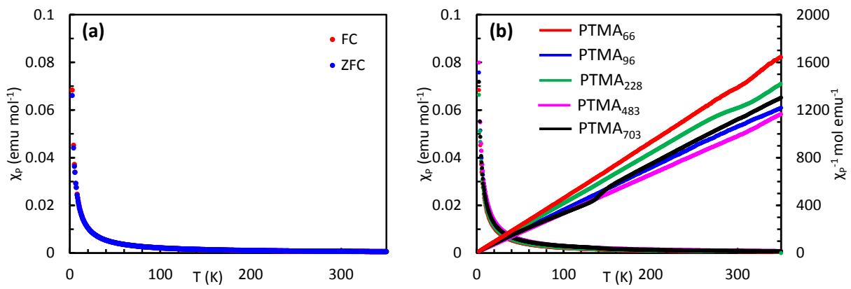
**Figure S9.** (a) Temperature dependence of the paramagnetic susceptibility  $\chi_P$  of PTMA<sub>66</sub> with both field cooling (FC) and zero-field cooling (ZFC) modes. (b) Temperature dependence of the paramagnetic susceptibility  $\chi_P$  and its inverse  $\chi_P^{-1}$  of all PTMA polymers with FC mode. All the measurements carried out at an applied magnetic field strength of 10 KOe.
