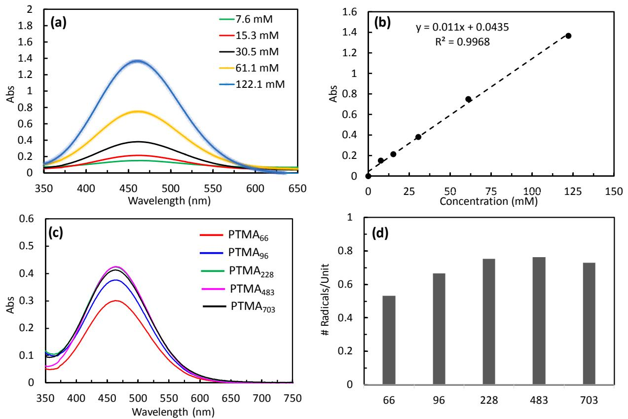
**Figure S8.** Oxidation efficiency determined by UV-Vis: (a) Absorption of 4-hydroxyl TEMPO with different concentration in DCM, (b) Calibration curve (c) Absorption of PTMA with different DPs oxidised from PTMPM by H<sub>2</sub>O<sub>2</sub> and (d) Number of radicals per unit vs DP of PTMA determined by UV-Vis.
