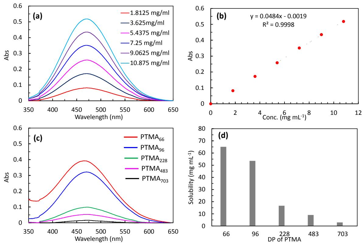
**Figure S6.** Solubility of PTMA in DMC with 1 M LiPF<sub>6</sub> determined by UV-Vis: (a) Absorption of 4-hydroxyl TEMPO with different concentration in THF, (b) Calibration curve (c) Absorption of PTMA in THF and (d) Solubility of PTMA with different DPs determined by UV-Vis.
