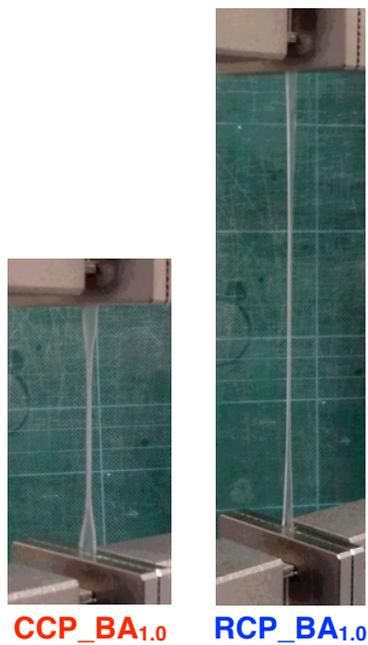
**Figure S7.** Pictures of tensile tests of **RCP\_BA<sub>1.0</sub>** and **CCP\_BA<sub>1.0</sub>**, taken just before fracture
