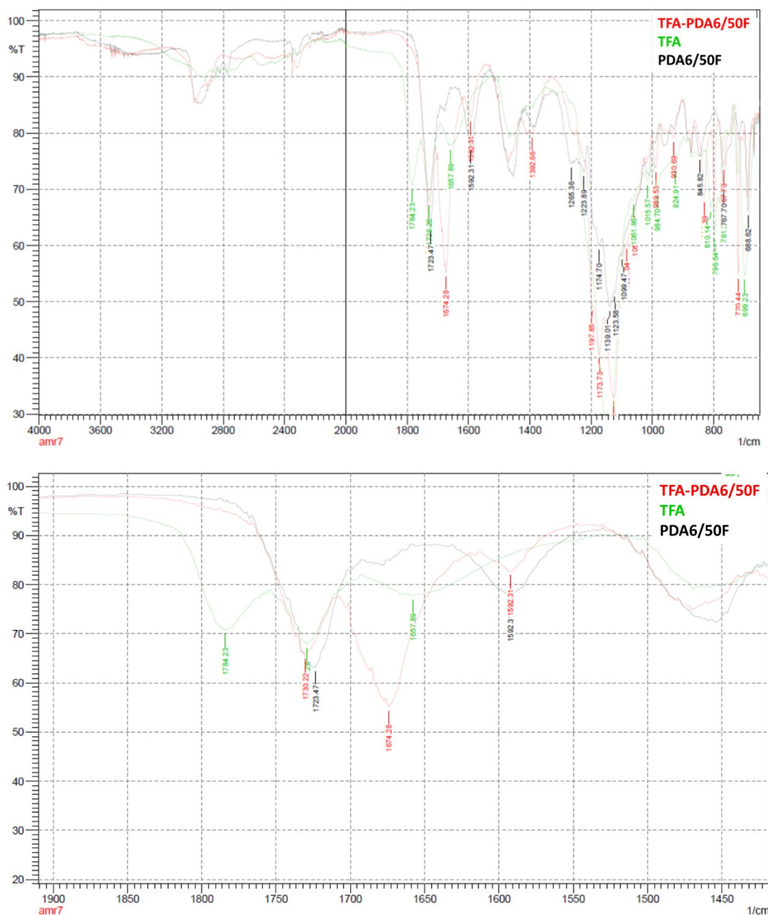
Figure S16. FTIR spectra of PDA6/50F , trifluoroacetic acid ( TFA ) and the resulting salt TFA-PDA6/50F showing the red-shift of the C=O stretching frequency of TFA (top) and magnification of the region 1400-1900 \text{cm}^{-1} (bottom).
