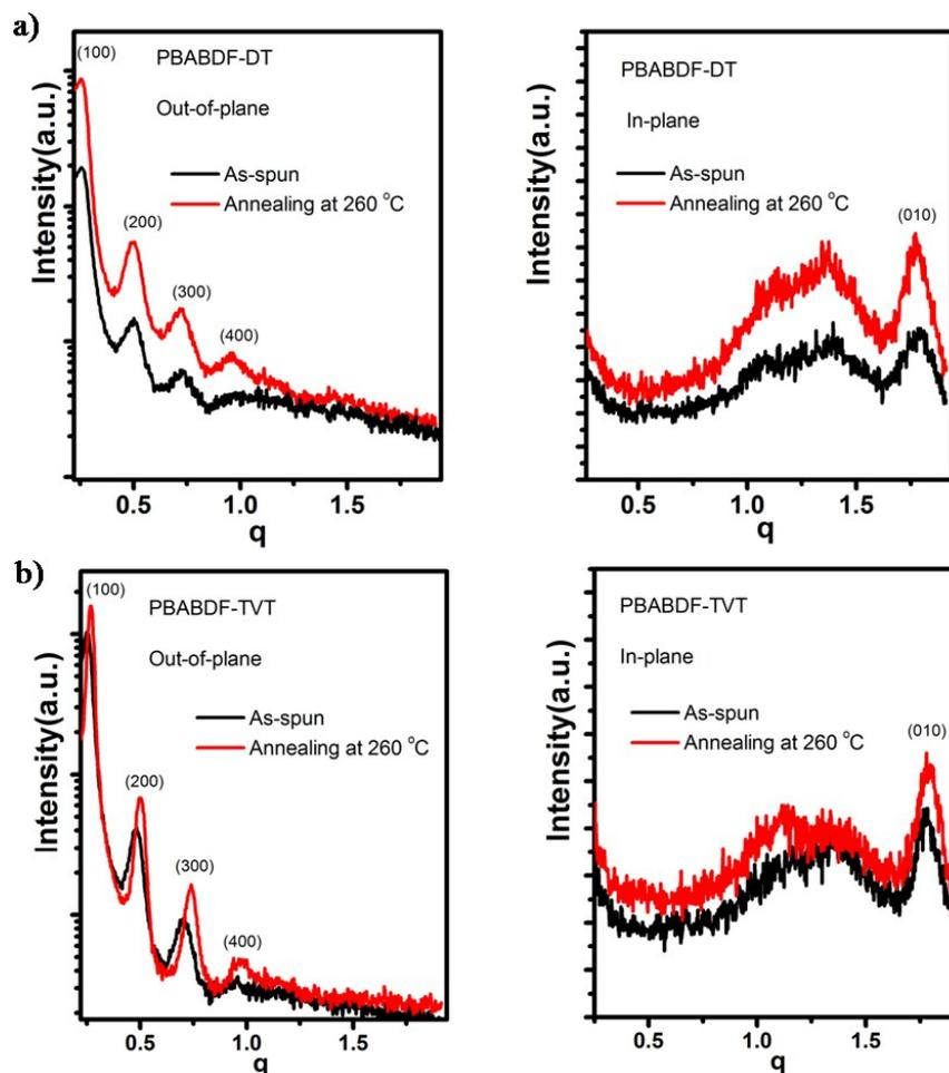
Fig. S6 Out-of-plane and in-plane line cuts of GIXD.
