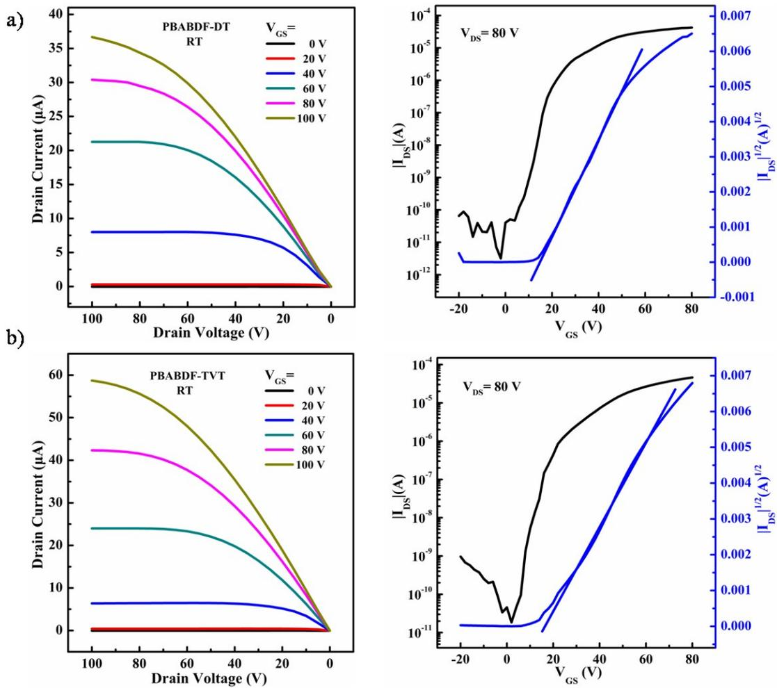
**Fig. S4** Transfer and output characteristics of **BABDF**-based polymer films without annealing.
