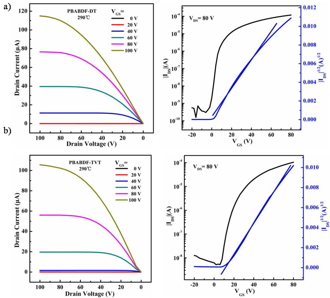
**Fig. S5** Transfer and output characteristics of **BABDF**-based polymer films annealed 290 °C in BG/TC devices.
