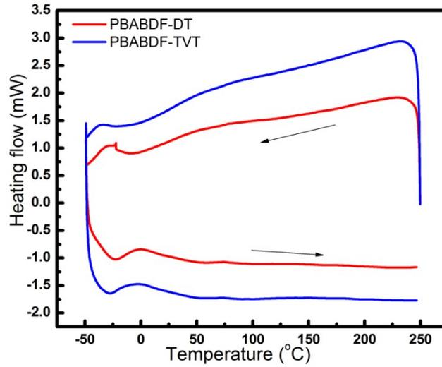
**Fig. S3** The DSC plots of **BABDF**-based polymers.
