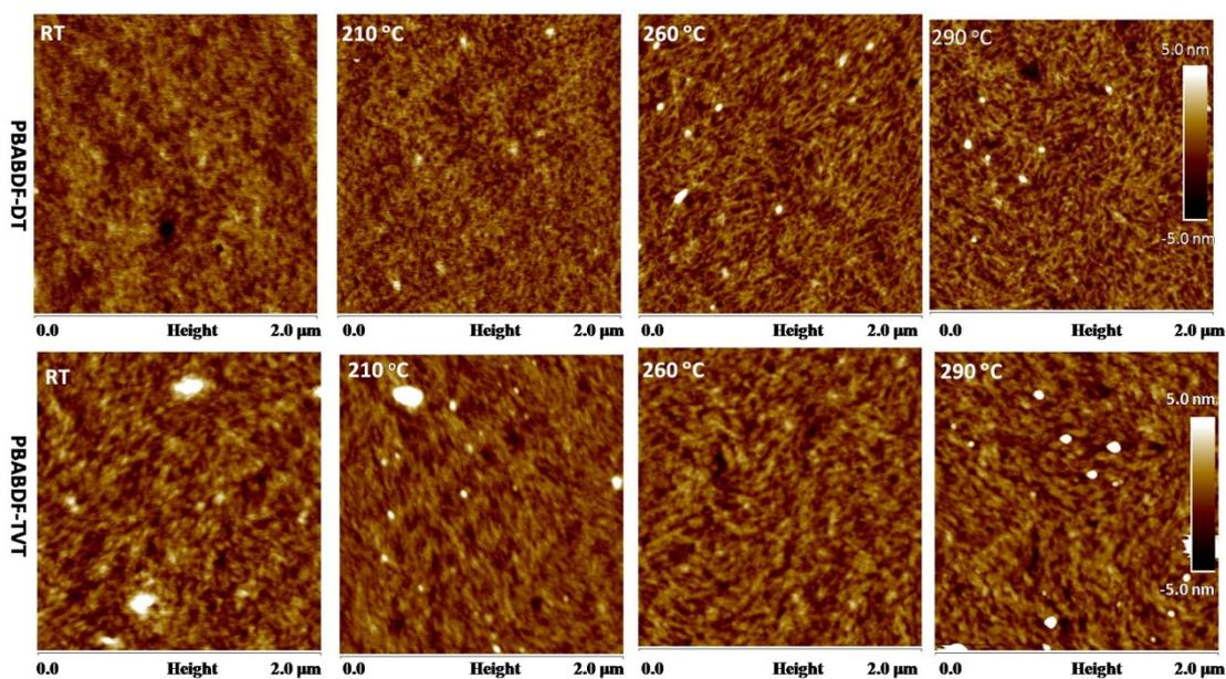
Fig. S7 AFM topography images of polymer films coated on Cytosol-modified  $\text{SiO}_2/\text{Si}$  substrate with and without annealing.
