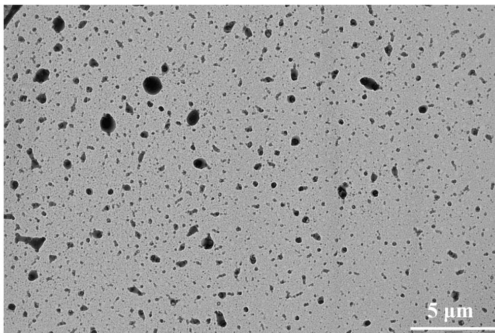
**Figure S21.** TEM images of PVDF<sub>40</sub>-*b*-PDMAEMA<sub>69</sub> amphiphilic block copolymers self-assembled in water (pH = 10).
