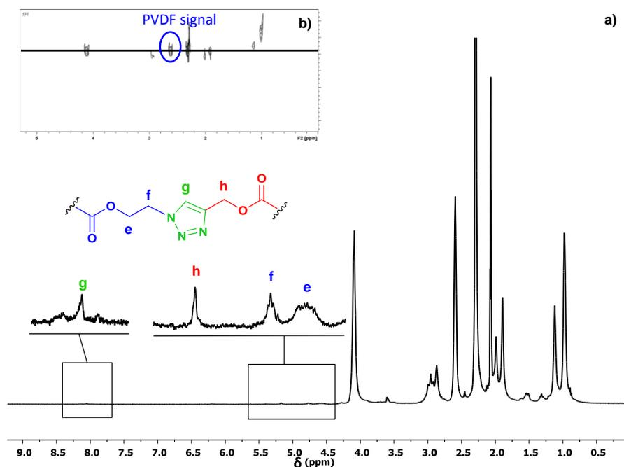
**Figure S8.** a) <sup>1</sup>H NMR spectrum in (CD<sub>3</sub>)<sub>2</sub>CO of PVDF<sub>40</sub>-*b*-PDMAEMA<sub>162</sub> BCP, b) DOSY <sup>1</sup>H NMR spectrum of PVDF<sub>40</sub>-*b*-PDMAEMA<sub>162</sub> BCP.
