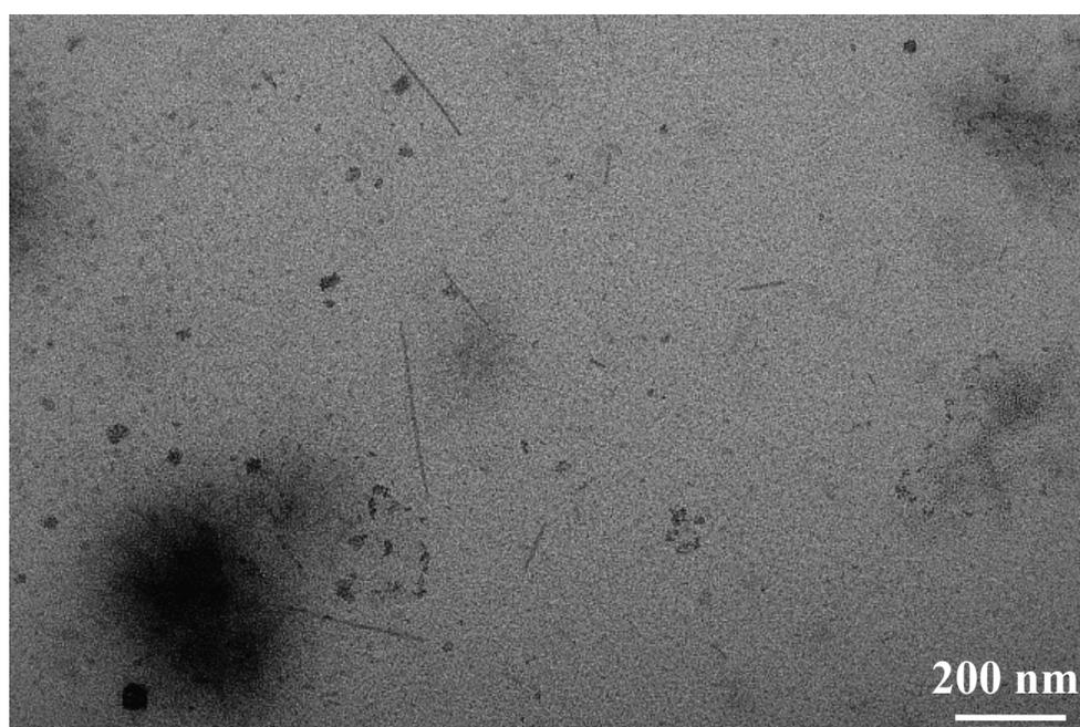
**Figure S20.** TEM images of PVDF<sub>40</sub>-*b*-PDMAEMA<sub>69</sub> amphiphilic block copolymers self-assembled in water, zoom on rod morphologies (pH = 8).
