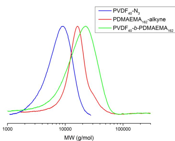
**Figure S9.** SEC chromatograms of PVDF<sub>40</sub>-N<sub>3</sub>, of ≡-PDMAEMA<sub>162</sub> and of the resulting PVDF<sub>40</sub>-*b*-PDMAEMA<sub>162</sub> BCP.
