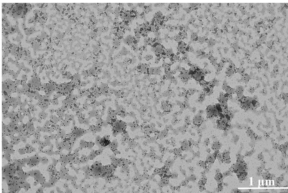
**Figure S17.** TEM images of PVDF<sub>40</sub>-*b*-PDMAEMA<sub>69</sub> amphiphilic block copolymers self-assembled in water (pH = 2).
