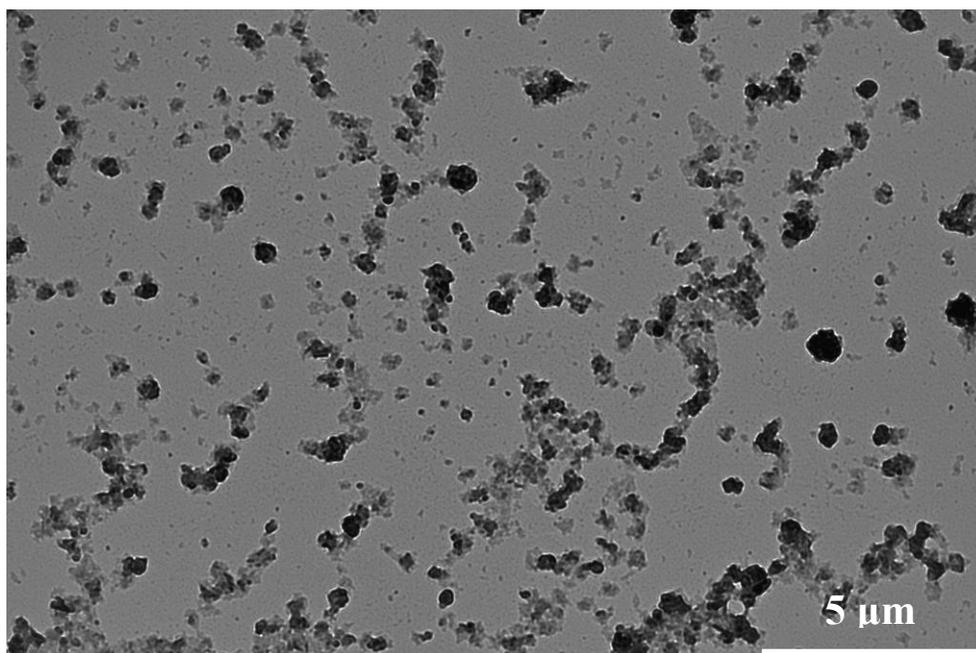
**Figure S14.** TEM images of PVDF<sub>40</sub>-*b*-PDMAEMA<sub>23</sub> amphiphilic block copolymers self-assembled in water. (pH = 2)
