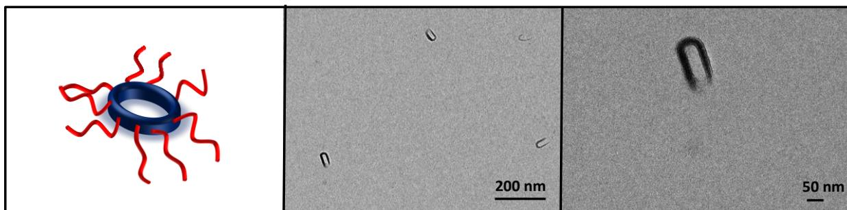
**Figure S24.** TEM morphologies of PVDF<sub>40</sub>-*b*-PDMAEMA<sub>162</sub> amphiphilic block copolymers self-assembled in water, zoom on ring morphologies (pH = 8).
