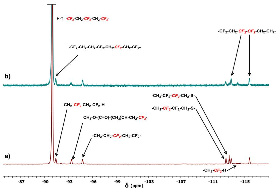
**Figure S2.**  $^{19}\text{F}$  NMR spectra in  $(\text{CD}_3)_2\text{CO}$  of: a)  $\text{N}_3\text{-PVDF}_{40}\text{-XA}$  and b)  $\text{PVDF}_{40}\text{-}b\text{-PDMAEMA}_{23}$  BCP. H-T stands for head-to-tail.
