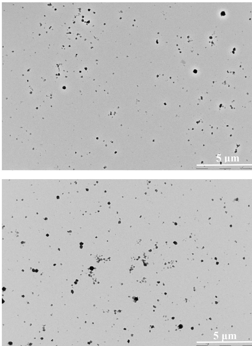
**Figure S15.** TEM images of PVDF<sub>40</sub>-*b*-PDMAEMA<sub>23</sub> amphiphilic block copolymers self-assembled in water (pH = 8).
