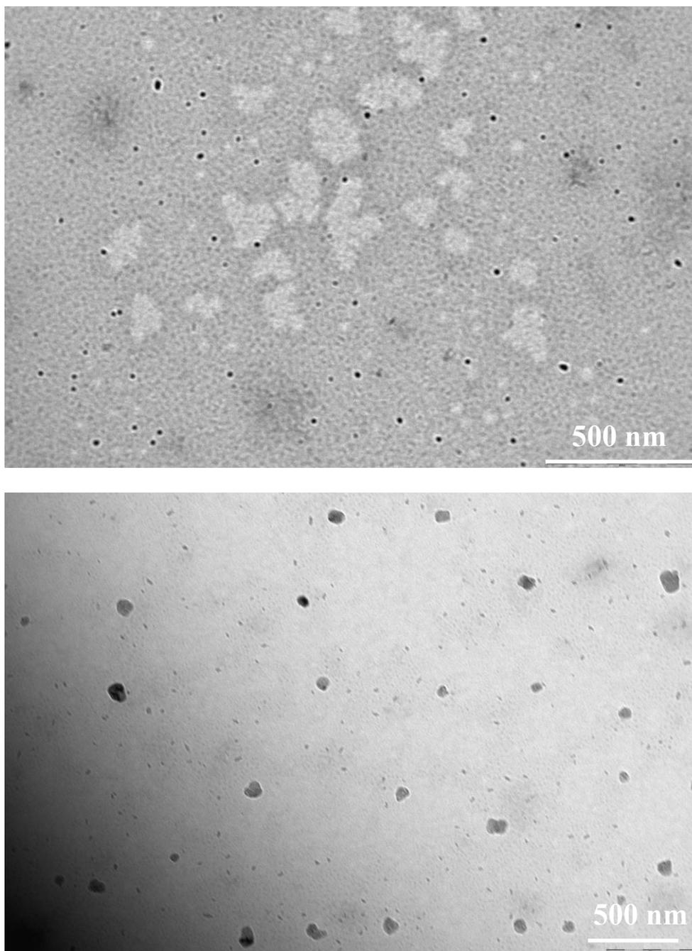
**Figure S22.** TEM images of PVDF<sub>40</sub>-*b*-PDMAEMA<sub>162</sub> amphiphilic block copolymers self-assembled in water (pH = 2).
