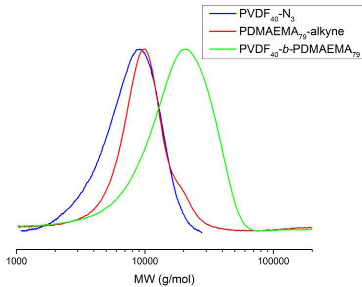
**Figure S7.** SEC chromatograms of PVDF<sub>40</sub>-N<sub>3</sub>, ≡-PDMAEMA<sub>79</sub> and of the resulting PVDF<sub>40</sub>-*b*-PDMAEMA<sub>79</sub> BCP.
