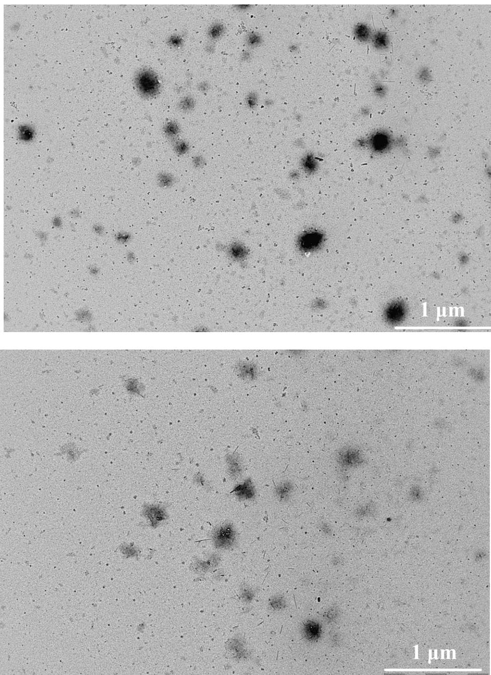
**Figure S18.** TEM images of PVDF<sub>40</sub>-*b*-PDMAEMA<sub>69</sub> amphiphilic block copolymers self-assembled in water (pH = 8).
