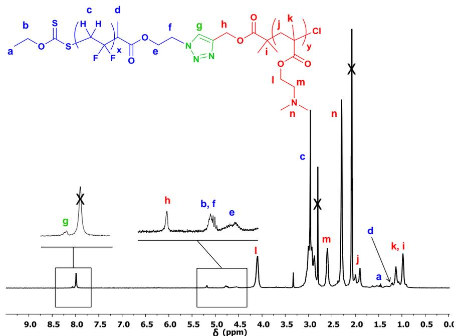
**Figure S1.** <sup>1</sup>H NMR spectrum in (CD<sub>3</sub>)<sub>2</sub>CO of PVDF<sub>40</sub>-*b*-PDMAEMA<sub>23</sub> BCP. The crossed-out peaks were assigned to residual (CH<sub>3</sub>)<sub>2</sub>CO and DMF.
