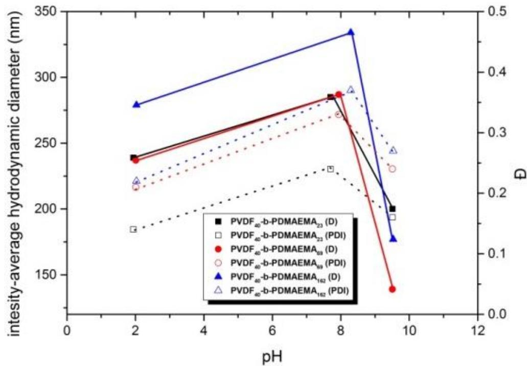
**Figure S13.** Evolution of the intensity-average hydrodynamic diameter and of the dispersity of PVDF-*b*-PDMAEMA amphiphilic block copolymers self-assembled nano-objects versus pH of the dispersions.
