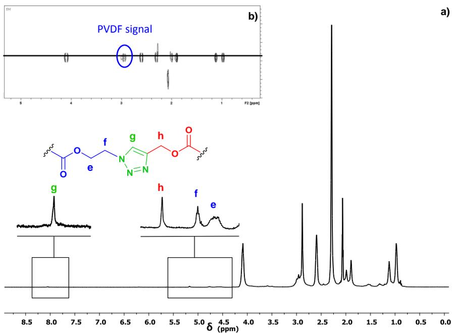
**Figure S6.** a) <sup>1</sup>H NMR spectrum in (CD<sub>3</sub>)<sub>2</sub>CO of PVDF<sub>40</sub>-b-PDMAEMA<sub>79</sub> BCP, b) DOSY <sup>1</sup>H NMR spectrum of PVDF<sub>40</sub>-b-PDMAEMA<sub>79</sub> BCP.
