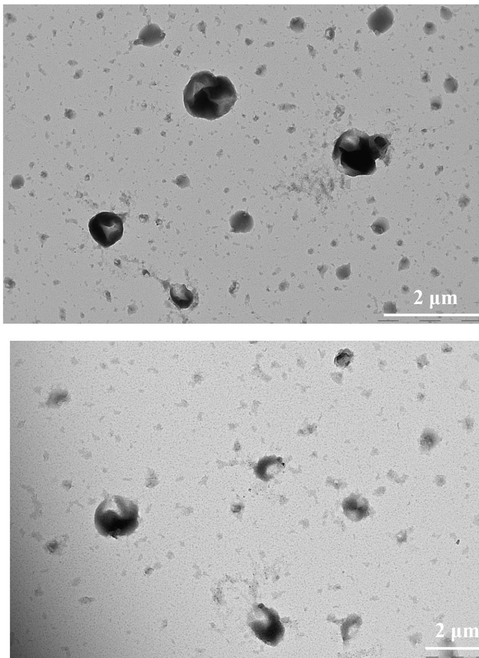
**Figure S25.** TEM images of PVDF<sub>40</sub>-*b*-PDMAEMA<sub>162</sub> amphiphilic block copolymers self-assembled in water (pH = 10).
