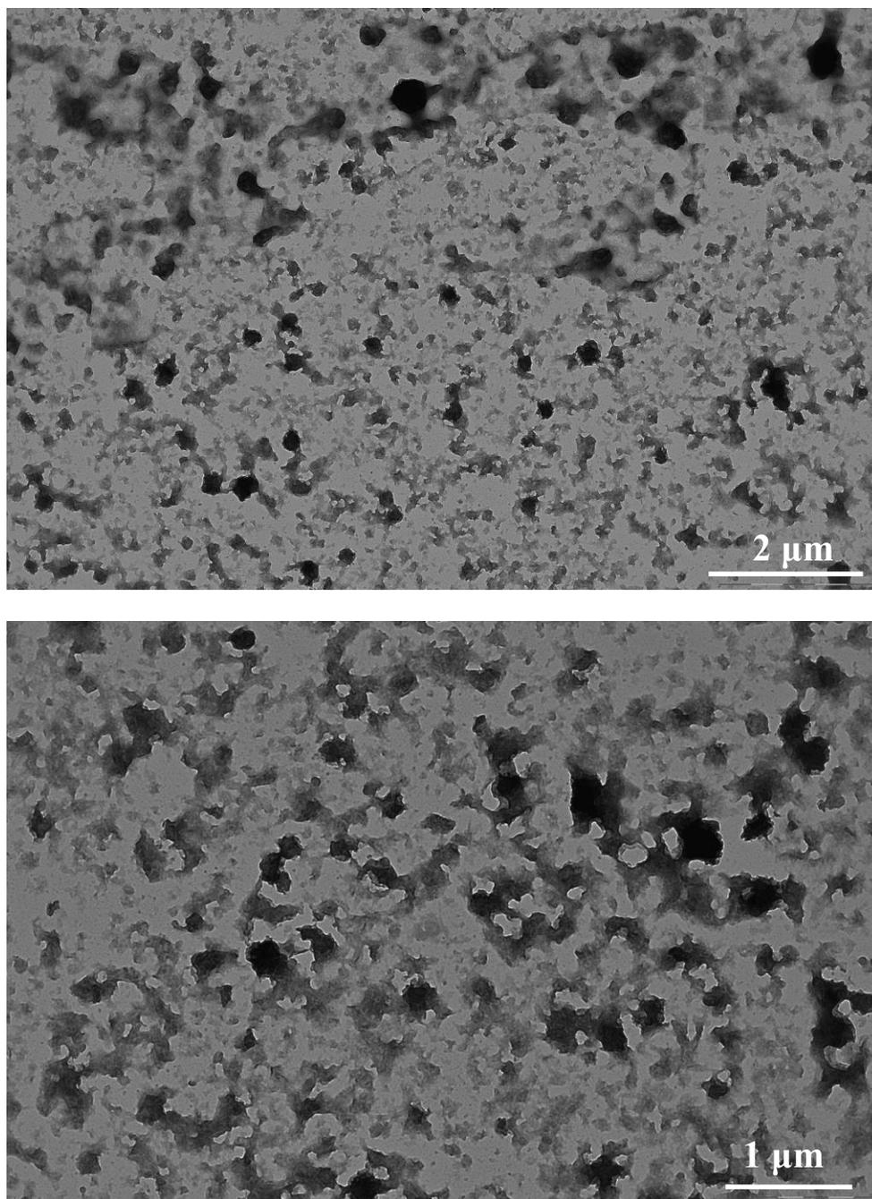
**Figure S16.** TEM images of PVDF<sub>40</sub>-*b*-PDMAEMA<sub>23</sub> amphiphilic block copolymers self-assembled in water (pH = 10).
