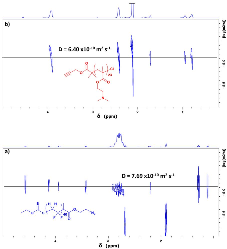
**Figure S4.** DOSY  $^1\text{H}$  NMR spectra in  $(\text{CD}_3)_2\text{CO}$  of: a)  $\text{N}_3\text{-PVDF}_{40}\text{-XA}$ , and b)  $\text{PDMAEMA-Cl}$ .
