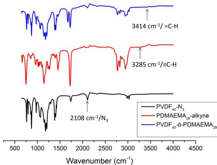
**Figure S5.** FTIR spectra of PVDF<sub>40</sub>-N<sub>3</sub> (black trace), ≡-PDMAEMA<sub>29</sub> (red trace) and of the resulting PVDF<sub>40</sub>-b-PDMAEMA<sub>29</sub> BCP (blue trace).
