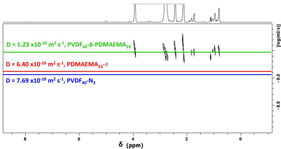
**Figure S3.** DOSY  $^1\text{H}$  NMR spectrum in  $(\text{CD}_3)_2\text{CO}$  of  $\text{PVDF}_{40}\text{-}b\text{-PDMAEMA}_{23}$  BCP (green line and black contours). The other colored lines correspond to the diffusion coefficients of the  $\text{N}_3\text{-PVDF}_{40}\text{-XA}$  (blue line) and  $\equiv\text{-PDMAEMA-Cl}$  (red line) building blocks. The  $^1\text{H}$  DOSY NMR spectra of these precursors are displayed in Figure S4.
