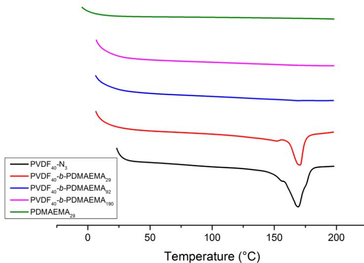
**Figure S10.** DSC thermograms (second heating) of PVDF<sub>40</sub>-N<sub>3</sub> (black trace), PVDF<sub>40</sub>-*b*-PDMAEMA<sub>29</sub> (red trace), PVDF<sub>40</sub>-*b*-PDMAEMA<sub>92</sub> (blue trace), PVDF<sub>40</sub>-*b*-PDMAEMA<sub>162</sub> (pink trace), and PDMAEMA<sub>29</sub> (green trace).
