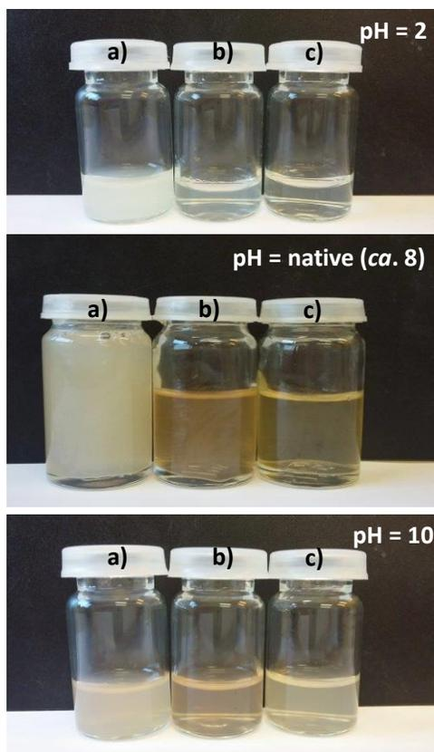
**Figure S11.** Macroscopic aspects of: a) PVDF<sub>40</sub>-*b*-PDMAEMA<sub>23</sub>, b) PVDF<sub>40</sub>-*b*-PDMAEMA<sub>69</sub>, and c) PVDF<sub>40</sub>-*b*-PDMAEMA<sub>162</sub> self-assembled dispersions in water
