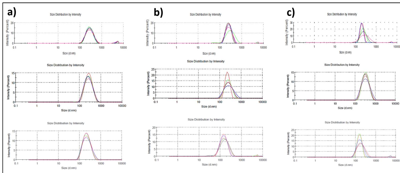
**Figure S12.** Comparison of intensity-average hydrodynamic diameter distributions of :a) PVDF<sub>40</sub>-*b*-PDMAEMA<sub>23</sub>, b) PVDF<sub>40</sub>-*b*-PDMAEMA<sub>69</sub>, and c) PVDF<sub>40</sub>-*b*-PDMAEMA<sub>162</sub> amphiphilic block copolymers self-assembled in water at pH = 2, 8 and 10.
