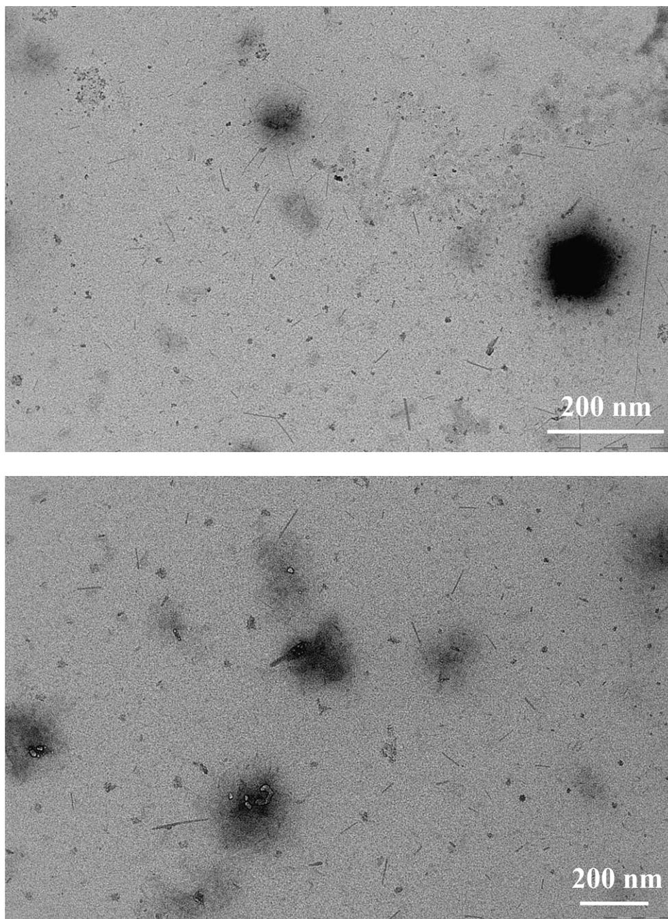
**Figure S19.** TEM images of PVDF<sub>40</sub>-*b*-PDMAEMA<sub>69</sub> amphiphilic block copolymers self-assembled in water, zoom on rod morphologies (pH = 8).
