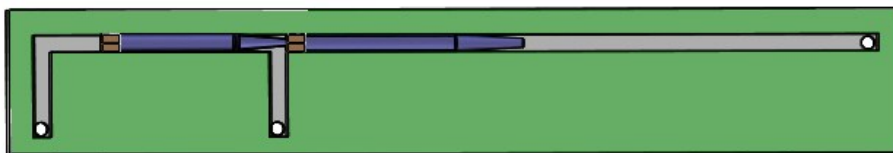
Fig. S5 Epoxy resin was filled in the blanks between capillary tube and square channel.
