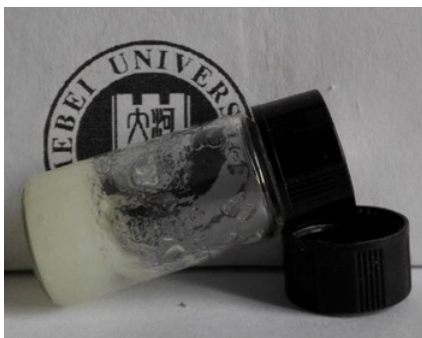
Fig. S7 Hydrogel from P(DMA 93 - stat -DAA 30 ) cross-linked by DTDPH did not show gel-sol transition by DTT reduction.
