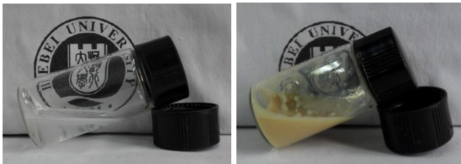
Fig. S6 The DTT reduced hydrogel after addition of (left) H 2 O 2 and (right) Fe 2 O 3 .
