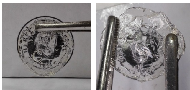
Fig. S2 Repeated self-healing of hydrogel prepared from P(DMA 96 - stat -DAA 50 ) cross-linked by 5:2 ratio of PEO 23 dihydrazide in 12 h.
