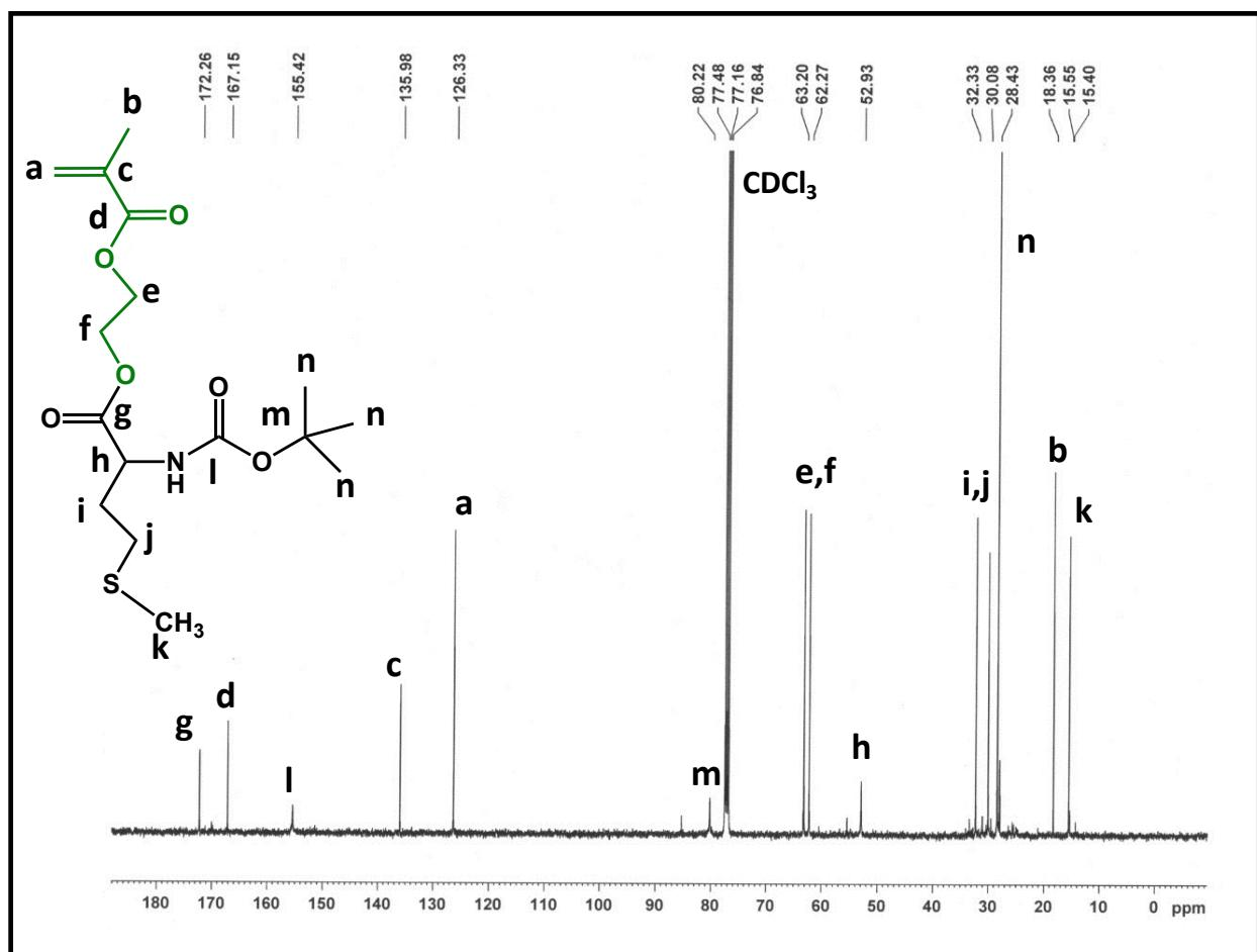
**Figure S4.**  $^{13}\text{C}$  NMR spectrum of Boc-L-methionine-(2-methacryloyloethyl)ester
