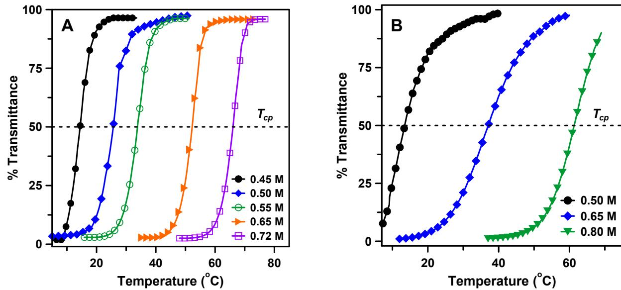
**Figure S15.** Turbidity curves (at  $\lambda = 600$  nm) of zwitterionic PMETMASPS<sub>50</sub> (0.1 wt %) in water in presence of different concentration of (A)  $\text{SO}_4^{2-}$  and (B)  $\text{H}_2\text{PO}_4^-$  anions.
