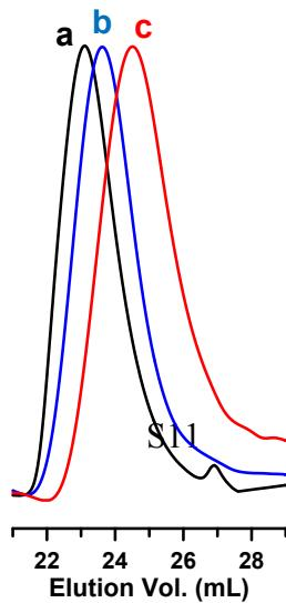
**Figure S11.** SEC traces of (a) PMETMASPS<sub>100</sub>, (b) PMETMASPS<sub>75</sub>, and (c) PMETMASPS<sub>50</sub> samples (Table 1). Eluent for SEC was water with 0.1 M LiBr.
