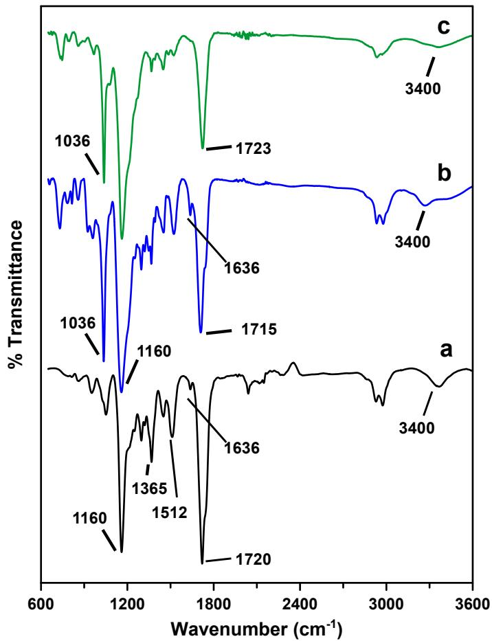
**Figure S9.** FTIR spectra of (a) METMA (b) METMASPS and (c) PMETMASPS acquired in ATR mood.
