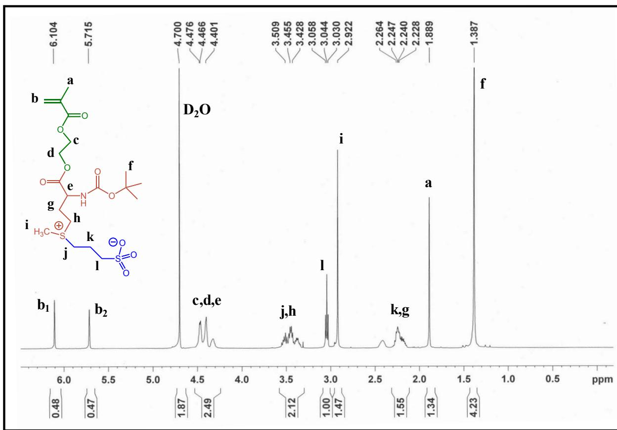
**Figure S6.**  $^1\text{H}$ NMR spectrum of METMASPS (The  $^1\text{H}$  NMR 500 MHz,  $\text{D}_2\text{O}$ , signal at  $\delta$  4.7 ppm corresponds to water present in  $\text{D}_2\text{O}$ ).
