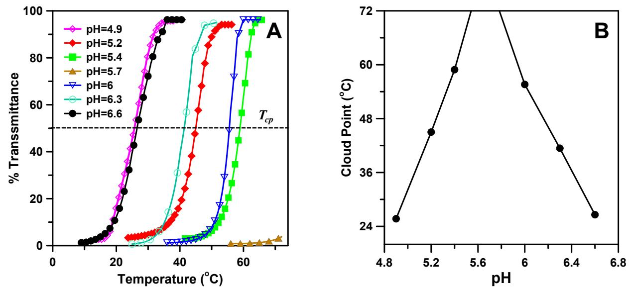
**Figure S12.** (A) Turbidity curves for the aqueous METMASPS monomer solution (1 wt%) at different pHs. (B) The plot of cloud point of the aqueous METMASPS solution (1 wt%) against pH of the solution.
