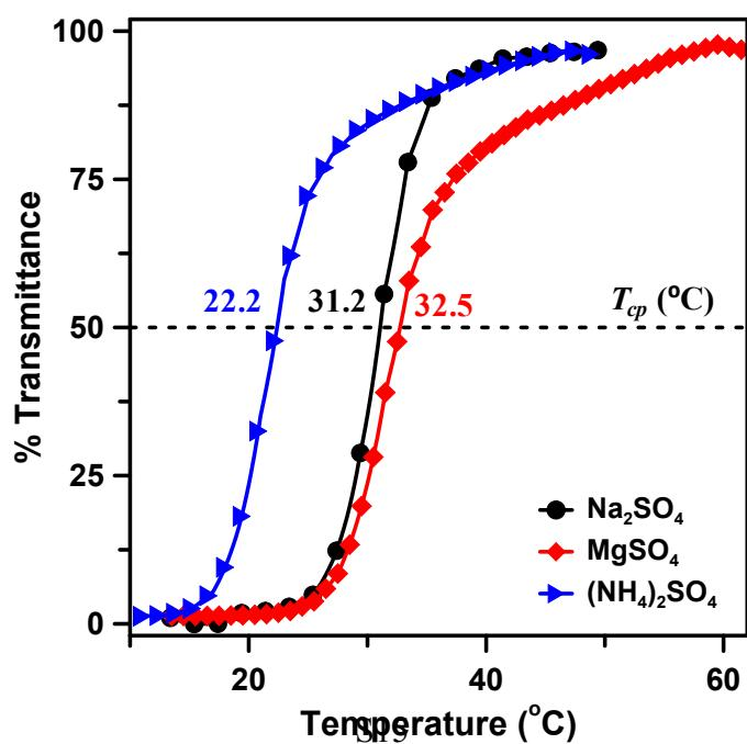
**Figure S18.** Turbidity curves (at  $\lambda = 600$  nm) of aqueous 1 wt % zwitterionic PMETMASPS<sub>75</sub> in presence of 0.5M SO<sub>4</sub><sup>2-</sup> ion from various salts at pH 3.5.
