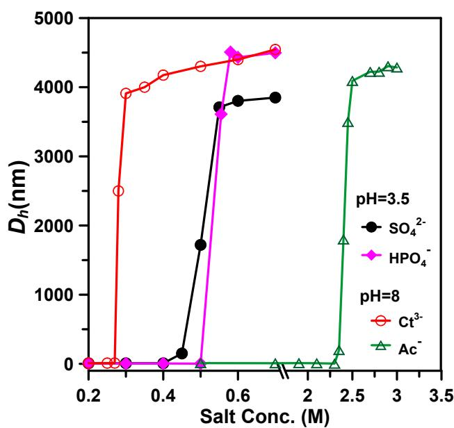
**Figure S14.** Variation of hydrodynamic diameters (measured by DLS) of 1.0 wt % aqueous solution of PMETMASPS<sub>50</sub> with increasing different anions concentration at 25 °C.
