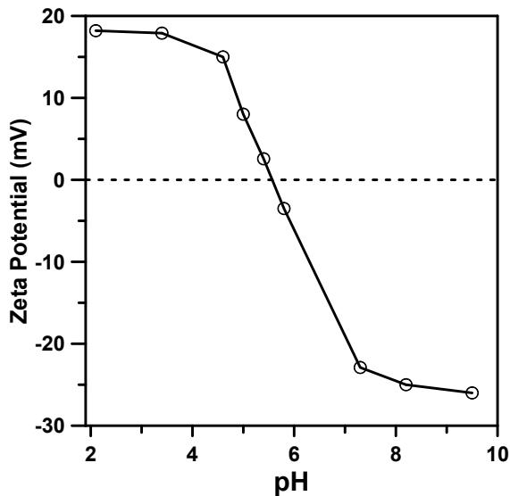
**Figure S13.** Zeta potentials of of 1.0 wt % aqueous solution of PMETMASPS at different pHs at 25 °C.
