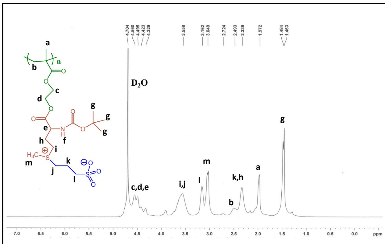
**Figure S10.**  $^1\text{H}$  NMR spectrum of PMETMASPS (The  $^1\text{H}$  NMR 500 MHz,  $\text{D}_2\text{O}$ , signal at  $\delta$  4.7 ppm corresponds to water present in  $\text{D}_2\text{O}$ ).
