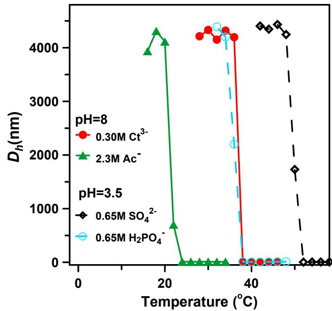
**Figure S17.** Variation of hydrodynamic diameters (measured by DLS) of 1.0 wt % aqueous solution of PMETMASPS<sub>50</sub> with increasing temperature in presence of different kosmotropic anions.
