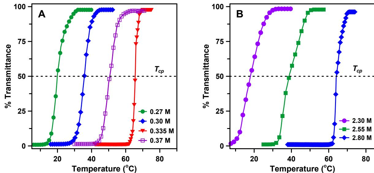
**Figure S16.** Turbidity curves (at  $\lambda = 600$  nm) of zwitterionic PMETMASPS<sub>50</sub> (0.1 wt %) in water in presence of different concentration of (A) Ct<sup>3-</sup> and (B) Ac<sup>-</sup> anions.
