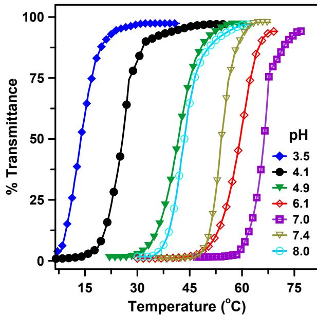
**Figure S19.** Turbidity curves (at  $\lambda = 600$  nm) of zwitterionic PMETMASPS<sub>50</sub> (0.1 wt %) in water in presence of 0.45 M SO<sub>4</sub><sup>2-</sup> at different pHs.
