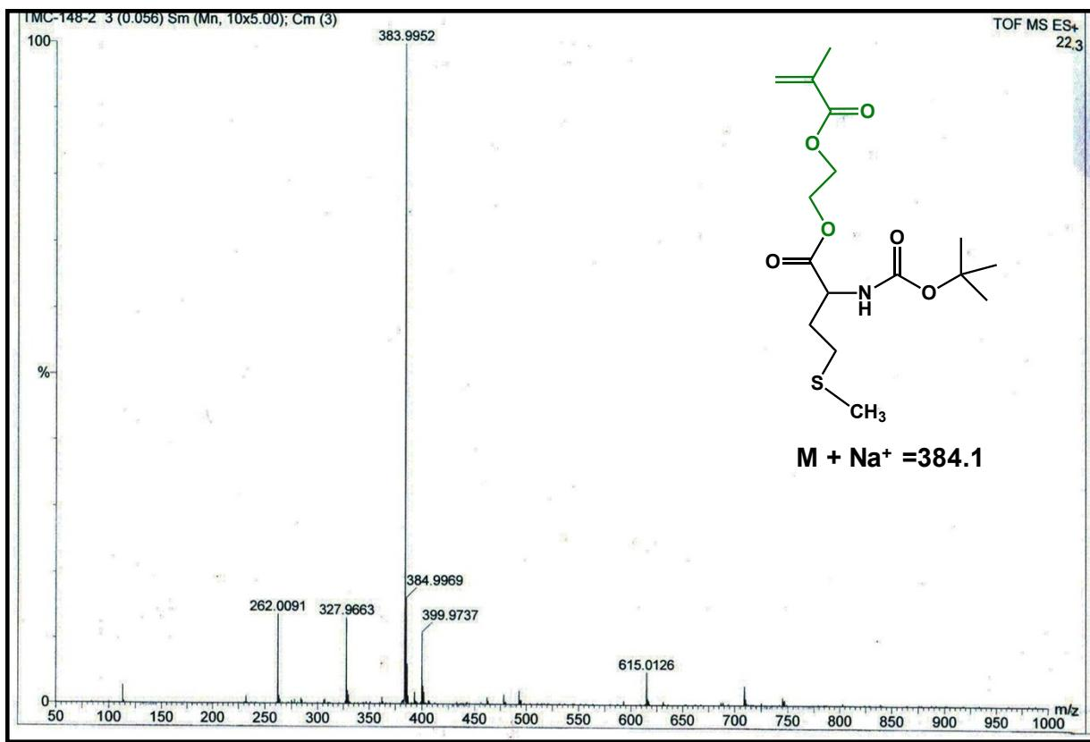
**Figure S5.** ESI-MS spectrum of Boc-L-methionine-(2-methacryloylethyl)ester ( $M/z + Na^+ = 384.1$ ).
