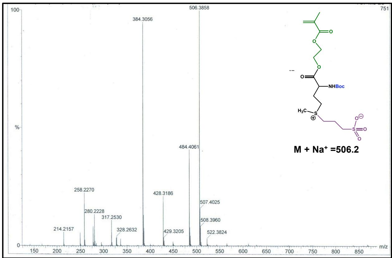
**Figure S8.** ESI-MS spectrum of METMASPS ( $M/z + Na^+ = 506.2$ ).
