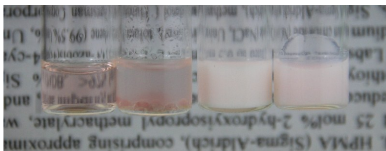
Fig. S1 Digital photos of system before polymerization in (a) methanol/water (b) water, and after 2 h polymerization in (c) methanol/water co-solvent and (d) water
