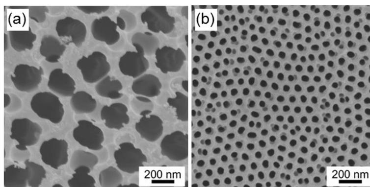
**Figure S1.** (a and b) SEM images of commercial and synthesized AAO templates with the average pore diameter ~230 nm and ~60 nm, respectively.
