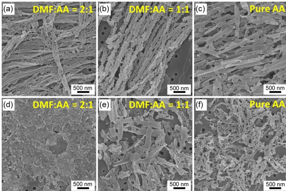
**Figure S2.** (a and b) SEM images of  $PS_{53k}\text{-}b\text{-}PMMA_{20.5k}$  nanostructures prepared by immersing  $PS\text{-}b\text{-}PMMA$  nanotubes in different DMF-to-AA ratios at different times: (a-c) 10 s and (d-f) 12 h.
