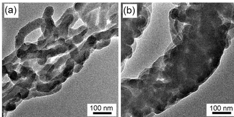
**Figure S3.** (a and b) TEM images of  $PS_{53k}\text{-}b\text{-}PMMA_{20.5k}$  mesoporous structures fabricated by the selective solvent-induced reconstruction method using  $PS\text{-}b\text{-}PMMA/DMF$  solution with concentration of 10 wt % and 20 wt %, respectively. Before the TEM measurements, the mesoporous structures are stained by  $RuO_4$  vapors, which selectively stain the PS blocks.
