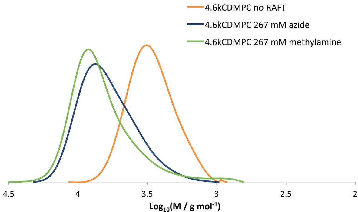
**Figure S11.** Disulphide coupling from thiol-terminated polymers generated after 48 hours of 267 mM sodium azide or methylamine attack on CDMPC CTA.
