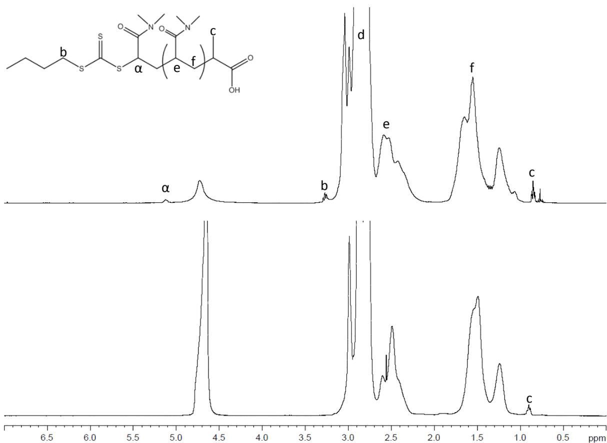
**Figure S5.** <sup>1</sup>H-NMR spectrum of **10kSPAT** polymer before (top, in CDCl<sub>3</sub>) and after treatment (bottom, in D<sub>2</sub>O) with 267 mM sodium azide solution. The α-carbon proton signal (broad, 5.1 ppm) and aliphatic protons from butyl Z group (t, 3.25 ppm) are absent in the water soluble component after treatment with sodium azide, suggesting CTA removal.
