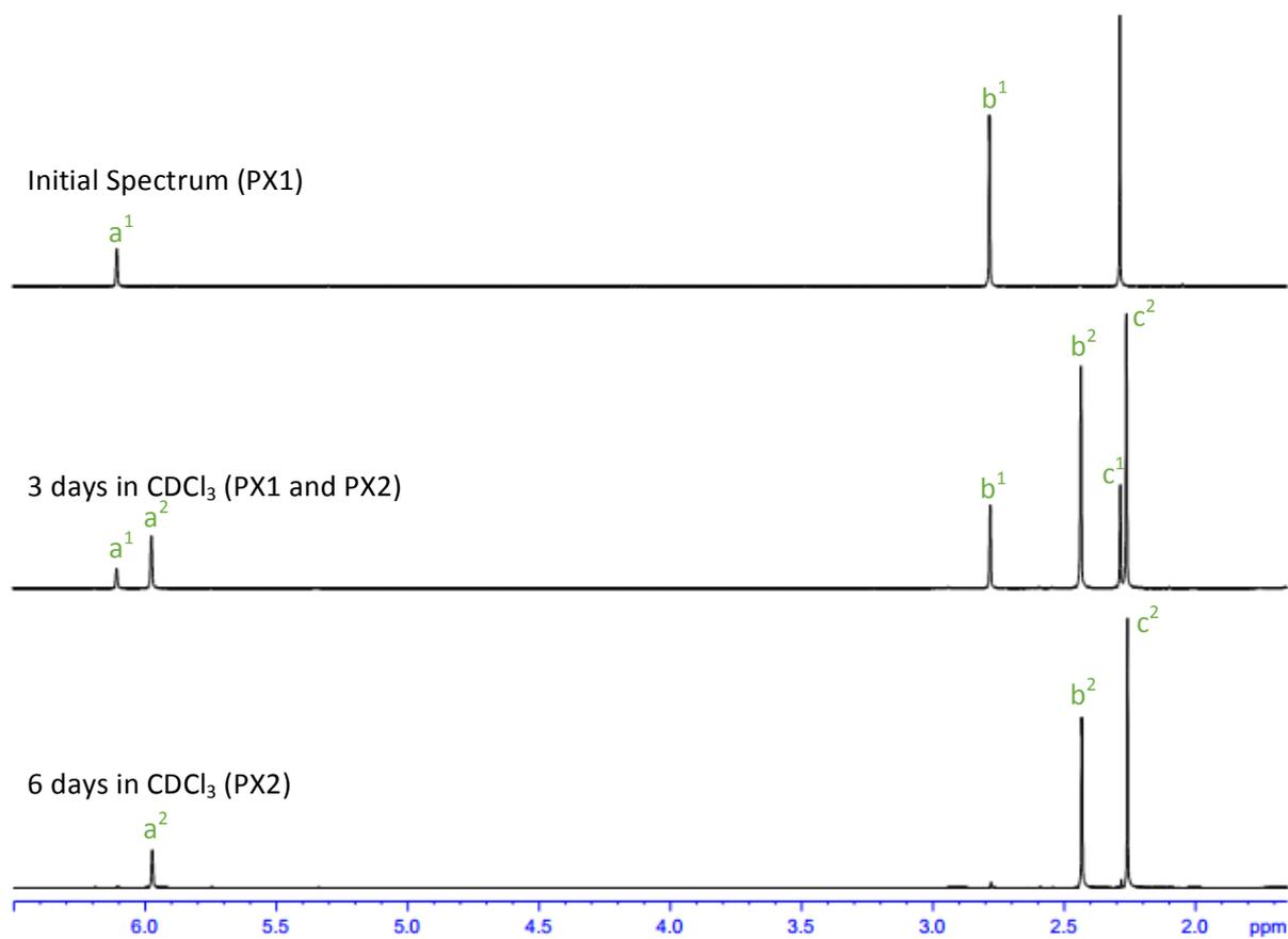
**Figure S14.** <sup>1</sup>H-NMR (CDCl<sub>3</sub>) over time of precipitated solid from sodium azide reaction with 4.6kCDMPC.
