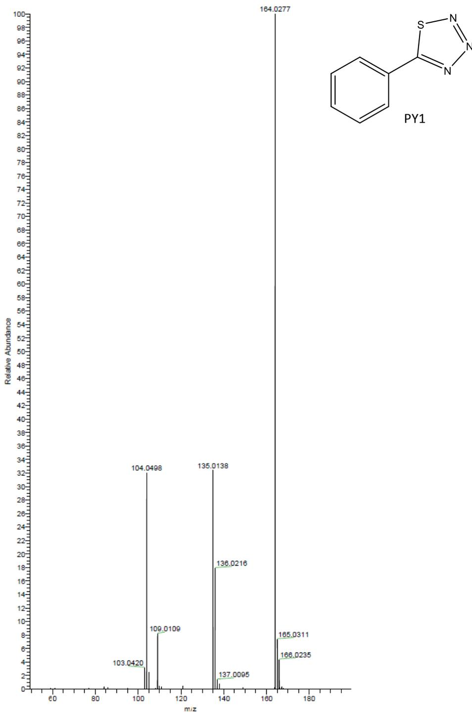
**Figure S17.** Mass spectra for solid precipitate formed after reaction of sodium azide and **5.3kCPDB** (PY1) as analysed by APCI-MS (calculated for  $C_7H_5N_3S + 1H^+$  164.0277, found 164.0277)
