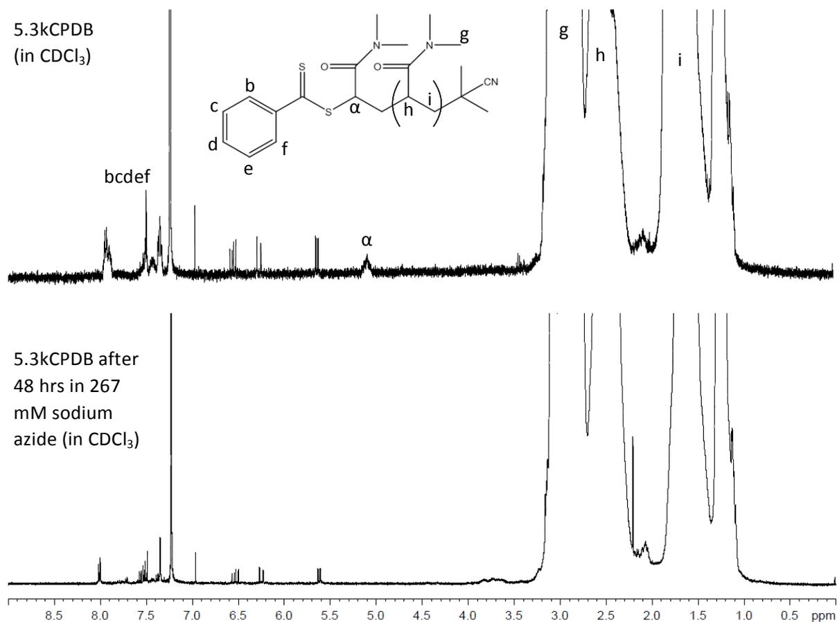
**Figure S9.** <sup>1</sup>H-NMR spectrum of **5.3kCPDB** polymer before (top, in CDCl<sub>3</sub>) and after treatment (bottom, in CDCl<sub>3</sub>) with 267 mM sodium azide solution. The α-carbon proton signal (broad, 5.1 ppm) is while and the aromatic Z group protons (7.3 – 8 ppm) are shifted and reduced in the water soluble component after treatment with sodium azide, suggesting CTA removal.
