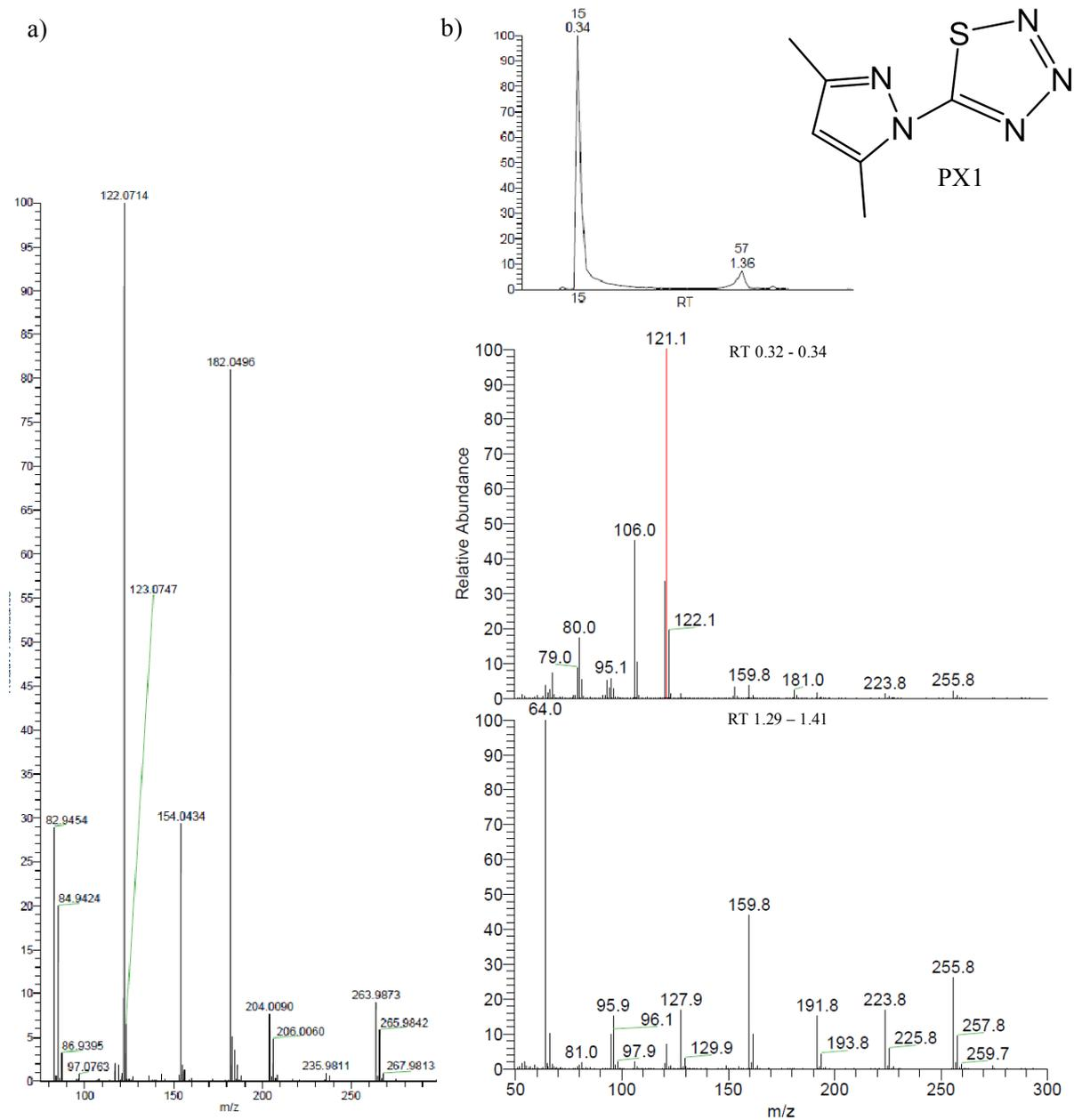
**Figure S15.** Mass spectra for **PX1** as analysed by a) APCI-MS (calculated for  $C_6H_7N_5S + 1H^+$  182.0500, found 182.0496) and b) EI-MS (calculated for  $C_6H_7N_5S$  181.0422, found 181.0; calculated for  $S_8$  255.7767, found 255.8).
