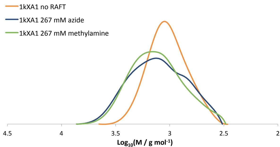
**Figure S13.** Disulphide coupling from thiol-terminated polymers generated after 48 hours of 267 mM sodium azide or methylamine attack on XA1 CTA.
