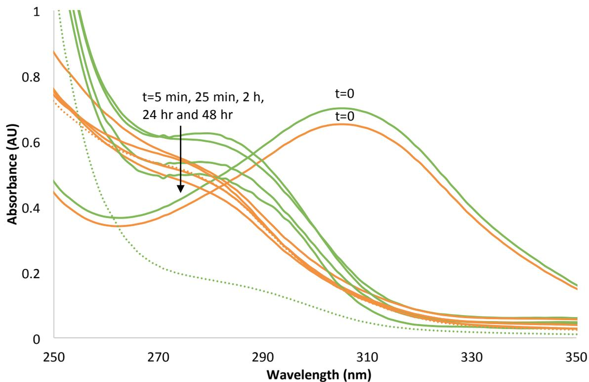
**Figure S4.** UV-vis spectrum for **5.3kCPDB** when reacted with 267 mM sodium azide (green) and methylamine (orange). A precipitate was produced during this reaction and the final measurement (taken at 48 hours) is of a filtered sample.
