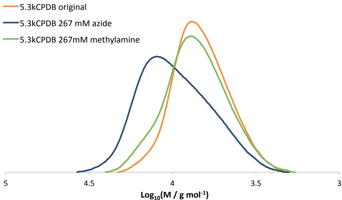
**Figure S12.** Disulphide coupling from thiol terminated polymers generated after 48 hours of 267 mM sodium azide or methylamine attack on CPDB CTA.
