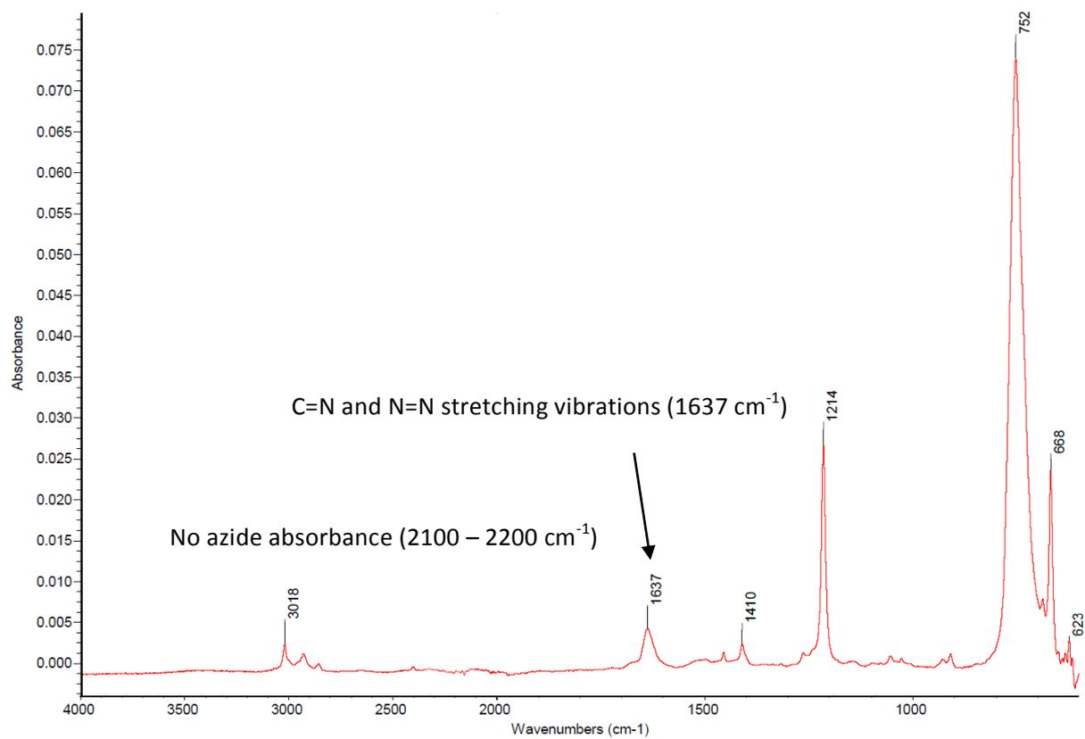
**Figure S18.** Infrared spectroscopy spectrum for **PY1** (in  $\text{CHCl}_3$ ) with peaks at  $3016\text{cm}^{-1}$  and  $752\text{cm}^{-1}$  attributed to the chloroform solvent.
