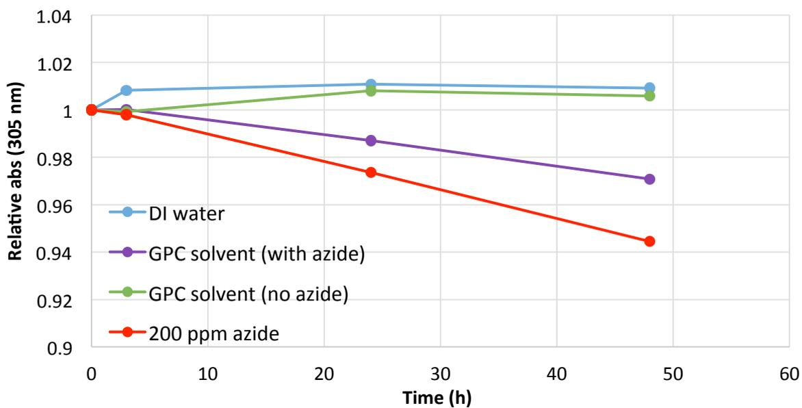
**Figure S1.** CTA loss of **7.4kBM1429** in different solvents monitored by UV-Vis absorbance at 305 nm ( $\lambda_{\text{max}}$  for trithiocarbonates).
