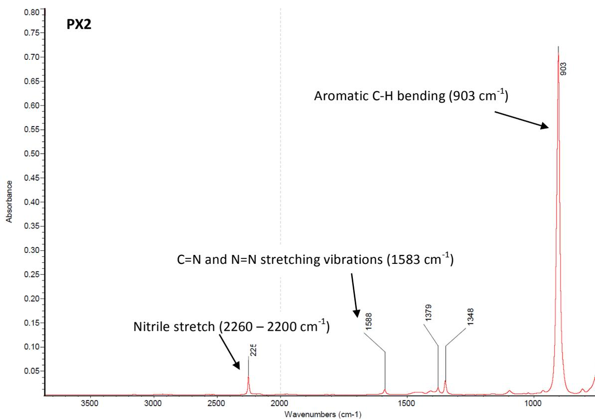
**Figure S16.** FTIR spectra for **PX1** (solid state) and **PX2** (in CDCl<sub>3</sub> with the CDCl<sub>3</sub> signal subtracted).
