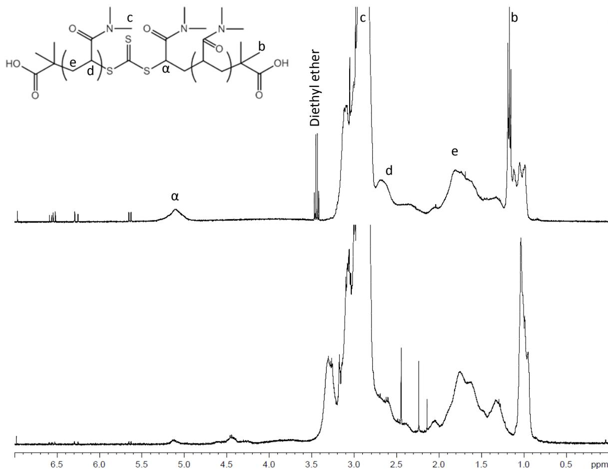
**Figure S7.** <sup>1</sup>H-NMR spectrum of **1.5kDMAT** polymer before (top, in CDCl<sub>3</sub>) and after treatment (bottom, in CDCl<sub>3</sub>) with 267 mM sodium azide solution. The α-carbon proton signal (broad, 5.1 ppm) is absent in the water soluble component after treatment with sodium azide, suggesting CTA removal.
