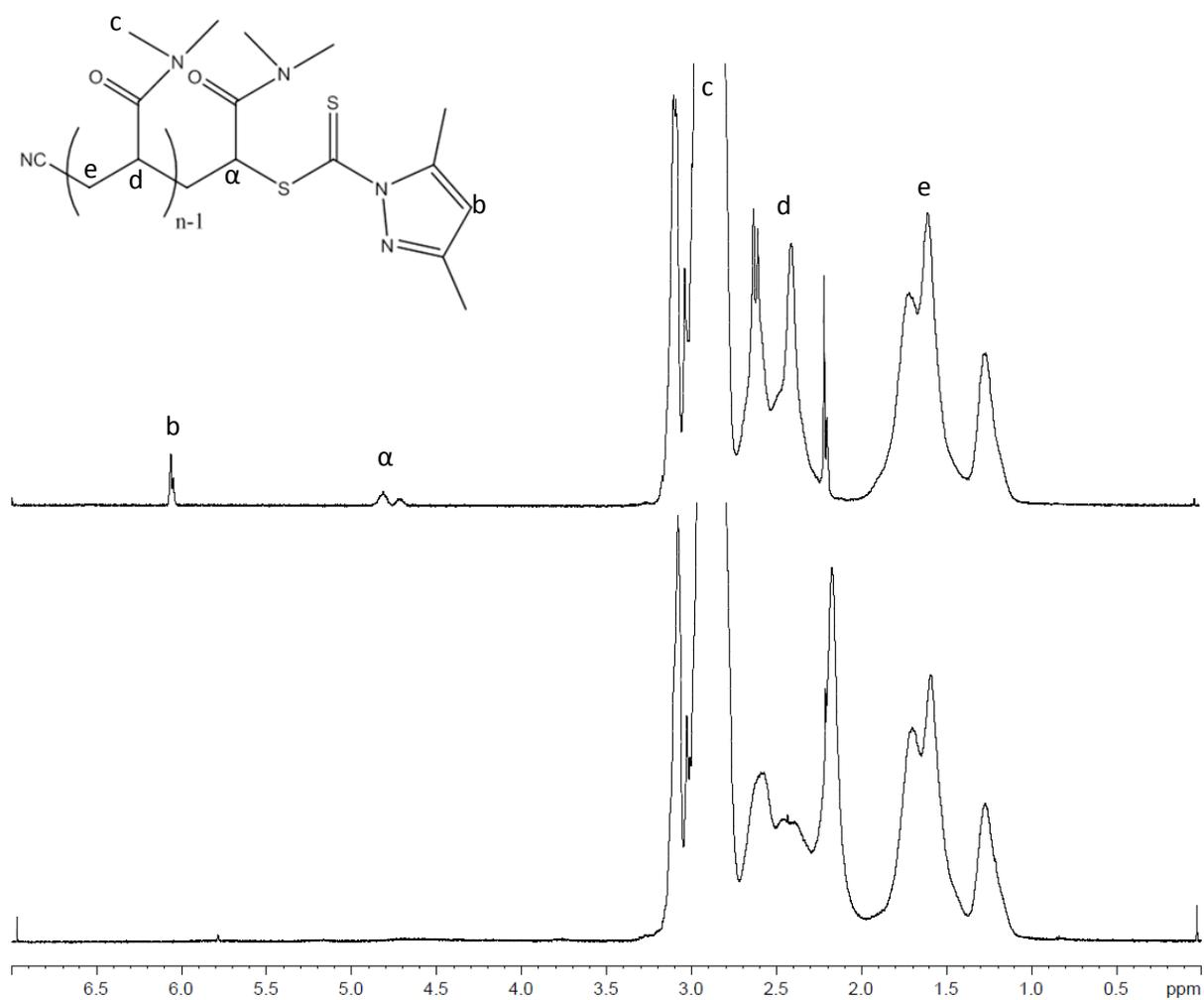
**Figure S6.**  $^1\text{H-NMR}$  spectrum of **4.6kCDMPC** polymer before (top, in  $\text{CDCl}_3$ ) and after treatment (bottom, in  $\text{CDCl}_3$ ) with 267 mM sodium azide solution. The  $\alpha$ -carbon proton signal (broad, 4.8 ppm) and pyrazole proton (d, 6.06 ppm) are absent in the water soluble component after treatment with sodium azide, suggesting CTA removal.
