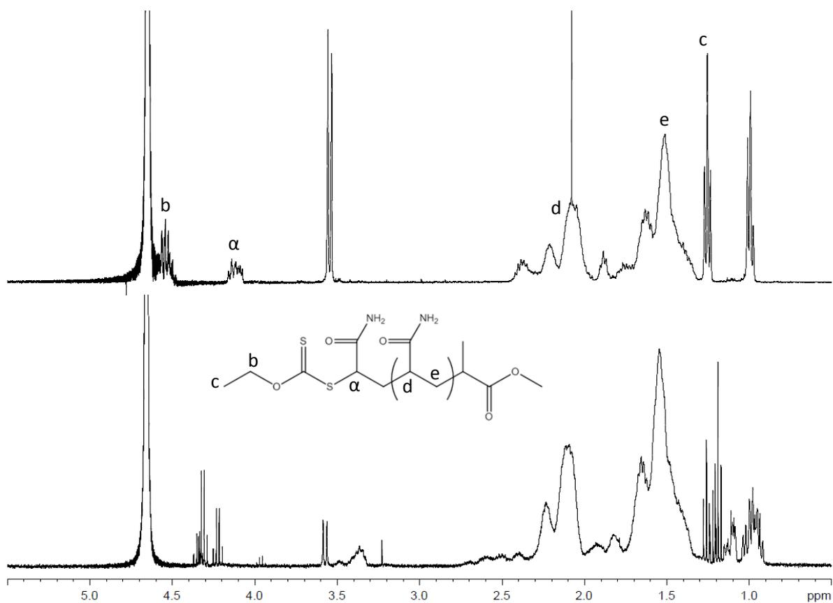
**Figure S8.** <sup>1</sup>H-NMR spectrum of **1kXA1** polymer before (top, in D<sub>2</sub>O) and after treatment (bottom, in D<sub>2</sub>O) with 267 mM sodium azide solution. The α-carbon proton signal (m, 4.1 ppm) is absent in the water soluble component after treatment with sodium azide, suggesting CTA removal.
