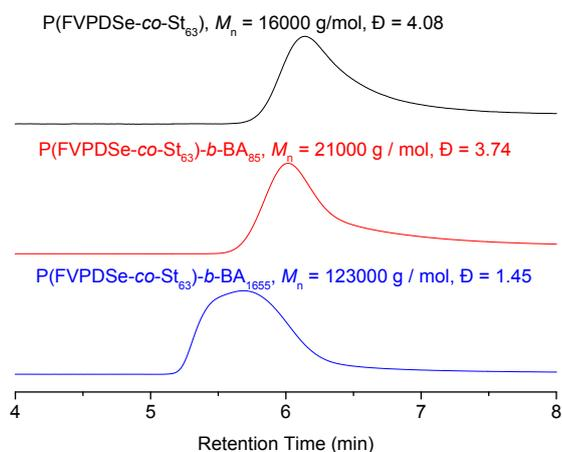
Figure S9 SEC curves of poly(FVPDSe-*co*-St) and poly(FVPDSe-*co*-St)-*b*-BA after oxidation by  $\text{H}_2\text{O}_2$ . Poly(FVPDSe-*co*-St) was prepared with an initial molar ratio  $[\text{St}]_0/[\text{FVPDSe}]_0$  of 100. Poly(FVPDSe-*co*-St)-*b*-BA was prepared with an initial molar ratio  $[\text{BA}]_0/[\text{Poly}(\text{FVPDSe-}co\text{-St})]_0$  of 500 and 2000.
