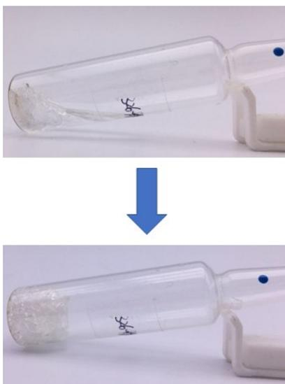
Figure S7 poly(FVPDSe-*co*-St) before and after chain extension in n-BA.
