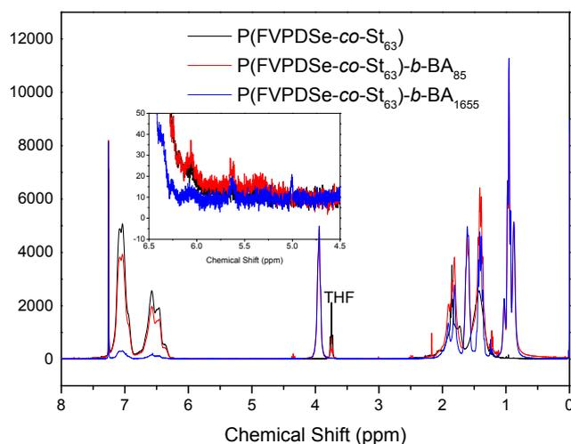
Figure S8  $^1\text{H}$  NMR spectra of poly(FVPDSe-*co*-St) and poly(FVPDSe-*co*-St)-*b*-BA after oxidation by  $\text{H}_2\text{O}_2$ . Poly(FVPDSe-*co*-St) was prepared with an initial molar ratio  $[\text{St}]_0/[\text{FVPDSe}]_0$  of 100. Poly(FVPDSe-*co*-St)-*b*-BA was prepared with an initial molar ratio  $[\text{BA}]_0/[\text{Poly}(\text{FVPDSe-}co\text{-St})]_0$  of 500 and 2000.
