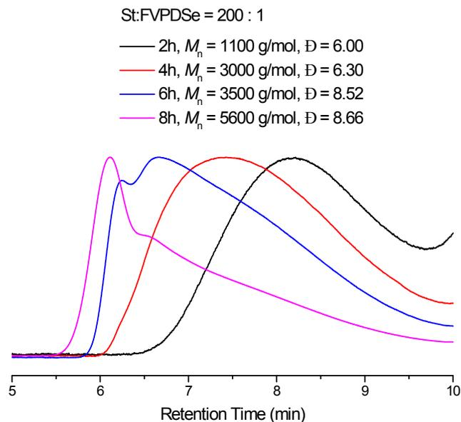
Figure S6 SEC curves of copolymers formed at low monomer conversion before gelation. Experimental condition:  $[St]_0/[FVPDSe]_0 = 40, 100, \text{ and } 200$ .  $[St]_0 = 8.0$  M, in toluene- $d_8$  at  $50^\circ\text{C}$ , linear polystyrene standards were used for THF SEC calibration.
