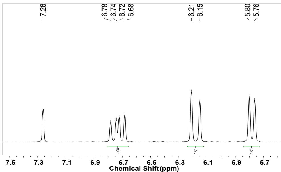
Figure S1.  $^1\text{H}$  NMR spectrum of FVPDSe in  $\text{CDCl}_3$ .
