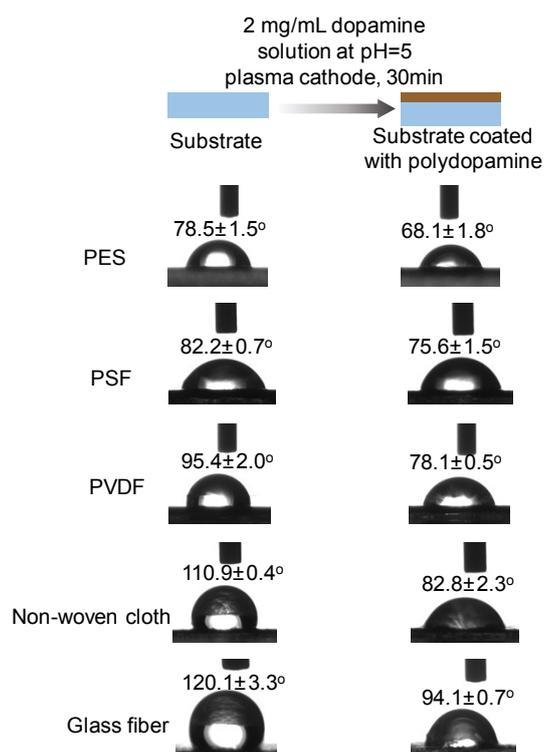
**Fig. S4** The water contact angles before and after the deposition of PDA coating on various substrates. PES: polyether sulfone, PSF: polysulfone, PVDF: polyvinylidene fluoride.
