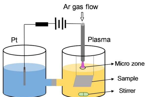
**Fig. S5** Scheme of the “H” type reactor in the preparation of PDA with microplasma method.
