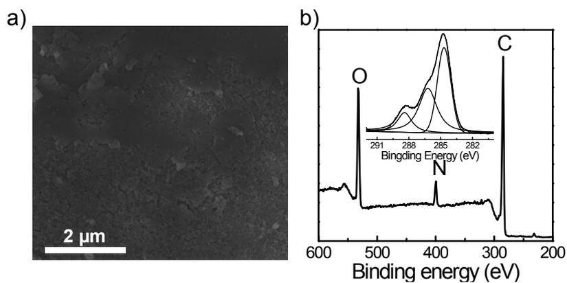
**Fig. S3** (a) SEM image and (b) XPS analysis of PDA coated on silicon wafer.
