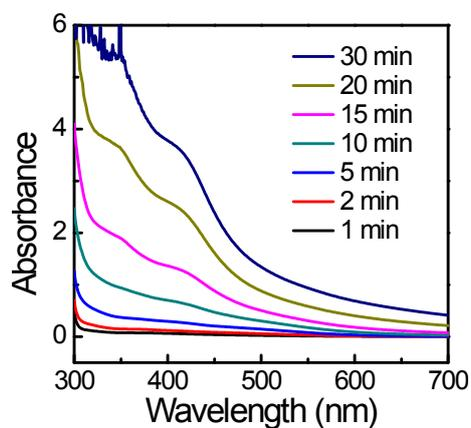
**Fig. S1** UV-Vis spectra of PDA treated by microplasma cathode for different time.
