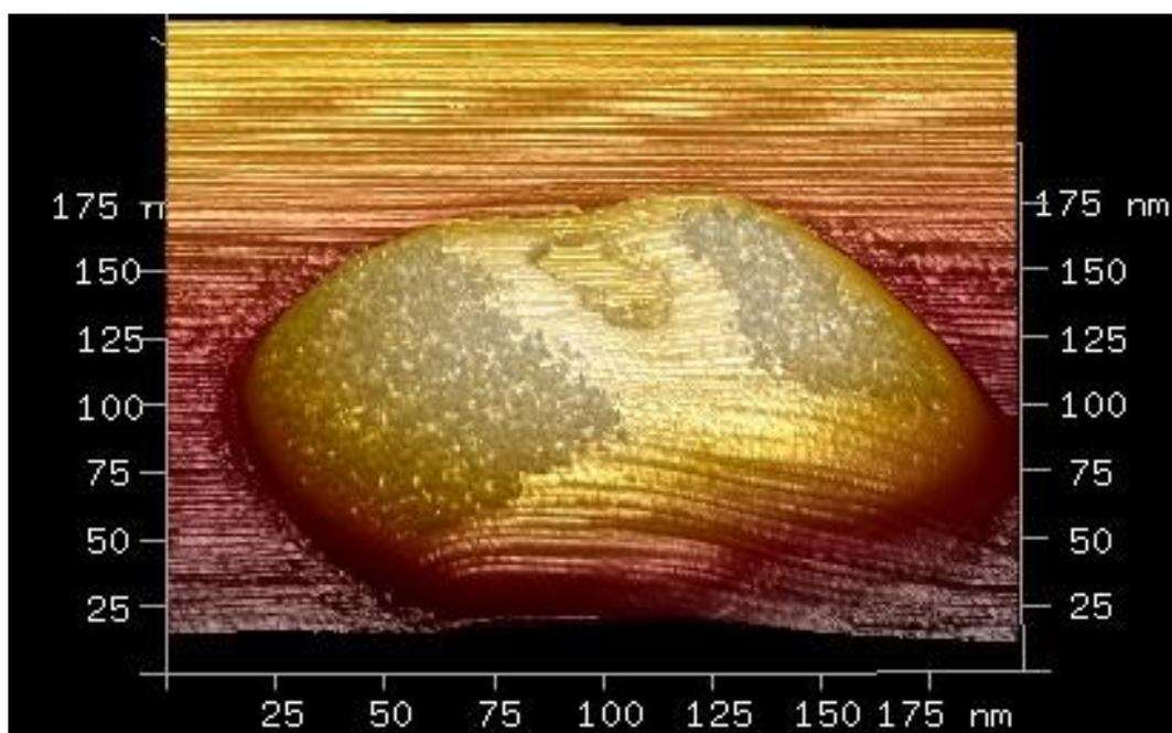
**Figure S11.** Characteristic AFM image of a single vesicle (before CO<sub>2</sub> purging).
