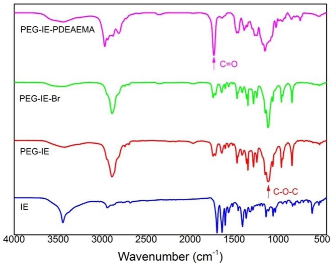
**Figure S6.** FTIR spectra of the synthesized polymers. The appearance of peak at around  $2900\text{ cm}^{-1}$  ( $\nu_{\text{C-H}}$  of ether) and the  $1120\text{ cm}^{-1}$  ( $\nu_{\text{C-O-C}}$ ) in the spectrum of PEG-IE demonstrates the successful addition of PEG segment to the chromophore, while the strong peak at  $1740\text{ cm}^{-1}$  ( $\nu_{\text{C=O}}$ ) in the spectrum of PEG-IE-PDEAEMA shows the successful growth of PDEAEMA chain on the other side of the chromophore.
