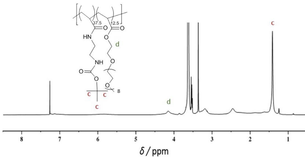
**Figure S4.**  $^1\text{H}$  NMR spectra of Boc-protected macroRAFT agent in  $\text{CDCl}_3$ .
