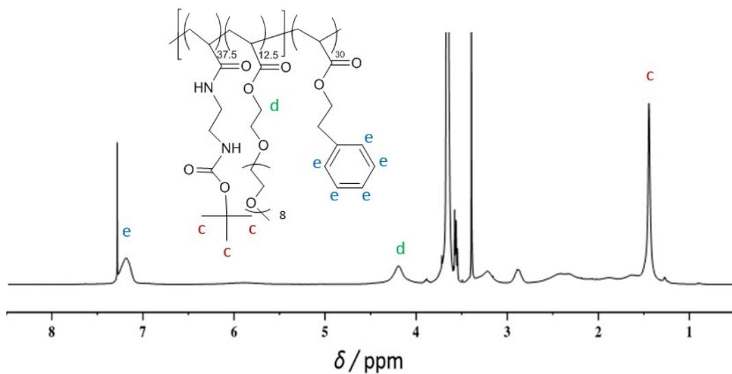
**Figure S6.**  $^1\text{H}$  NMR spectra of Boc-protected block copolymer B2 in  $\text{CDCl}_3$ .
