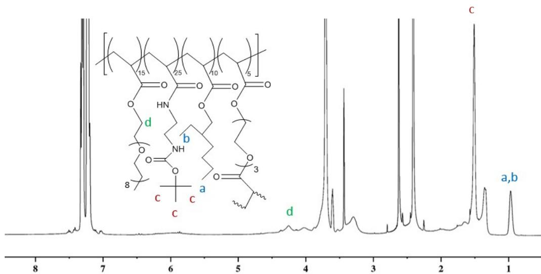
**Figure S8.** <sup>1</sup>H NMR spectra of Boc-protected hyperbranched polymer H2 in CDCl<sub>3</sub>.
