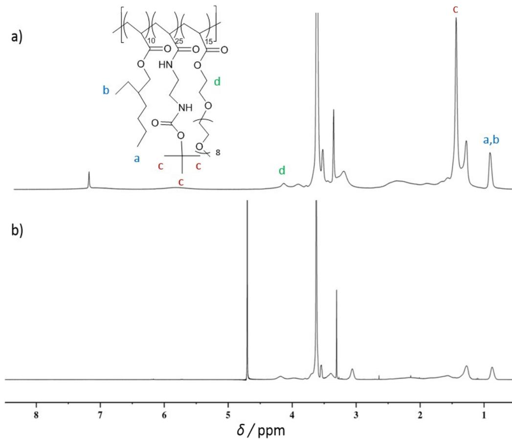
**Figure S2.**  $^1\text{H}$  NMR spectra of Boc-protected linear random copolymer L2 in  $\text{CDCl}_3$  (a) and the corresponding Boc-deprotected L2 in  $\text{D}_2\text{O}$  (b).
