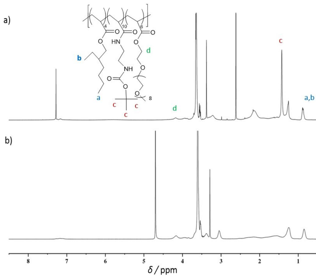
**Figure S3.**  $^1\text{H}$  NMR spectra of Boc-protected linear random copolymer L3 in  $\text{CDCl}_3$  (a) and the corresponding Boc-deprotected L3 in  $\text{D}_2\text{O}$  (b).
