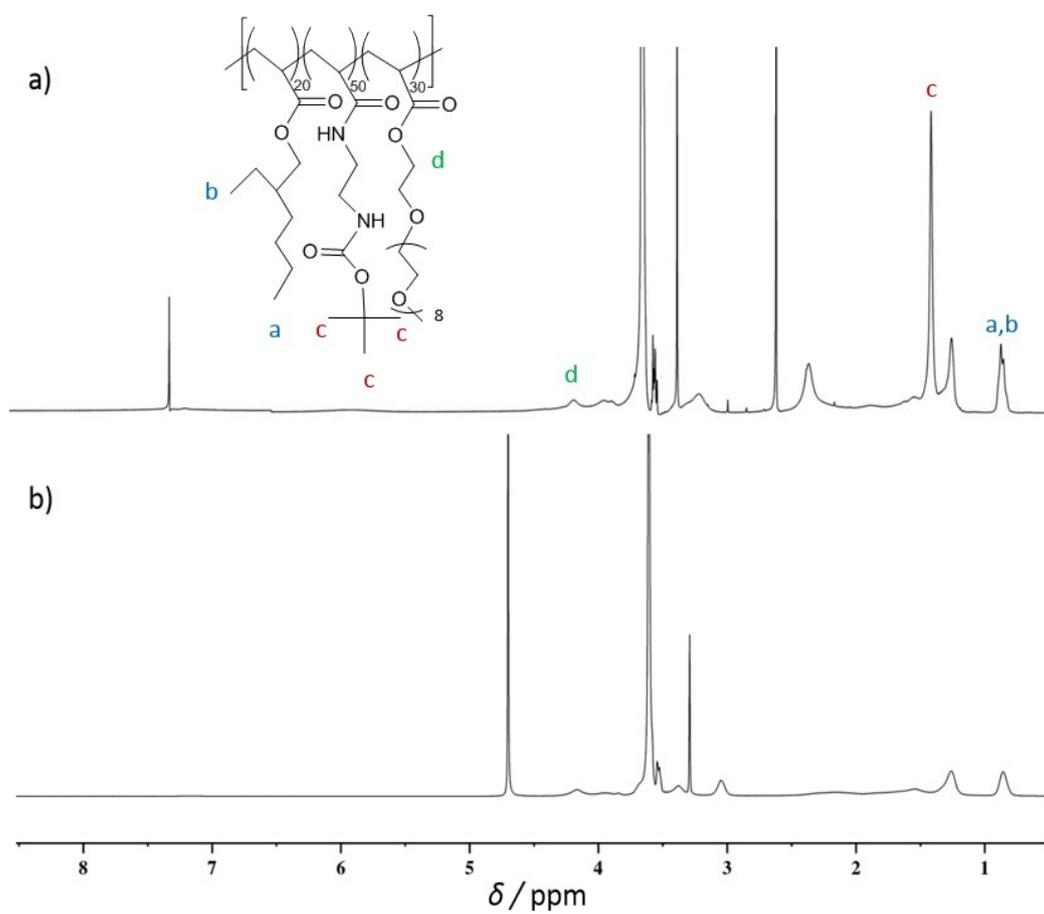
**Figure S1.**  $^1\text{H}$  NMR spectra of Boc-protected linear random copolymer L1 in  $\text{CDCl}_3$  (a) and the corresponding Boc-deprotected L1 in  $\text{D}_2\text{O}$  (b).
