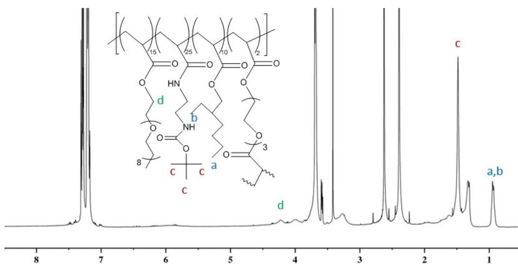
**Figure S7.**  $^1\text{H}$  NMR spectra of Boc-protected hyperbranched polymer H1 in  $\text{CDCl}_3$ .
