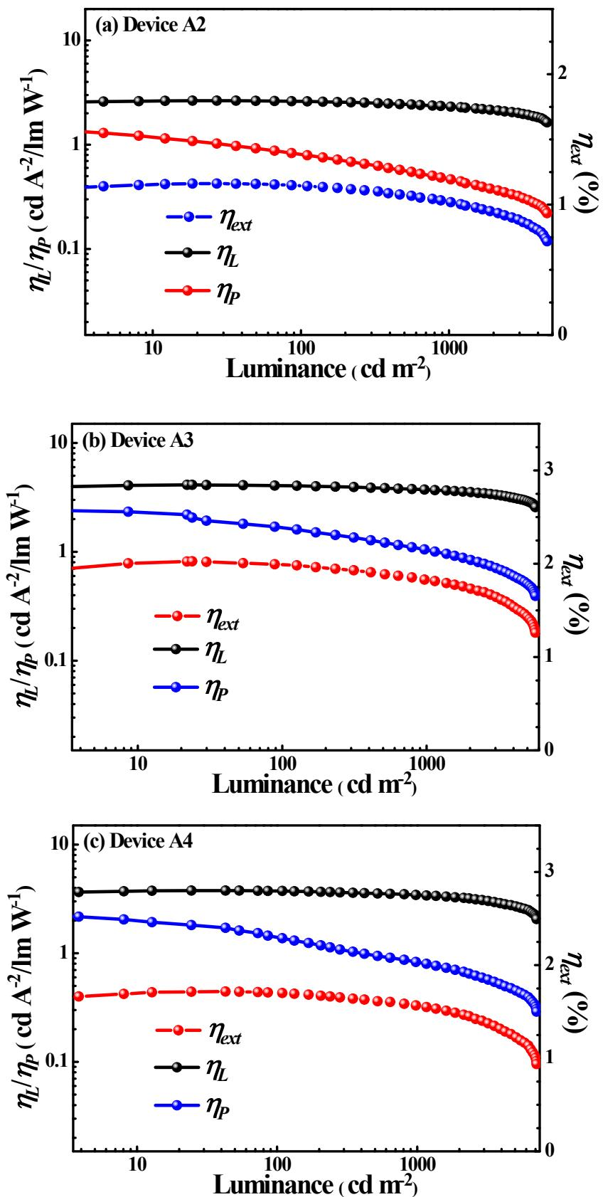
**Fig. S15** Relationship between EL efficiencies and luminance for devices A2, A3 and A4.
