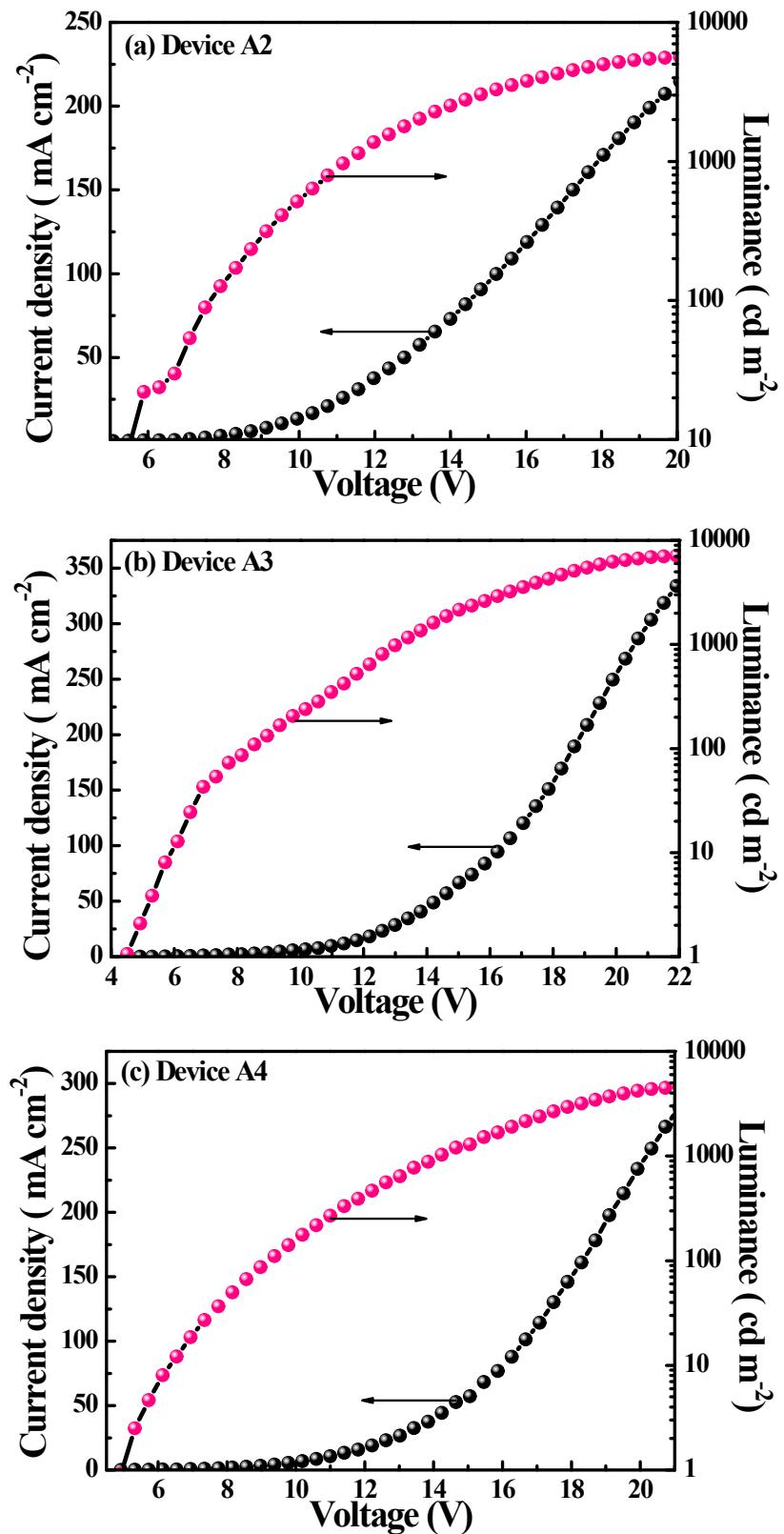
**Fig. S14**  $J$ - $V$ - $L$  curves for the devices A2, A3 and A4.
