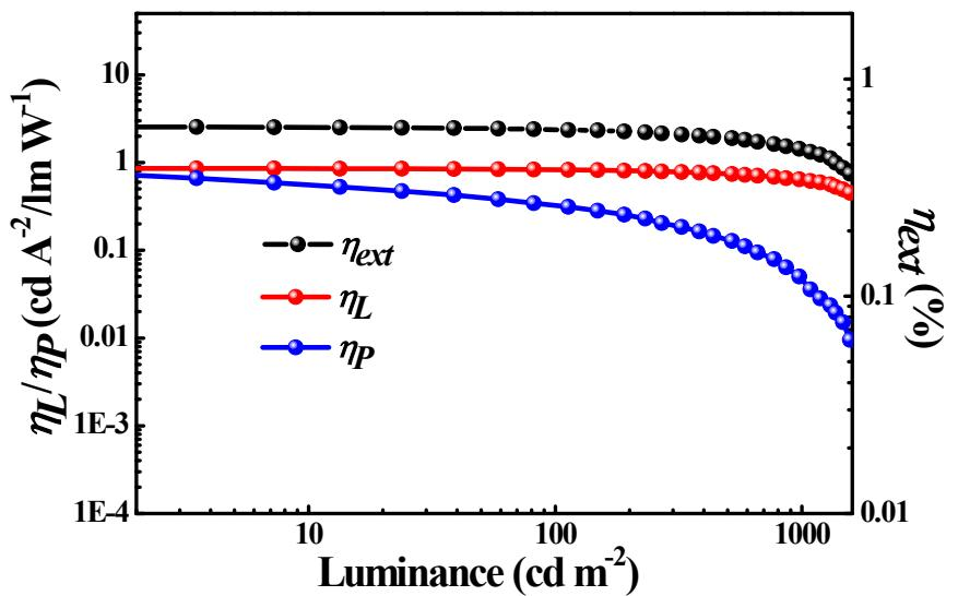
**Fig. S16** Relationship between EL efficiencies and luminance for OLED based on **Zn-C**.
