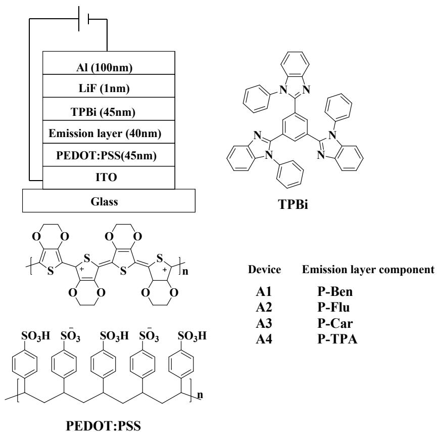
**Fig. S13** Configuration of the PLEDs made from these *bis*-Zn<sup>II</sup> salphen coordination polymers and the chemical structures of the functional materials involved.
