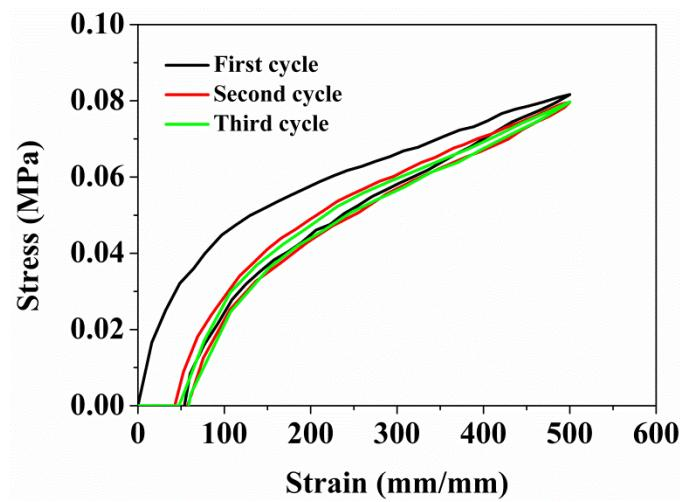
**Fig. S3** Three consecutive loading-unloading cycles curves without any lapse time between the cycles of PEA<sub>P-A</sub>-10%-PAAm hydrogel.
