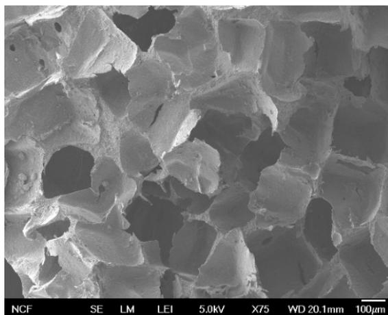
5 **Figure S1:** SEM image of the CuAAC foam. The scan was performed with acceleration voltage
