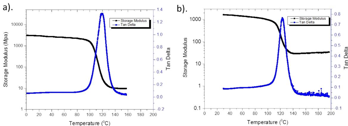
22 **Figure S3:** Glass transition temperature,  $T_g$ , and storage modulus of a CuAAC non-foam
