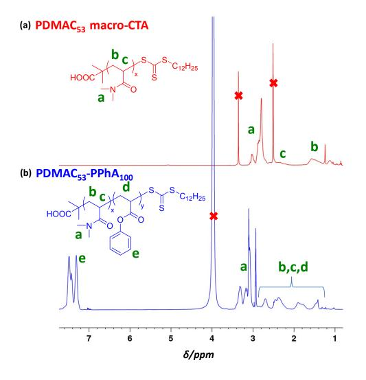
**Figure S1**. <sup>1</sup>H NMR spectra recorded for (a) PDMAC<sub>53</sub> macro-CTA in DMSO-d<sub>6</sub> and (b) PDMAC<sub>53</sub>-PPhA<sub>100</sub> diblock copolymer in DMF-d<sub>7</sub> (>99% PhA conversion after polymerization for 4.5 h in water at 30 °C; DDMAT/initiator molar ratio = 5.0).
