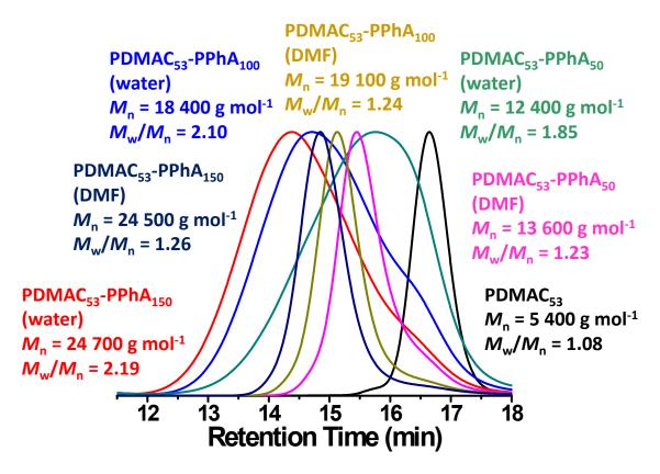
**Figure S4**. DMF GPC curves for PDMAC<sub>53</sub>–PPhA<sub>x</sub> diblock copolymers prepared at 25% w/w solids and 30 °C via either RAFT aqueous emulsion polymerization or solution polymerization in DMF.  $M_n$  values are expressed relative to a series of near-monodisperse poly(methyl methacrylate) calibration standards. All reactions reached high conversion (>96 %) as judged by <sup>1</sup>H NMR in DMF-d<sub>7</sub>.
