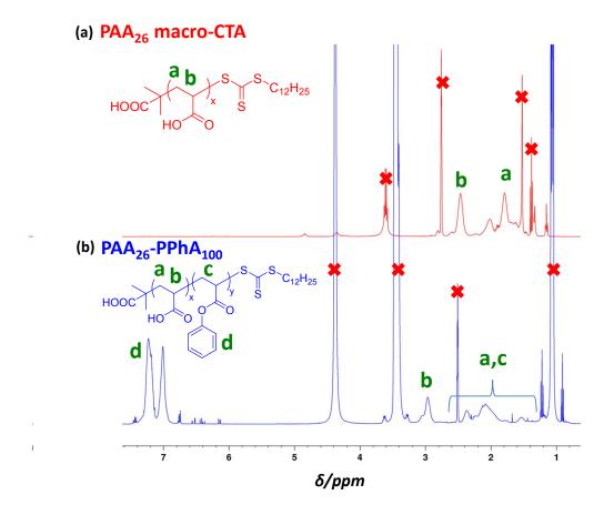
**Figure S2**. <sup>1</sup>H NMR spectra in DMSO-d<sub>6</sub> recorded for (a) PAA<sub>26</sub> macro-CTA and (b) PAA<sub>26</sub>-PPhA<sub>80</sub> diblock copolymer (98% PhA conversion after polymerization in ethanol for 16 h at 70 °C; DDMAT/initiator molar ratio = 5.0).
