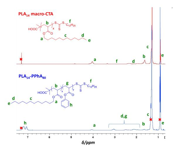
**Figure S3**. <sup>1</sup>H NMR spectra recorded in CDCl<sub>3</sub> for (a) PLA<sub>14</sub> macro-CTA and (b) PLA<sub>14</sub>-PPhA<sub>100</sub> diblock copolymer (>99% % PhA conversion after polymerization in *n*-heptane for 16 h at 80 °C; CTA/initiator molar ratio = 5.0).
