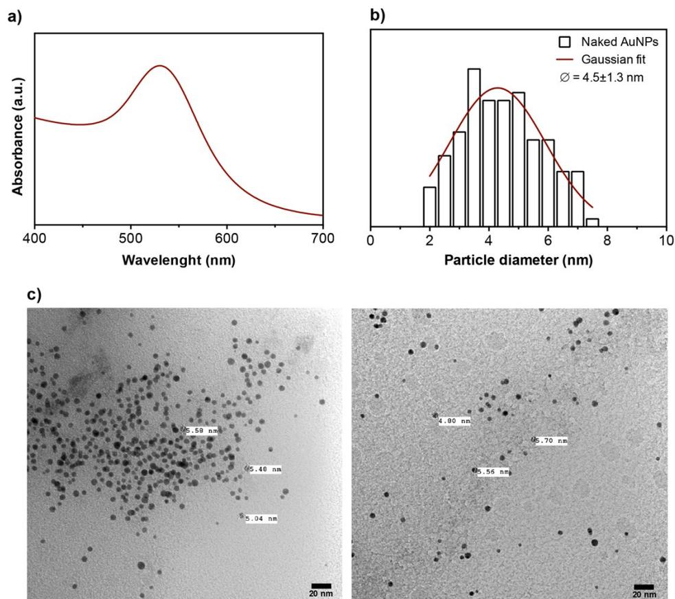
**Fig. S3** (a) UV/Vis spectrum of the as prepared AuNPs in aqueous solution. (b) Size distribution histogram derived by measuring the diameter of 100 nanoparticles. (c) TEM microphotographs of PVP-coated AuNPs (scale bars = 20 nm).
