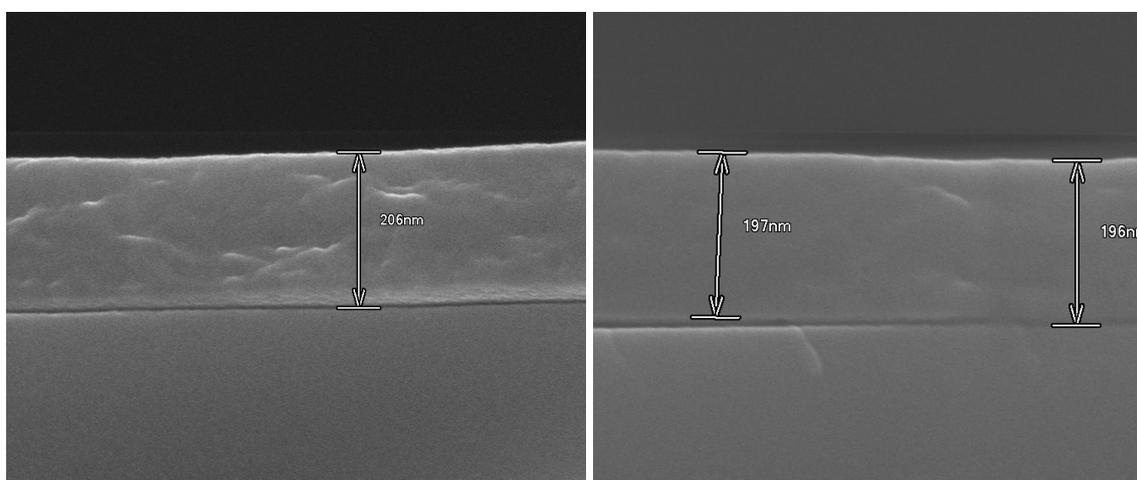
**Fig. S4** SEM images of the section plane of cured **P1** film (left) and PPE film (right) on wafers for the measurement of dielectric strength.
