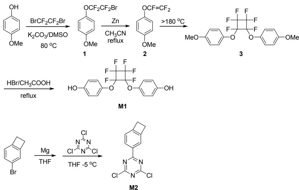
**Scheme S1.** Procedure for the synthesis of monomers **M1** and **M2**.
