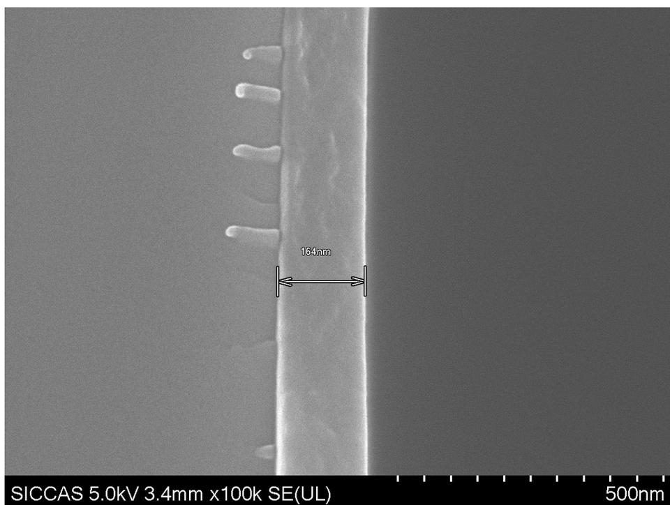
**Fig. S3** SEM image of the section plane of cured **P1** film on wafer for the measurement of dielectric constants and dissipation factors.
