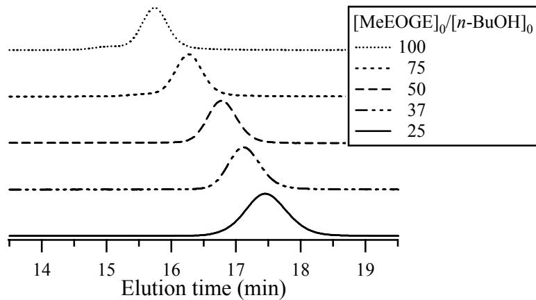
**Figure S3.** SEC traces of poly(MeEOGE)s with various molecular weight (eluent, THF; flow rate,  $1.0 \text{ mL min}^{-1}$ ).
