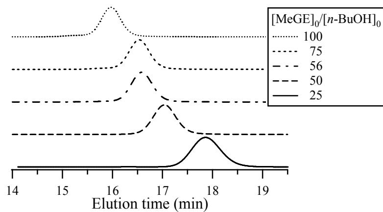
**Figure S1.** SEC traces of poly(MeGE)s with various molecular weights (eluent, THF; flow rate, 1.0 mL min<sup>-1</sup>).
