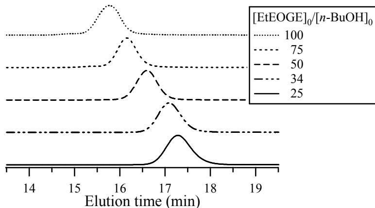
**Figure S4.** SEC traces of poly(EtEOGE)s with various molecular weights (eluent, THF; flow rate,  $1.0 \text{ mL min}^{-1}$ ).
