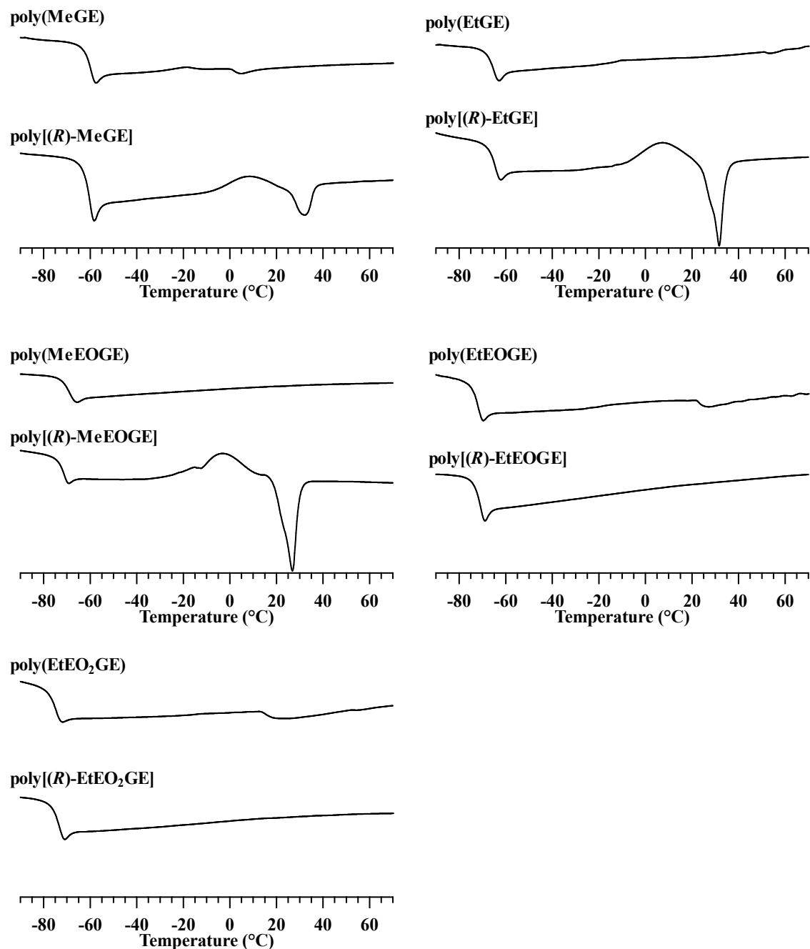
**Figure S19.** DSC thermograms of atactic and isotactic poly(MeGE)s, poly(EtGE)s, poly(MeEOGE)s, poly(EtEOGE)s, and poly(EtEO<sub>2</sub>GE)s during the second heating (heating rate of  $10\text{ }^{\circ}\text{C min}^{-1}$ ).
