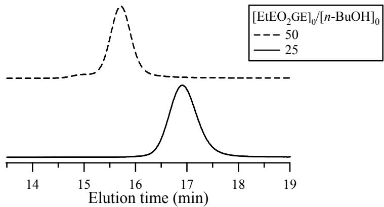
**Figure S5.** SEC traces of poly(EtEO<sub>2</sub>GE)s with various molecular weights (eluent, THF; flow rate, 1.0 mL min<sup>-1</sup>).
