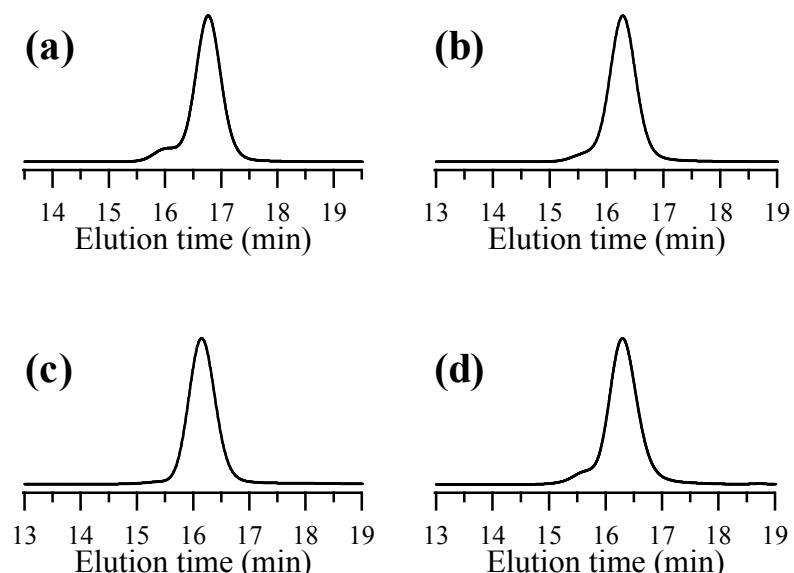
**Figure S6.** SEC traces of (a) poly(*i*PrGE)<sub>6k</sub>, (b) poly(PrEOGE)<sub>10k</sub>, (c) poly(MeEO<sub>2</sub>GE)<sub>9k</sub>, and (d) poly(MeEO<sub>3</sub>GE)<sub>8k</sub> (eluent, THF; flow rate, 1.0 mL min<sup>-1</sup>).
