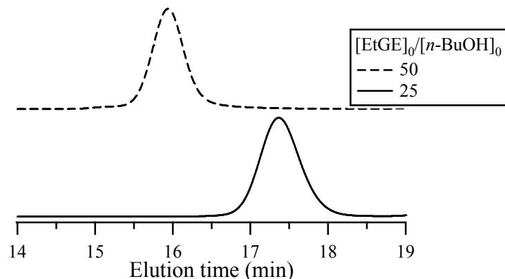
**Figure S2.** SEC traces of poly(EtGE)s with various molecular weights (eluent, THF; flow rate, 1.0 mL min<sup>-1</sup>).
