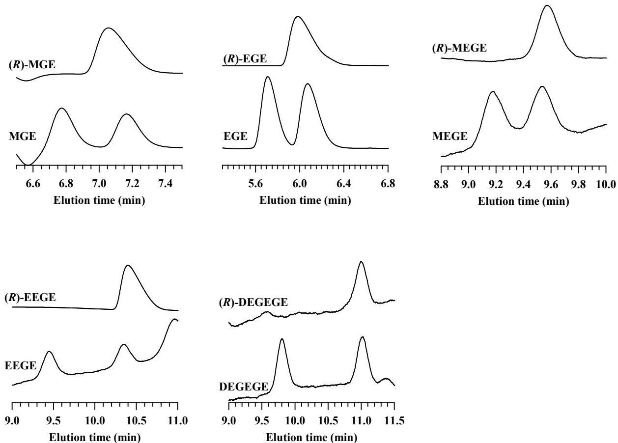
**Figure S12.** Chiral HPLC chromatograms of racemic and optically pure glycidyl ethers (column, CHIRALPAK IC; mobile phase, *n*-hexane/ethanol = 95/5 v/v; flow rate, 1.0  $\text{mL min}^{-1}$ ).
