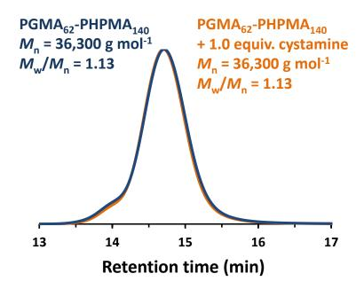
**Figure S3.** DMF GPC chromatograms obtained for PGMA<sub>62</sub>-PHPMA<sub>140</sub>, and PGMA<sub>62</sub>-PHPMA<sub>140</sub> + cystamine at 10 % w/w, after stirring for 24 h at 22 °C (equivalent to cystamine/epoxide molar ratio = 1.0 for P(GMA<sub>65</sub>-stat-GlyMA<sub>1.7</sub>)-HPMA<sub>140</sub>), as a control experiment.
