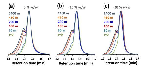
**Figure S4.** DMF GPC chromatograms for cystamine functionalization of P(GMA<sub>65</sub>-stat-GlyMA<sub>1.7</sub>)-PHPMA<sub>140</sub> worm gel ([cystamine]/[epoxide] = 0.50) at (a) 5 % w/w, (b) 10 % w/w, and (c) 20 % w/w solids, stirred for 24 h at 22 °C.
