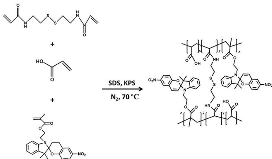
**Figure S1.** Synthetic route of SP-based nanogels.
