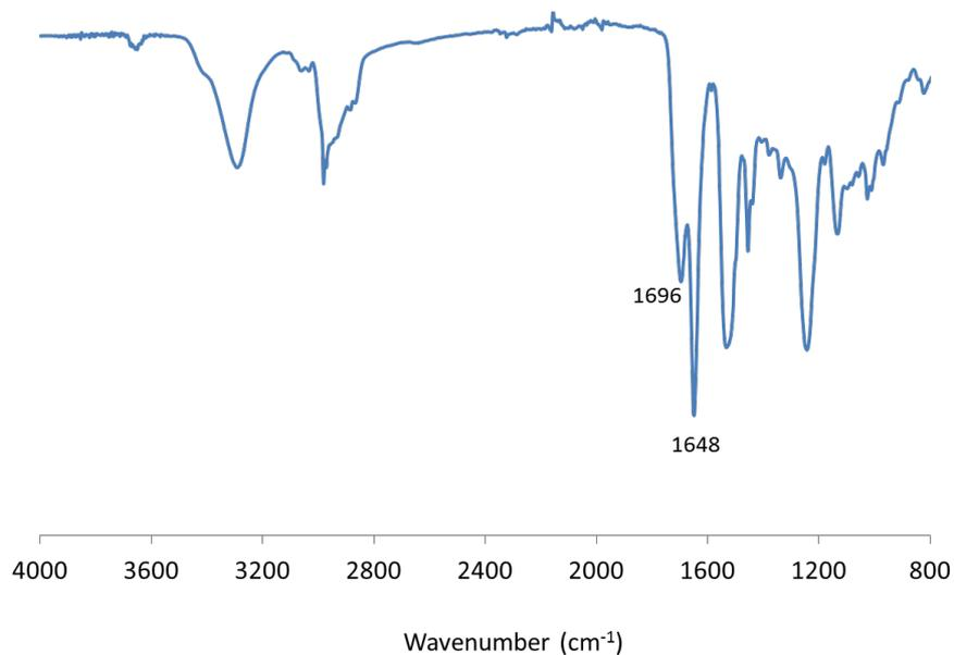
Figure S4. FTIR spectrum of P1.
