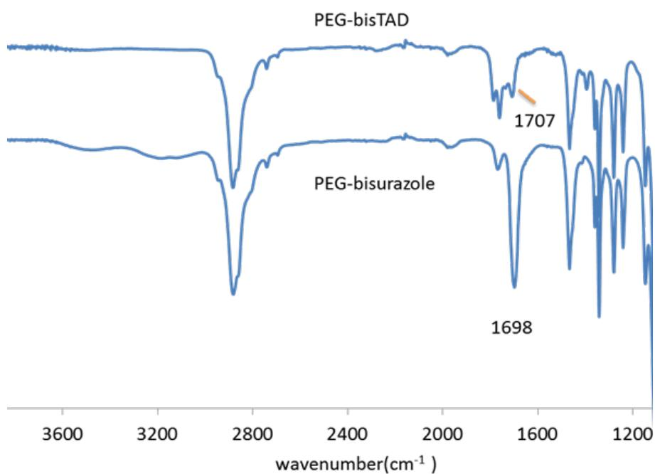
**Figure S8.** FTIR spectrum of PEG2K-bisurazole and PEG2K-bisTAD.
