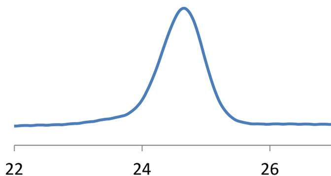
**Figure S7.** HFIP-SEC trace of PEG2K-bisurazole.  $M_w$ : 14,300 g/mol, PDI: 1.1
