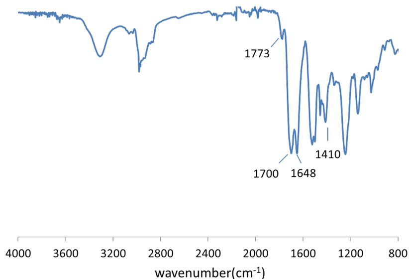
**Figure S10.** FTIR spectrum of PTAD functionalized P1.
