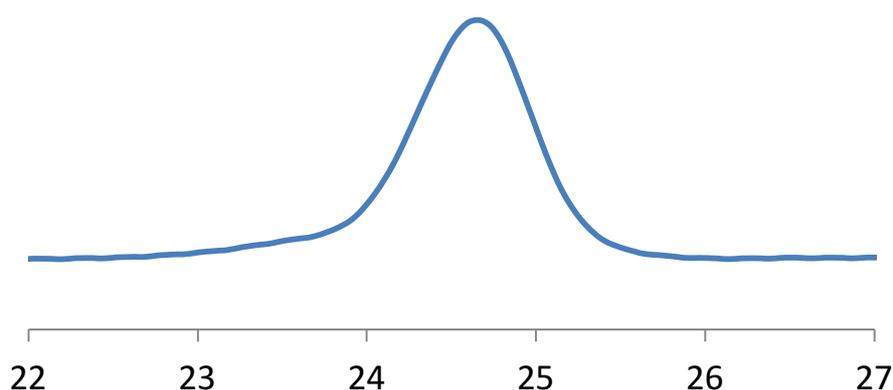
**Figure S6.** HFIP-SEC trace of PEG2K-hydrazine carboxylate.  $M_w$ : 14,300 g/mol, PDI: 1.1
