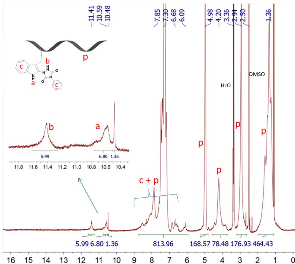
Figure S9.  $^1\text{H-NMR}$  spectrum of PTAD functionalized P1.
