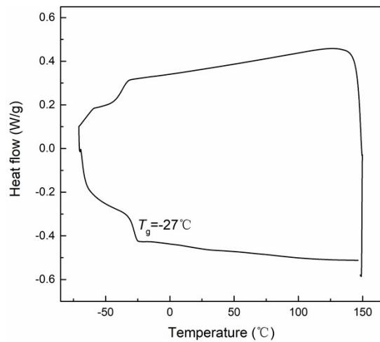
**Fig. S13** DSC curve of a FGE homopolymer prepared by  $i\text{-Bu}_3\text{Al}/\text{H}_3\text{PO}_4/\text{DBU}$  (Table 1, run 9).
