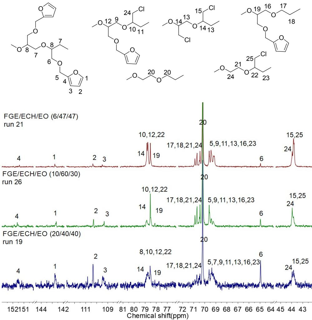
**Fig. S5** <sup>13</sup>C-NMR spectra (100 MHz, C<sub>2</sub>D<sub>2</sub>Cl<sub>4</sub>, r.t.) of FGE/ECH/EO terpolymers with different composites prepared by *i*-Bu<sub>3</sub>Al/H<sub>3</sub>PO<sub>4</sub>/DBU (Table 1, runs 19, 21, 26).
