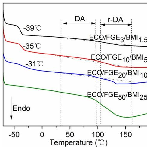
**Fig. S21** Thermal changes of DA cross-linked polyepichlorohydrin elastomers in DA and retro-DA process.
