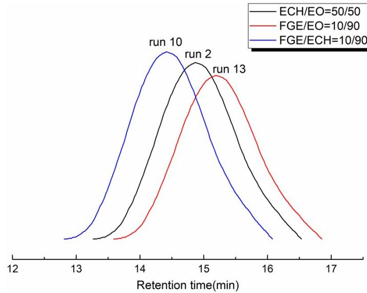
**Fig. S18** GPC curves of a FGE/ECH copolymer, a FGE/EO copolymer and a ECH/EO copolymer prepared by *i*-Bu<sub>3</sub>Al/H<sub>3</sub>PO<sub>4</sub>/DBU (Table 1, runs 2, 10, 13).
