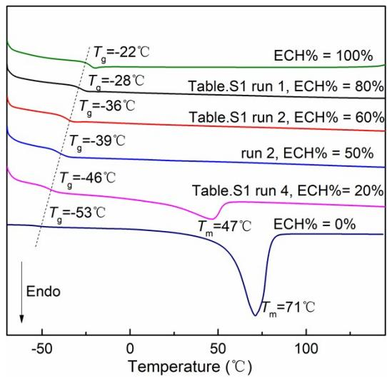
**Fig. S12** DSC curves of ECH/EO copolymers with different ECH contents prepared by  $i\text{-Bu}_3\text{Al}/\text{H}_3\text{PO}_4/\text{DBU}$  (Table 1, runs 2, Table.S1 run 1, 2, 4).
