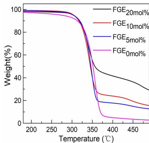
**Fig. S23** TGA curves of DA cross-linked polyepichlorohydrin elastomers with different FGE contents.
