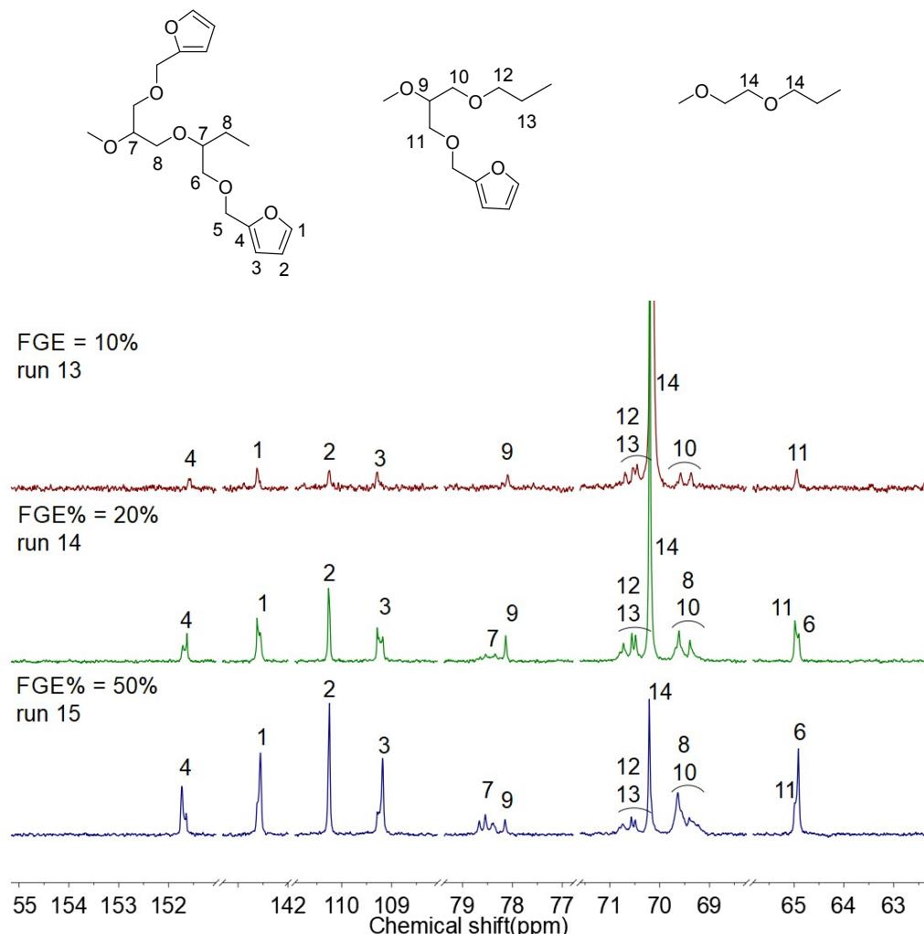
**Fig. S3** <sup>13</sup>C-NMR spectra (100 MHz, C<sub>2</sub>D<sub>2</sub>Cl<sub>4</sub>, r.t.) of FGE/EO copolymers with different FGE contents prepared by *i*-Bu<sub>3</sub>Al/H<sub>3</sub>PO<sub>4</sub>/DBU (Table 1, runs 13–15).
