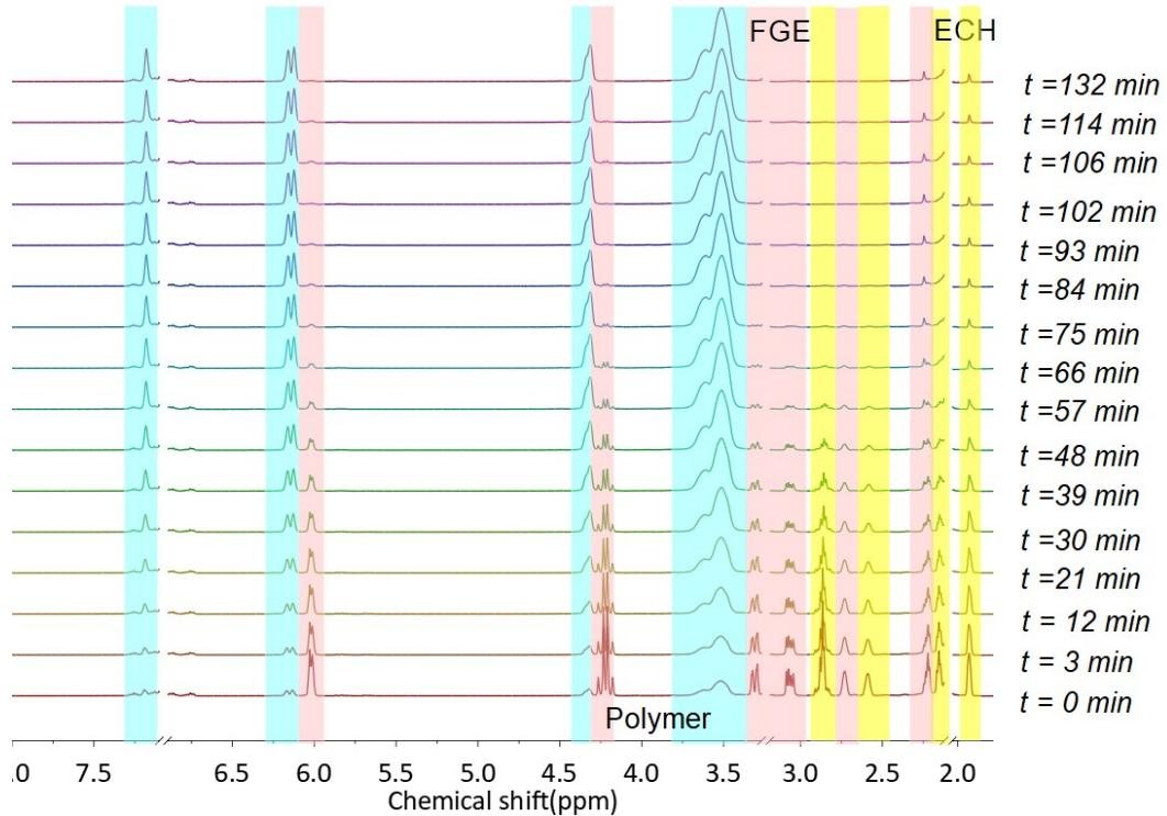
**Fig. S8**  $^1\text{H}$ -NMR spectra (500 MHz, toluene-d<sub>8</sub>, 25°C) of the copolymerization ECH and FGE. FGE resonances are shaded in pink, and ECH resonances are shaded in yellow. Resonances associated with the copolymer are shaded in blue.
