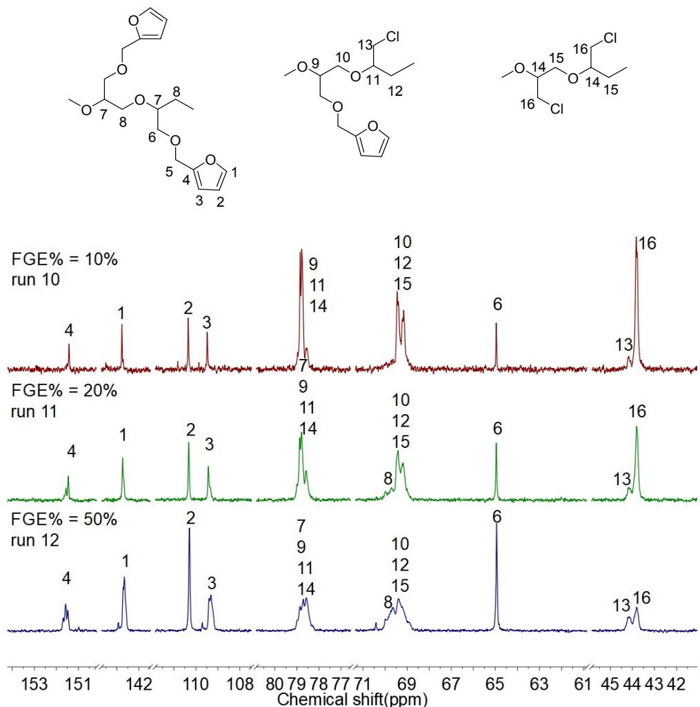
**Fig. S4**  $^{13}\text{C}$ -NMR spectra (100 MHz,  $\text{C}_2\text{D}_2\text{Cl}_4$ , r.t.) of FGE/ECH copolymers with different FGE contents prepared by *i*- $\text{Bu}_3\text{Al}/\text{H}_3\text{PO}_4/\text{DBU}$  (Table 1, runs 10–12).
