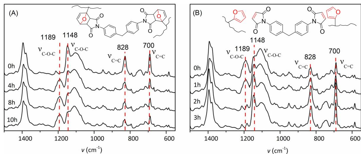
**Fig. S11** FT-IR spectra of a ECO/FGE<sub>20</sub>/BMI<sub>10</sub> terpolymer in the procedure of DA cross-linking (A) at 70 °C and retrocross-linking (B) at 150 °C.
