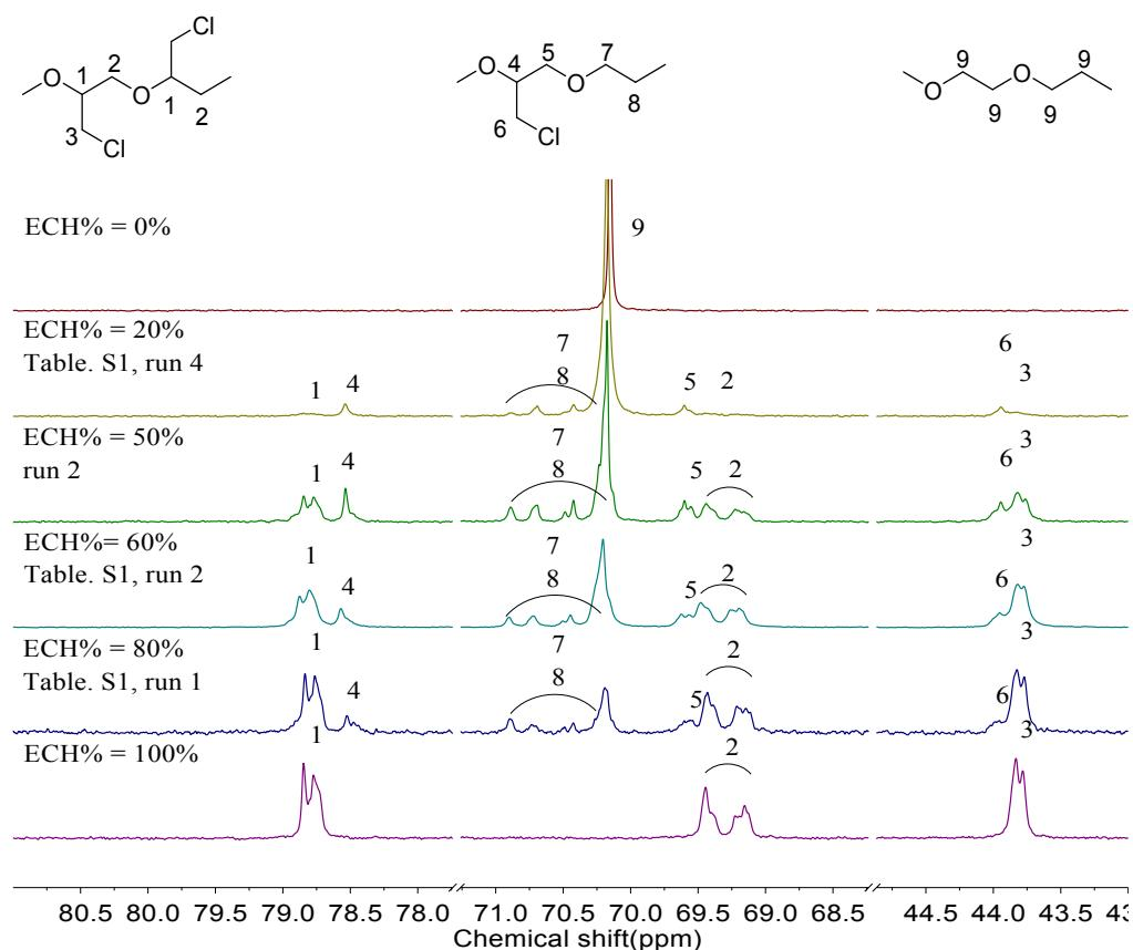
**Fig. S1** <sup>13</sup>C-NMR spectra (100 MHz, C<sub>2</sub>D<sub>2</sub>Cl<sub>4</sub>, r.t.) of a EO homopolymer, a ECH homopolymer and ECH/EO copolymers having different ECH contents prepared by *i*-Bu<sub>3</sub>Al/H<sub>3</sub>PO<sub>4</sub>/DBU (Table 1, run 2, Table. S1, runs 1, 2, 4).
