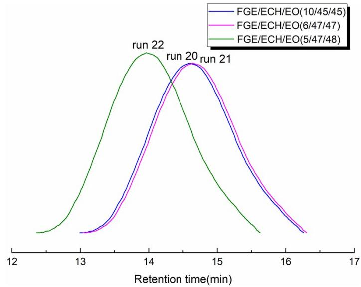
**Fig. S19** GPC curves of FGE/ECH/EO terpolymers prepared by *i*-Bu<sub>3</sub>Al/H<sub>3</sub>PO<sub>4</sub>/DBU (Table 1, runs 20–22).
