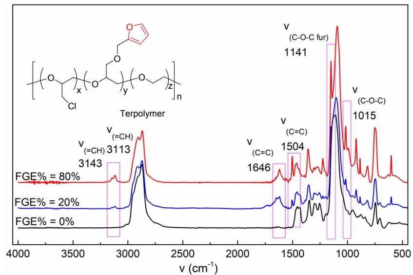
**Fig. S10** FT-IR spectra of FGE/ECH/EO terpolymers with different FGE contents prepared by  $i\text{-Bu}_3\text{Al}/\text{H}_3\text{PO}_4/\text{DBU}$ .
