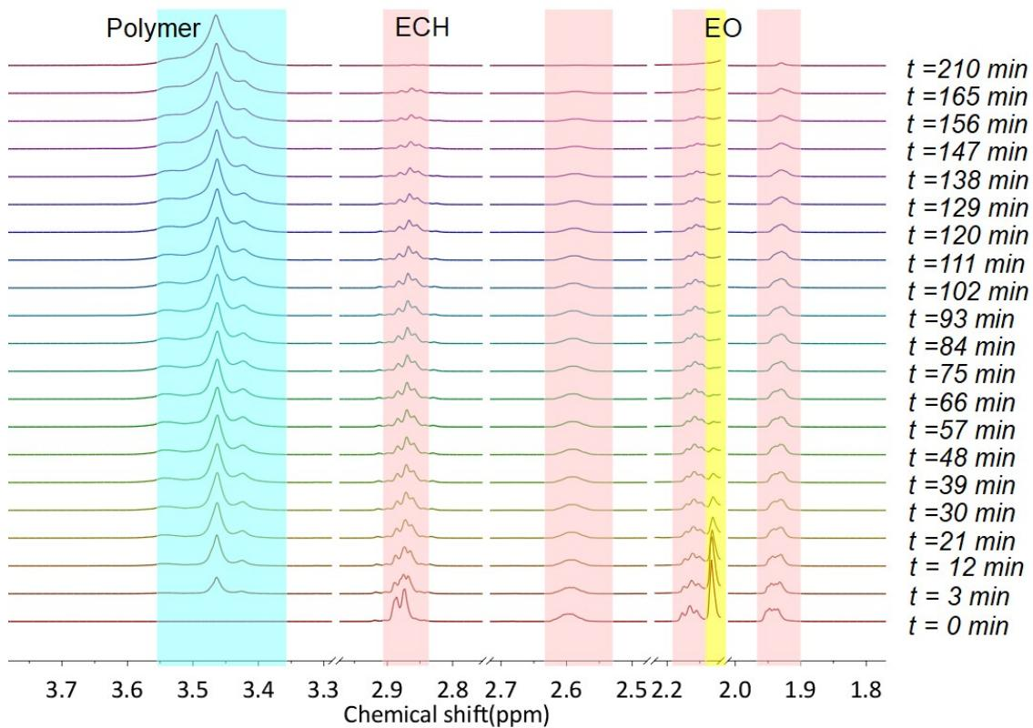
**Fig. S6**  $^1\text{H}$ -NMR spectra (500 MHz, toluene-d<sub>8</sub>, 25°C) of the copolymerization ECH and EO. ECH resonances are shaded in pink, and EO resonances are shaded in yellow. Resonances associated with the copolymer are shaded in blue.
