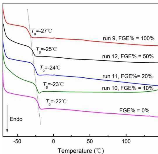
**Fig. S15** DSC curves of FGE/ECH copolymers with different FGE contents prepared by  $i\text{-Bu}_3\text{Al}/\text{H}_3\text{PO}_4/\text{DBU}$  (Table 1, runs 9–12).
