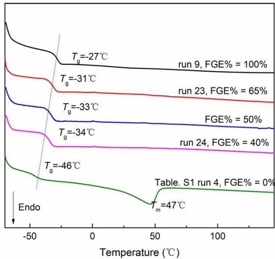
**Fig. S17** DSC curves of FGE/ECH/EO terpolymers with different FGE contents (mole ratio of ECH/EO is 1/4) prepared by *i*-Bu<sub>3</sub>Al/H<sub>3</sub>PO<sub>4</sub>/DBU (Table 1, runs 9, 23, 24, Table. S1, run 4).
