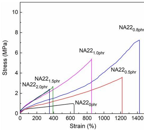
**Fig. S24** Stress-strain curves of Vulcanized\_ECO/NA22<sub>n</sub> materials verify different crosslinked agents NA22.
