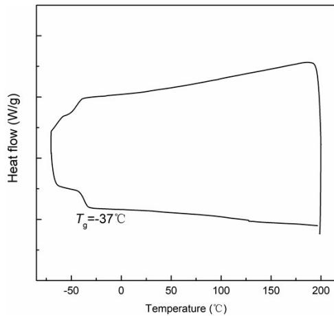
**Fig. S22** DSC curve of DA cross-linked polyepichlorohydrin elastomers (DA\_ECO/FGE<sub>5</sub>/BMI<sub>2.5</sub>).
