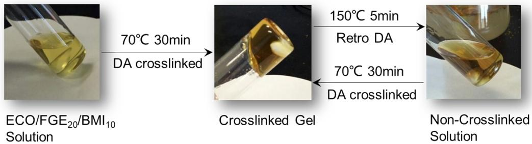
**Fig. S20** Solubility evolution of ECO/FGE<sub>20</sub> after DA and retro-DA process in CHCl<sub>2</sub>CHCl<sub>2</sub> (20 mg polymer/mL).
