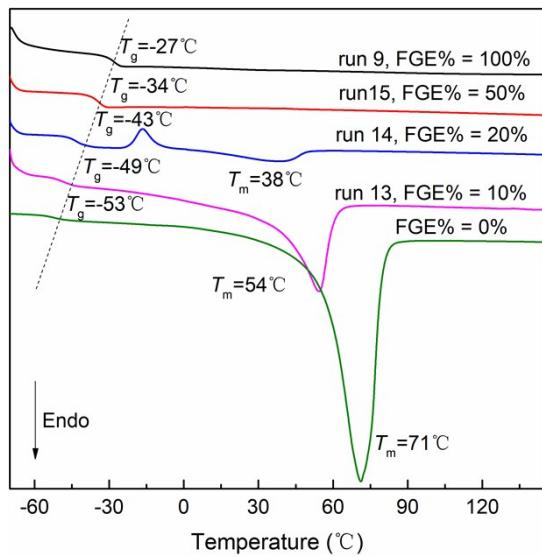
**Fig. S14** DSC curves of FGE/EO copolymers with different FGE contents prepared by  $i\text{-Bu}_3\text{Al}/\text{H}_3\text{PO}_4/\text{DBU}$  (Table 1, runs 9, 13–15).
