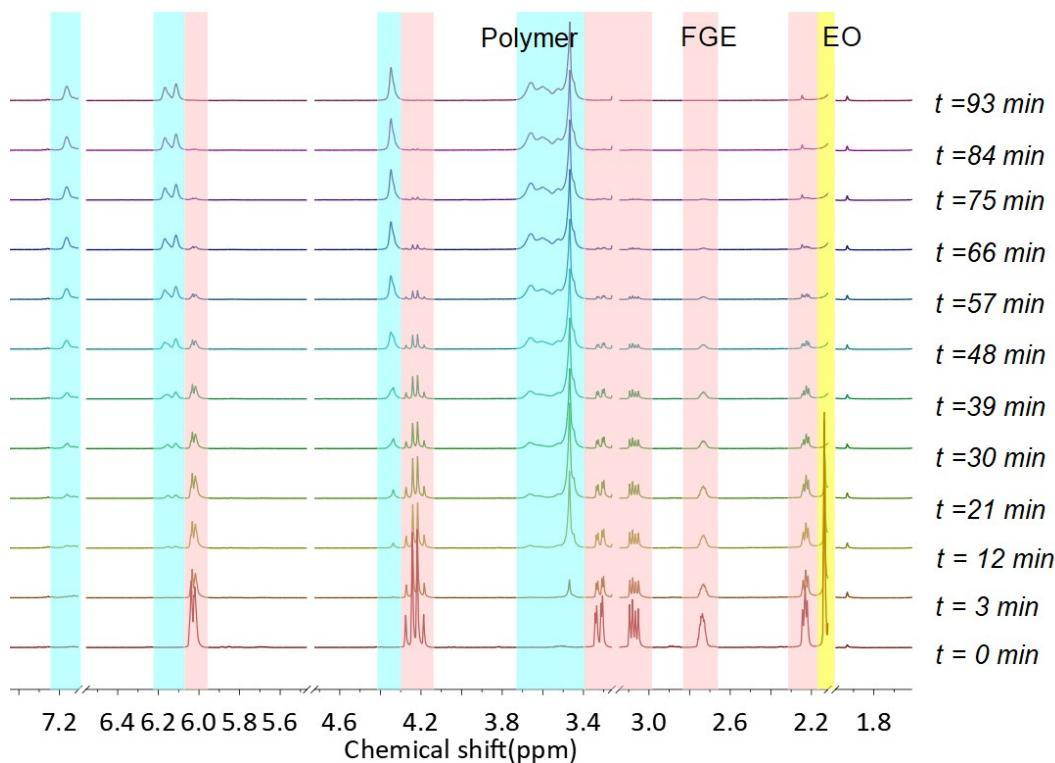
**Fig. S7**  $^1\text{H}$ -NMR spectra (500 MHz, toluene-d<sub>8</sub>, 25°C) of the copolymerization EO and FGE. FGE resonances are shaded in pink, and EO resonances are shaded in yellow. Resonances associated with the copolymer are shaded in blue.
