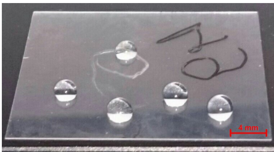
Figure S52. Water droplets (4 \mu l) on a poly(TFMST- co -ST) copolymer surface.
