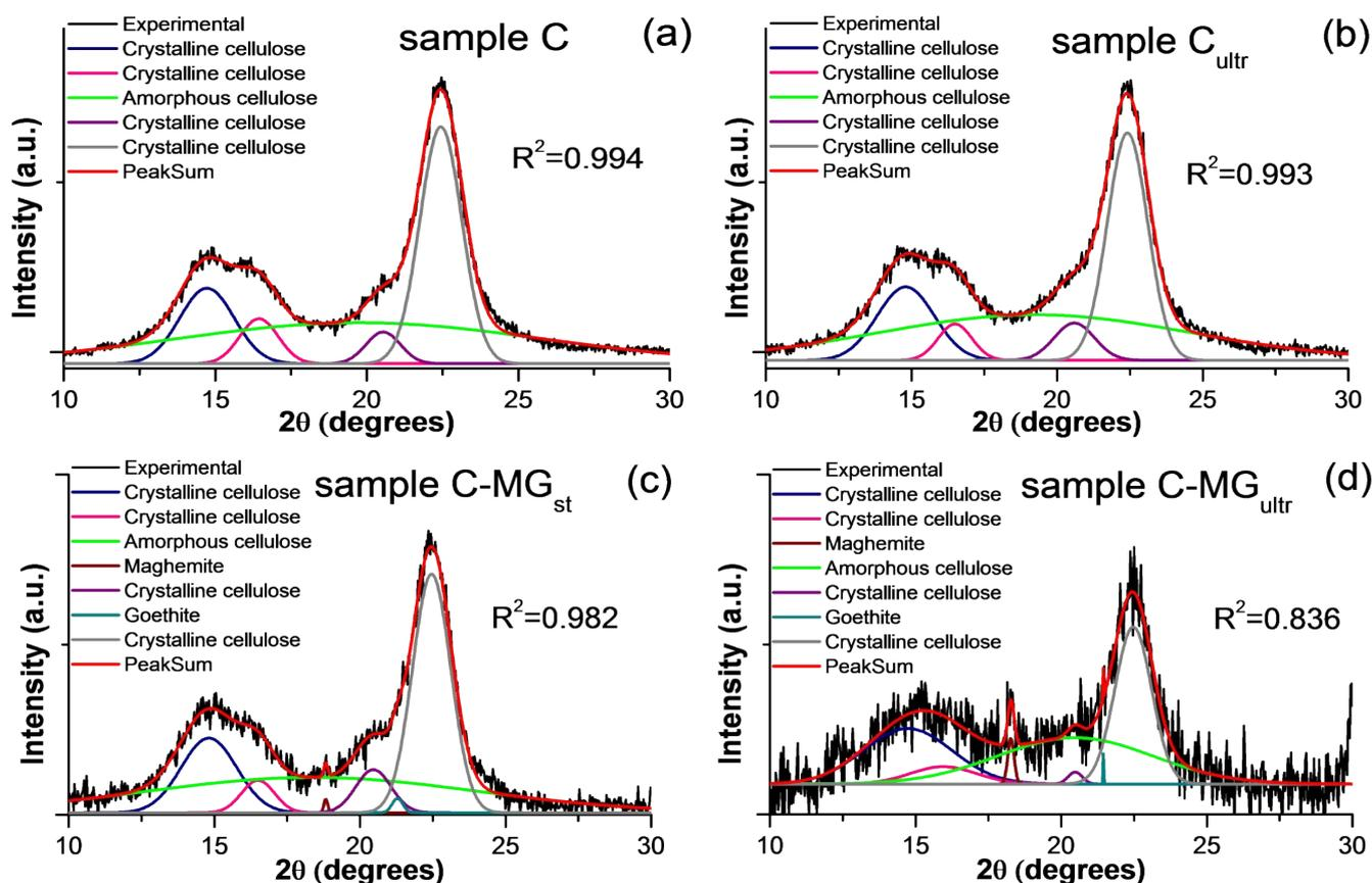
Fig. S1. Deconvolution of XRD patterns for (a) pristine cellulose: C, (b) cellulose ultrasonicated: C<sub>ultr</sub>, and composites obtained by (c) stirring: C-MG<sub>st</sub> and (d) ultrasonication: C-MG<sub>ultr</sub>.
