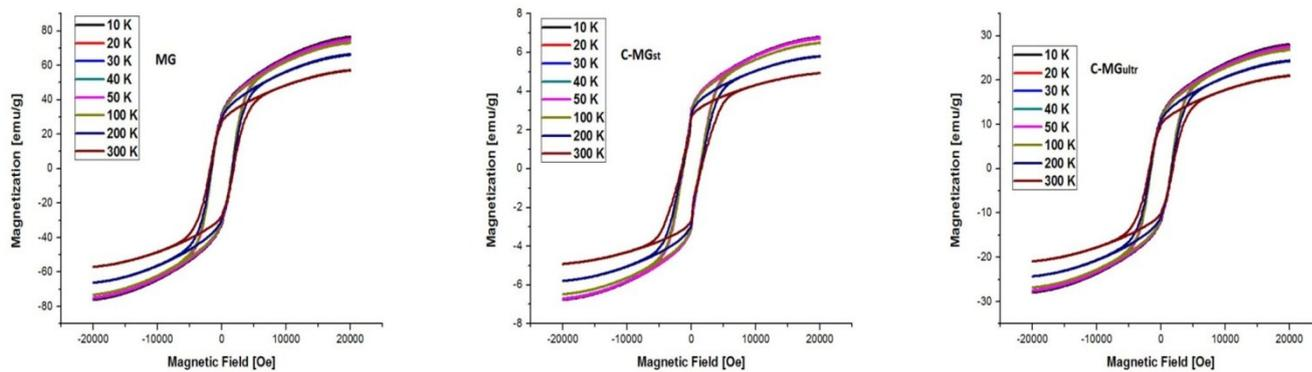
Fig. S4. Magnetization curve for MG, C-MGst and C-MGultr.
