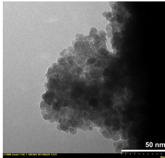
Fig. S3. TEM images of MG nanoparticles (a) and of C-MGst and C-MGultr samples (b) at different magnifications.
