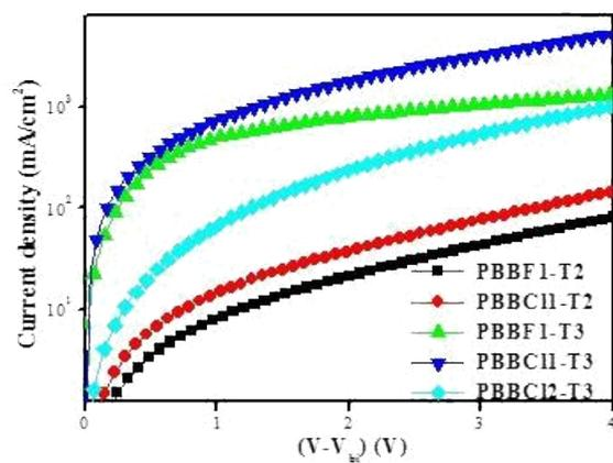
**Figure S4.** The  $J$ - $V$  curves of hole-only **PBBF1-T2**, **PBBC11-T2**, **PBBF1-T3**, **PBBC11-T3** and **PBBC12-T3**:PC<sub>71</sub>BM blend films in dark.
