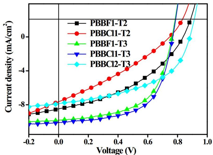
**Figure S3.**  $J$ - $V$  curves of the PSCs devices without DIO as an additive under  $100 \text{ mW cm}^{-2}$  AM 1.5 G irradiation.
