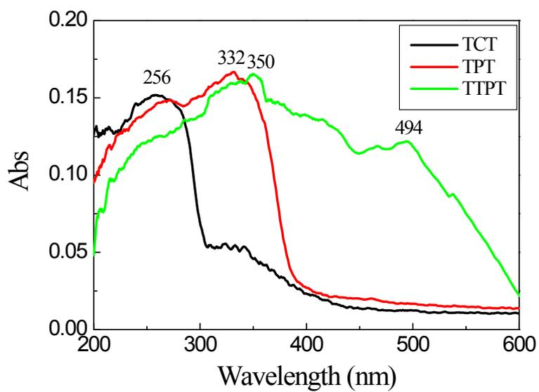
Fig. S2. Solid-State UV-VIS spectra of TTPT, TCT and TPT.
