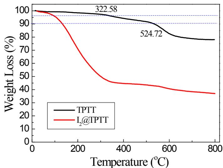
Fig. S5. TGA curves for TTPT and I<sub>2</sub>@TTPT with a heating rate of 10 °C·min<sup>-1</sup> in N<sub>2</sub>.
