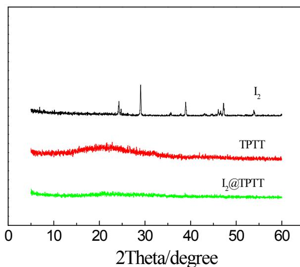
Fig. S4. X-ray powder diffraction patterns of  $\text{I}_2$ , TTPT and  $\text{I}_2$ @TTPT.
