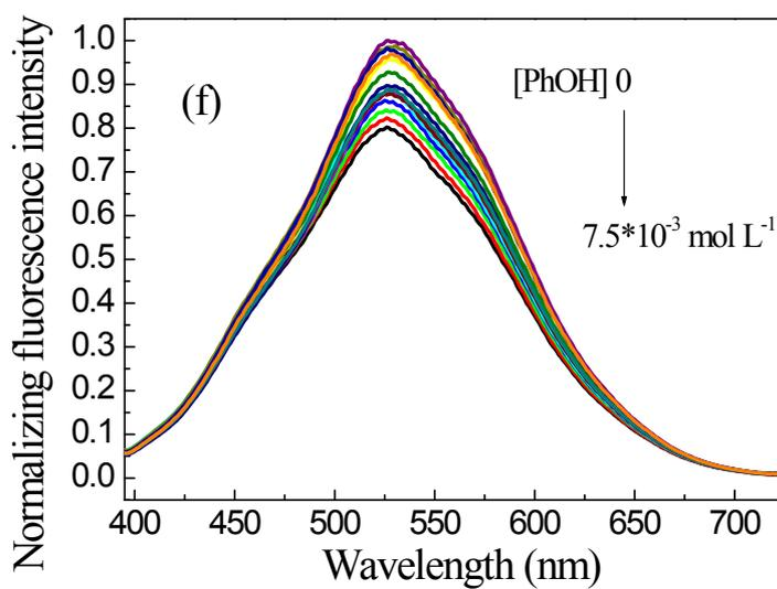
Fig. S7. Fluorescence spectra of the TTPT measured in dispersions of THF (1.0 mg mL<sup>-1</sup>, excited at 370 nm). (a) DNT, (b) DCIB, (c) NB, (d) NT, (e) PA, and (f) PhOH.
