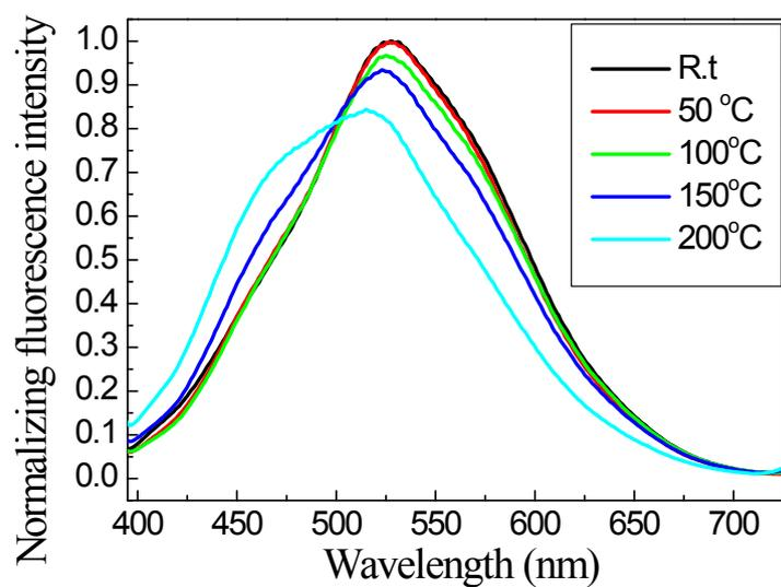
Fig. S8. Fluorescent spectra of the TTPT before and after annealing at different temperatures for 30 min in air. ( $1.0 \text{ mg mL}^{-1}$  in THF,  $\lambda_{\text{ex}}=370 \text{ nm}$ .)
