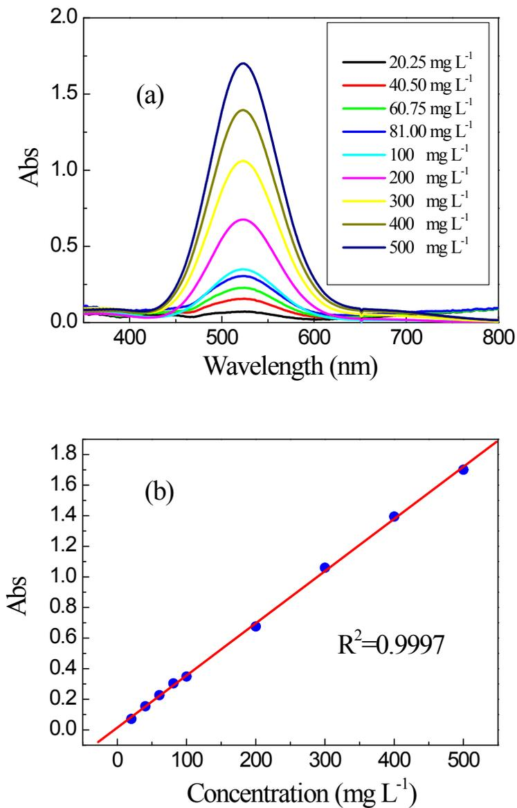
Fig. S12 (a) Calibration plot of standard iodine by UV-Vis spectra in cyclohexane solution. (b) The fitting of Abs value vs concentration of I<sub>2</sub> with the relatively good linearity satisfies Lambert-Beer Law.
