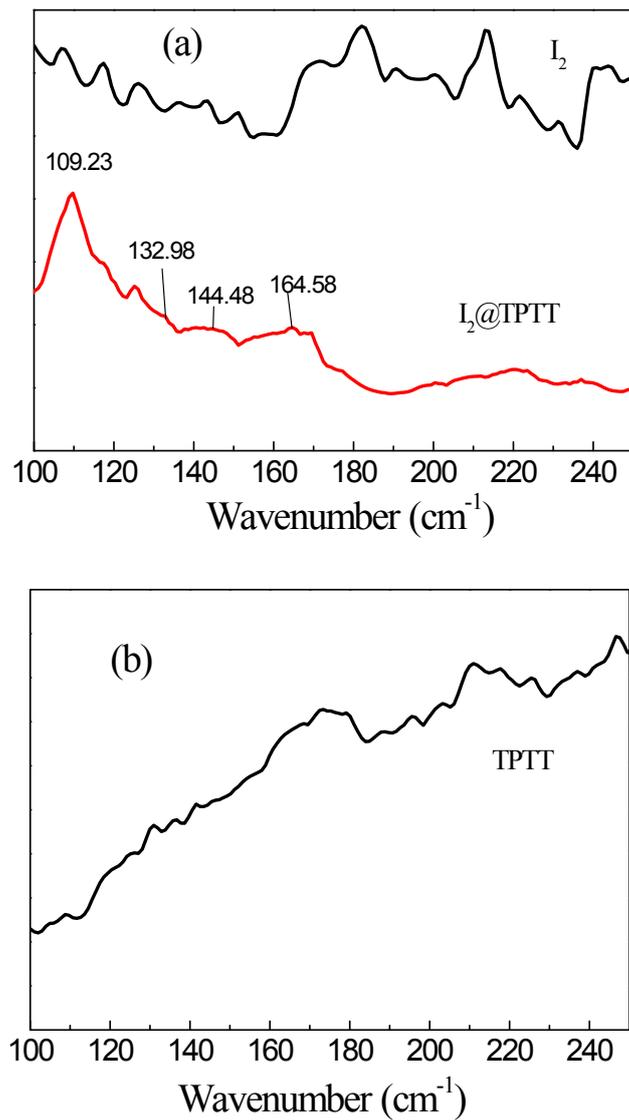
Fig. S10 Raman spectrums of (a)  $I_2$ , iodine-loaded TTPT ( $I_2@TTPT$ ) and (b) TTPT.
