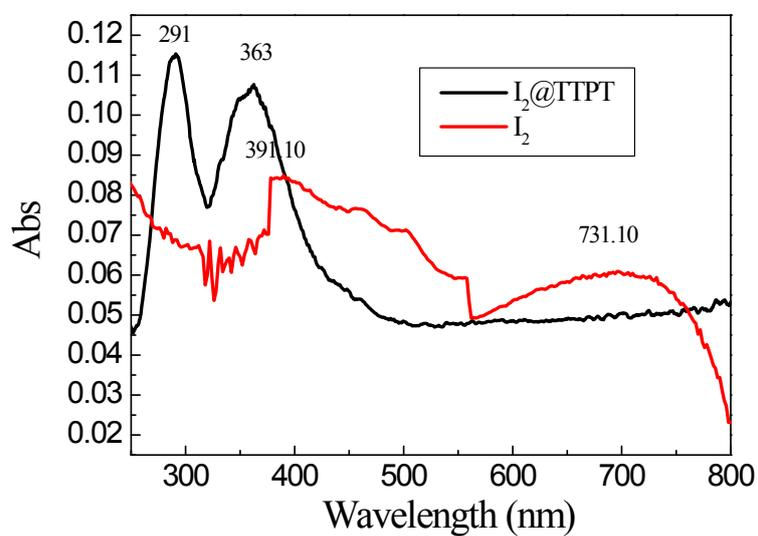
Fig. S9 UV-vis spectra of  $\text{I}_2$ @TTPT and  $\text{I}_2$ .
