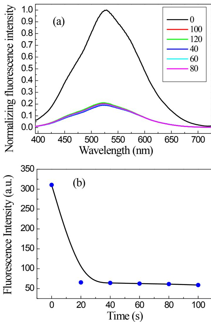
Fig. S6. (a) Fluorescence spectral changes of TTPT dispersed in THF upon addition of o-NP ( $5.0 \times 10^{-5}$  mol L<sup>-1</sup>). (b) The curve of (b) is the evolution of maximum fluorescence intensity as a function of time. The excitation wavelength was 370 nm.
