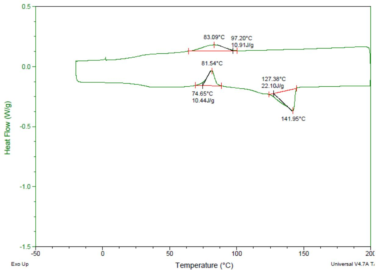
**Figure S-10.** DSC thermogram of phenyl acrylate adduct of 4 % thiol-PL copolymer showing the second thermal cycle. 5 °C/min, -10 °C to 200 °C.
