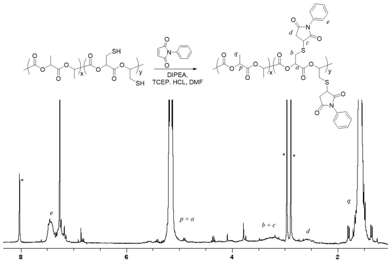
**Figure S-12.**  $^1\text{H}$  NMR spectrum (300 MHz,  $\text{CDCl}_3$ ) of *N*-phenylmaleimide adduct of 4 % thiol-PL. \* residual DMF
