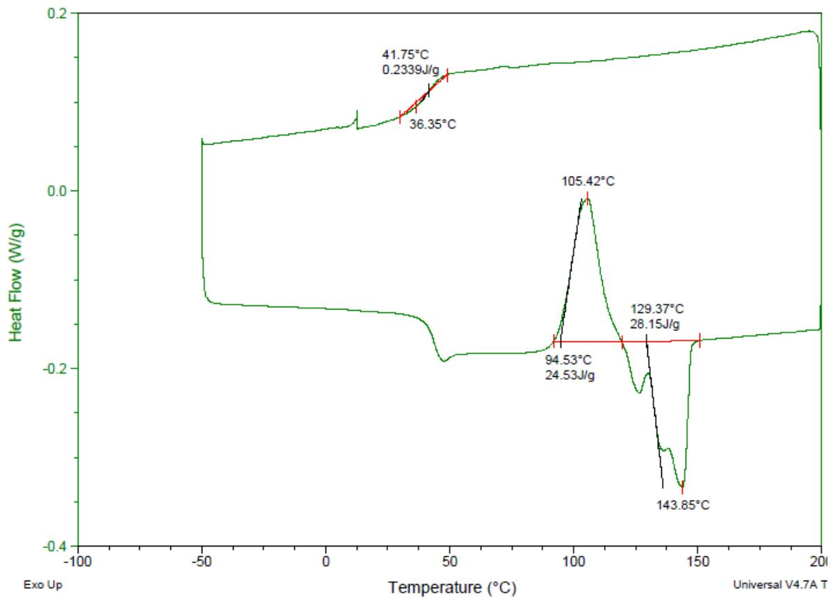
**Figure S-6.** DSC thermogram of 5 % MBT-PL obtained by copolymerization of the cis stereoisomer of monomer **1** with L-lactide. 5 °C/min, -50 °C to 200 °C.
