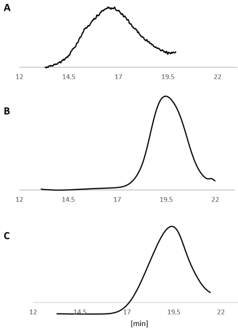
**Figure S-3.** GPC. A, 5 % MBT-PL obtained by copolymerization of trans MBT-lactide with L-lactide. B, 4 % thiol-PL. C, 4 % thiol-PL-phenylacrylate adduct.
