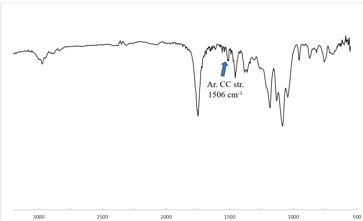
**Figure S-4.** IR spectrum of 5 % MBT-PL.
