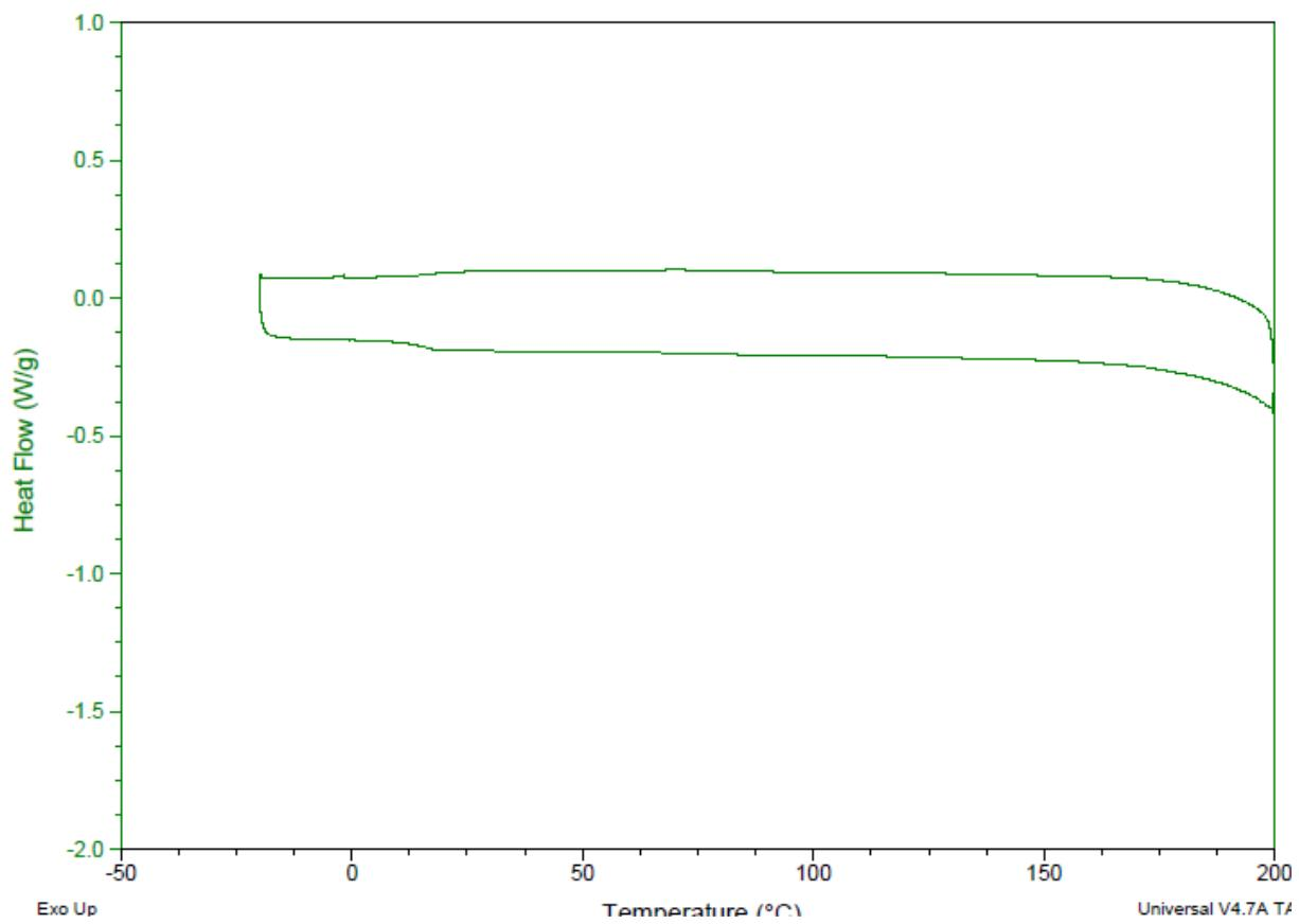
**Figure S-9.** DSC thermogram of 4 % thiol-PL showing the second thermal cycle. 5 °C/min, -20 °C to 200 °C.
