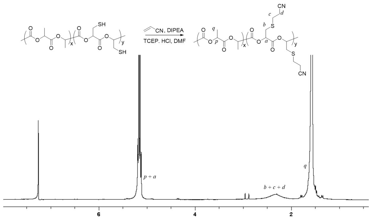
**Figure S-11.**  $^1\text{H}$  NMR spectrum (300 MHz,  $\text{CDCl}_3$ ) of acrylonitrile adduct of 4 % thiol-PL.
