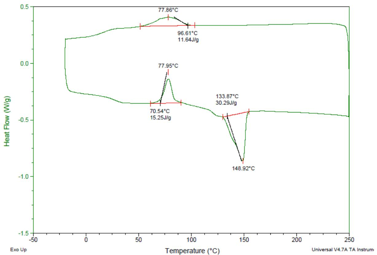
**Figure S-7.** DSC thermogram of 5 % MBT-PL obtained by copolymerization of the trans stereoisomer of monomer **1** with L-lactide. 5 °C/min, -10 °C to 250 °C
