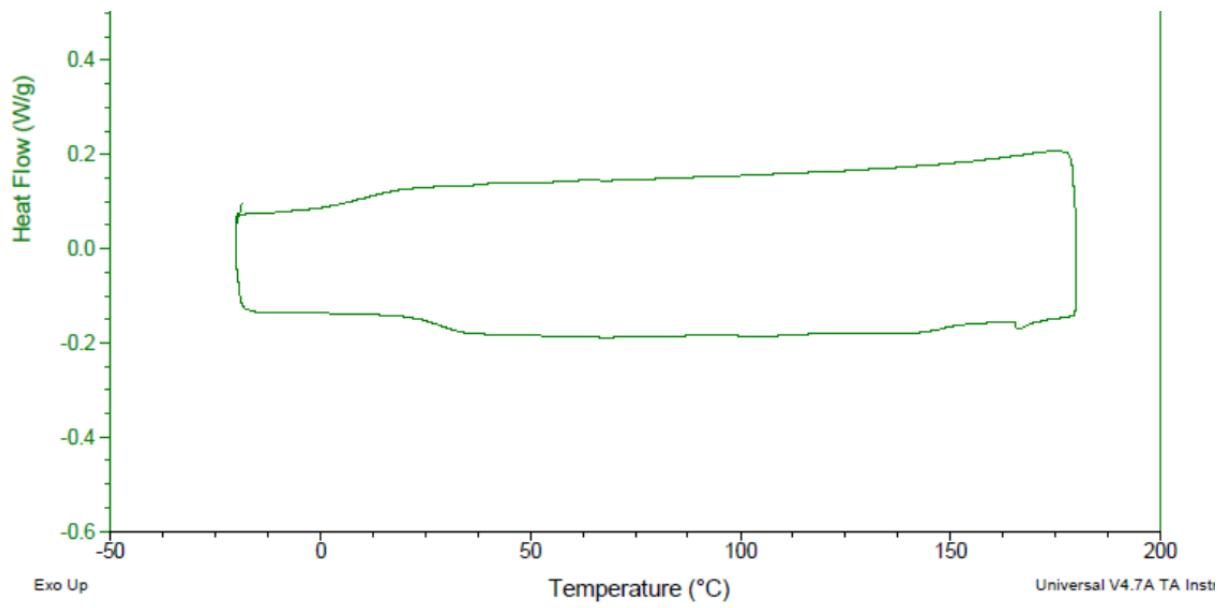
**Figure S-8.** DSC thermogram of 5 % MBT-PL obtained by copolymerization of the diasteriomer mixture of monomer **1** with L-lactide. 5 °C/min, -10 °C to 180 °C
