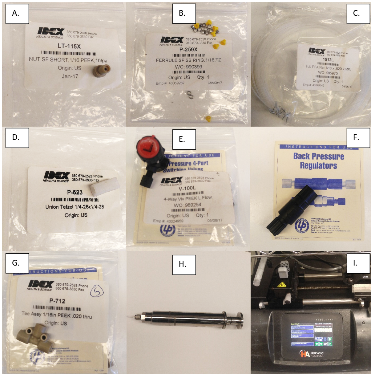
Figure S1. A. PEEK super-flangeless nut B. Yellow super-flangeless ferrule with corresponding stainless steel ferrule ring -- sold separately. C. 0.02 ID PFA tubing D. Standard union, Tefzel E. 4-way "L" switch valve F. back pressure regulator, 40 PSI (part number P-785) G. Static mixing Tee H. 20 mL stainless steel syringe I. Ph.D Ultra syringe pump
