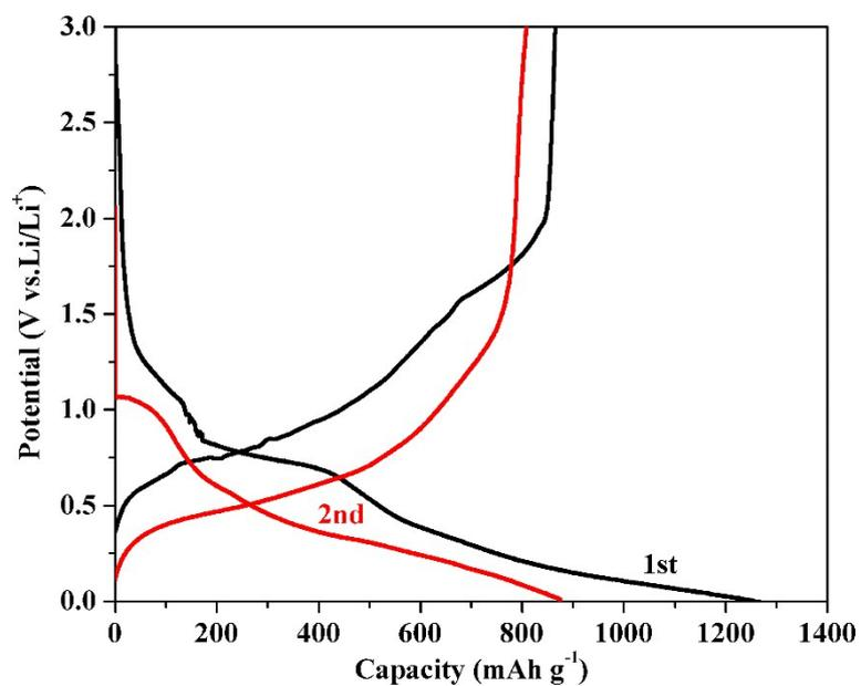
Fig. S11 Discharge-charge profiles for 1<sup>st</sup> and 2<sup>nd</sup> cycle of SnO<sub>2</sub> NPs.
