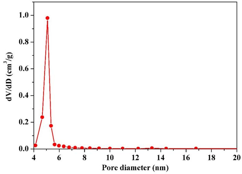
Fig. S5 Pore size distribution curve of MCF
