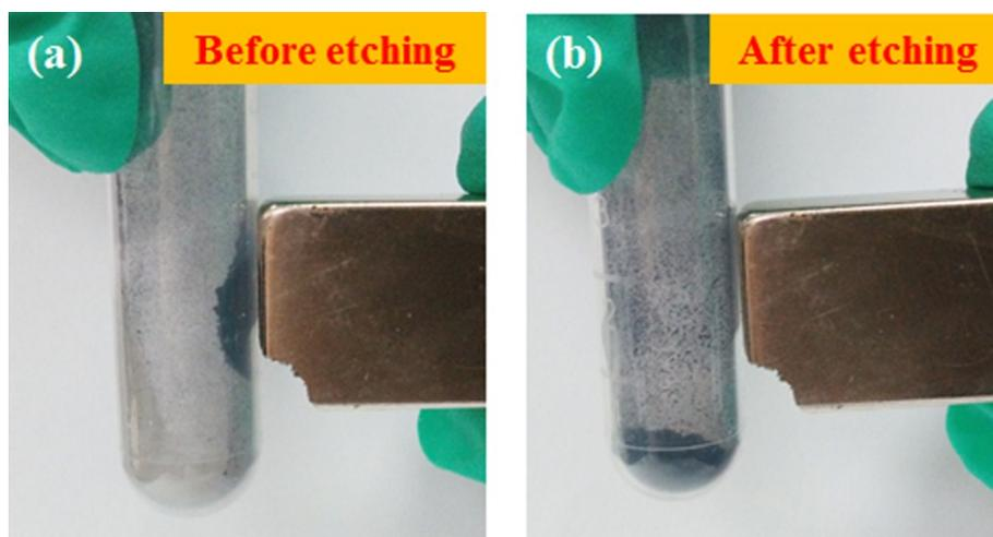
**Fig. S2** Photographs of the magnetism change of the graphene@Fe<sub>3</sub>O<sub>4</sub>@C composite before and after acid etching.
