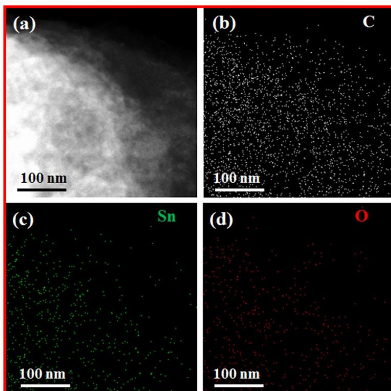
Fig. S12 STEM image of MCF@SnO<sub>2</sub> electrode after 200 cycles at 1 A g<sup>-1</sup> (a) and the corresponding EDX elemental mapping of C, Sn and O at the region in (a), respectively (b-d).
