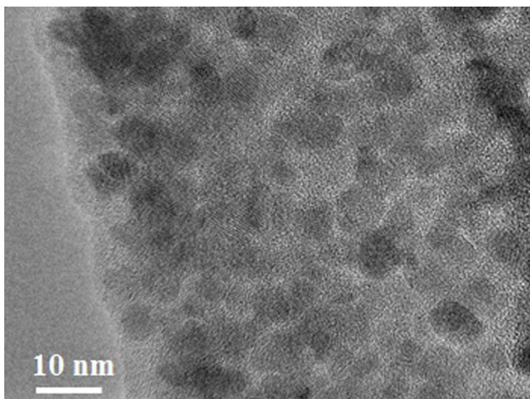
**Fig. S1** TEM image of the graphene@Fe<sub>3</sub>O<sub>4</sub>@C composite
