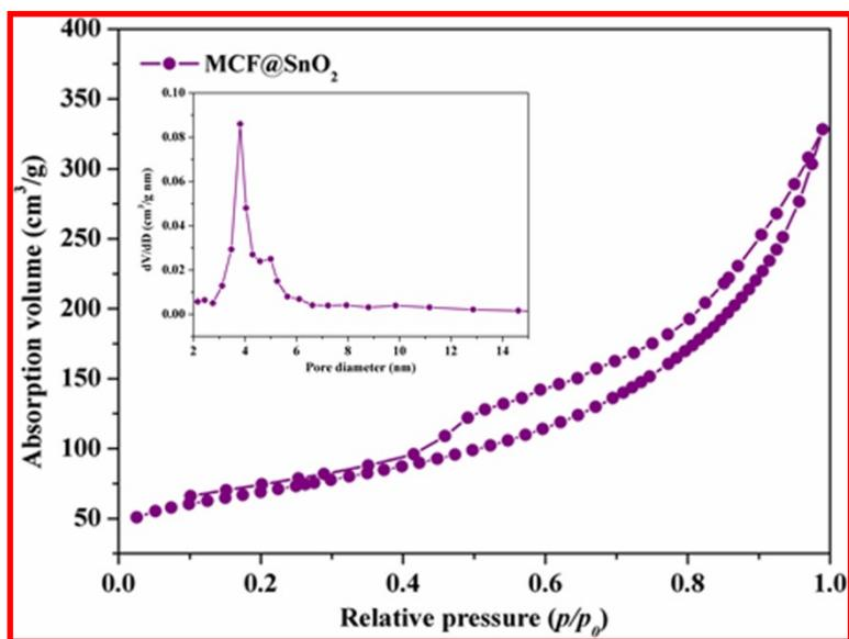
**Fig. S8** Nitrogen adsorption/desorption isotherm of MCF@SnO<sub>2</sub>, inset shows the corresponding pore size distribution curve.
