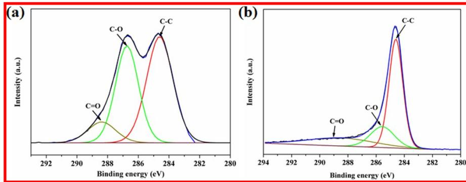
Fig. S6 High-resolution XPS spectra of C 1s of GO (a) and MCF (b).
