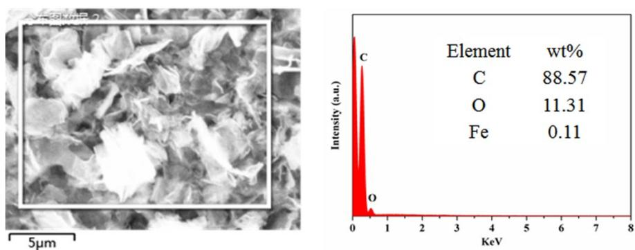
**Fig. S4** Energy dispersion X-ray (EDX) spectrum of the graphene@Fe<sub>3</sub>O<sub>4</sub>@C after acid etching
