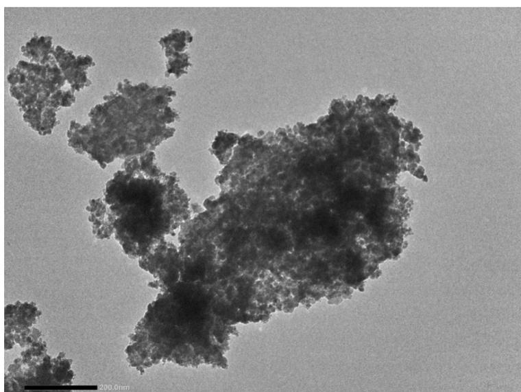
**Fig. S10** TEM image of the synthesized SnO<sub>2</sub> nanoparticles
