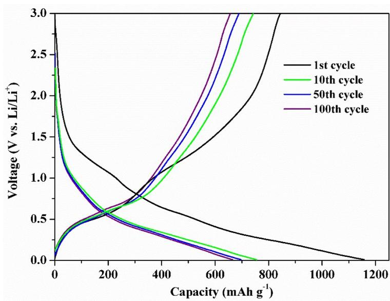
**Fig. S9** Discharge-charge profiles for 1<sup>st</sup> and 50<sup>th</sup> and 100<sup>th</sup> cycle of MCF@SnO<sub>2</sub> at a current density of 1 A g<sup>-1</sup>.
