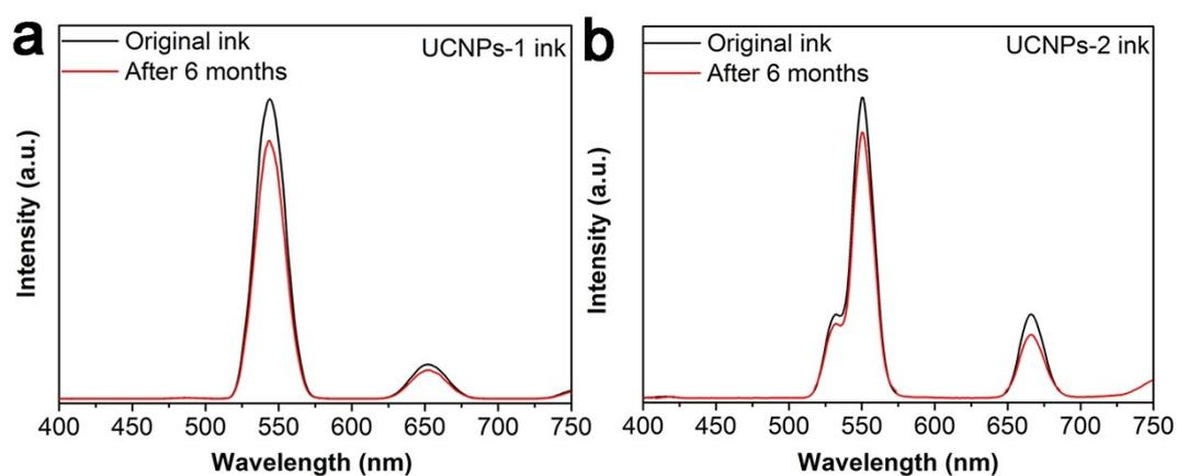
**Fig. S5** Luminescence spectra of UCNPs-1 ink (a) and UCNPs-2 ink (b) before and after storage for 6 months.
