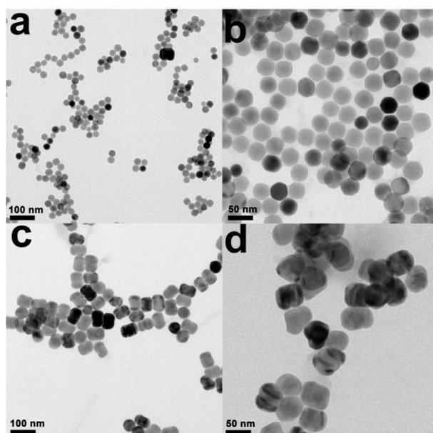
**Fig. S2** TEM images of NaYF<sub>4</sub>:18%Yb,2%Er core nanoparticles (a, b) and NaYF<sub>4</sub>:Yb,Er@NaYF<sub>4</sub>:Yb@NaNdF<sub>4</sub>:Yb@NaYF<sub>4</sub>:Yb core-shell nanoparticles (c, d).
