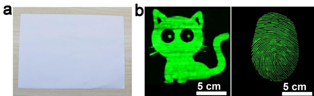
**Fig. S7** (a) Image of the paper encrypted with UCNPs-2 ink under ambient light. b) Images of the paper encrypted with UCNPs-2 ink under 808 nm CW laser.
