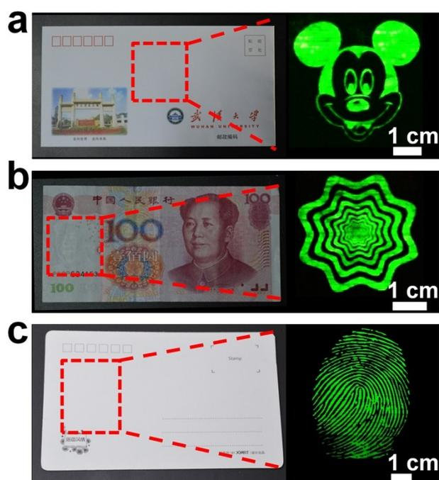
**Fig. S8** Images of envelope (a), banknote (b) and postcard (c) encrypted with UCNPs-2 ink under 808 nm CW laser.
