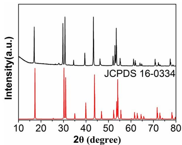
**Fig. S3** XRD pattern of NaYF<sub>4</sub>:20%Yb,2%Ho nanoparticles.
