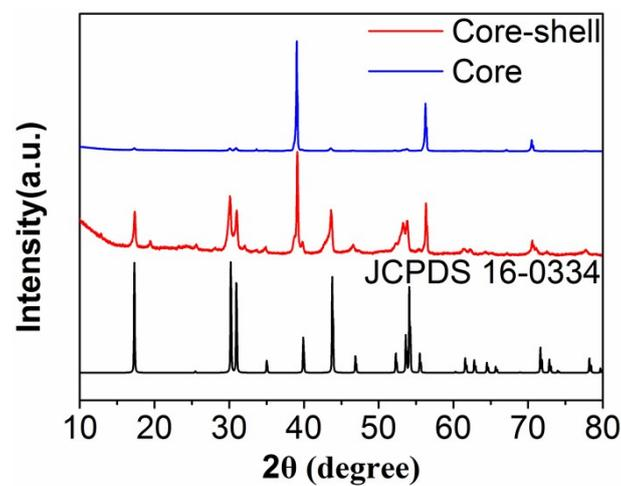
**Fig. S4** XRD patterns NaYF<sub>4</sub>:18%Yb,2%Er core nanoparticles and NaYF<sub>4</sub>:Yb,Er@NaYF<sub>4</sub>:Yb@NaNdF<sub>4</sub>:Yb@NaYF<sub>4</sub>:Yb core-shell nanoparticles.
