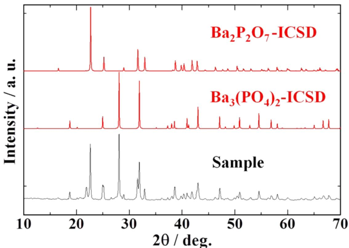
**Figure S1.** XRD patterns of the  $\sigma$ –(Ba<sub>0.99</sub>Eu<sub>0.03</sub>)<sub>2</sub>P<sub>2</sub>O<sub>7</sub> phosphor synthesized by conventional solid state reaction.
