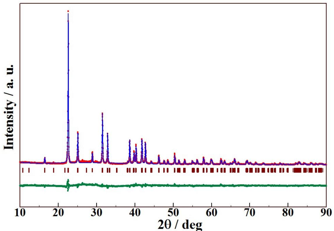
**Figure S3.** Observed (red + symbol), calculated (blue solid line) and difference (green solid line) patterns for the Rietveld refinement from the X-ray powder diffraction data of the synthesized  $\sigma$ – $(\text{Ba}_{0.72}\text{Eu}_{0.03}\text{Mg}_{0.30})_2\text{P}_2\text{O}_7$ .
