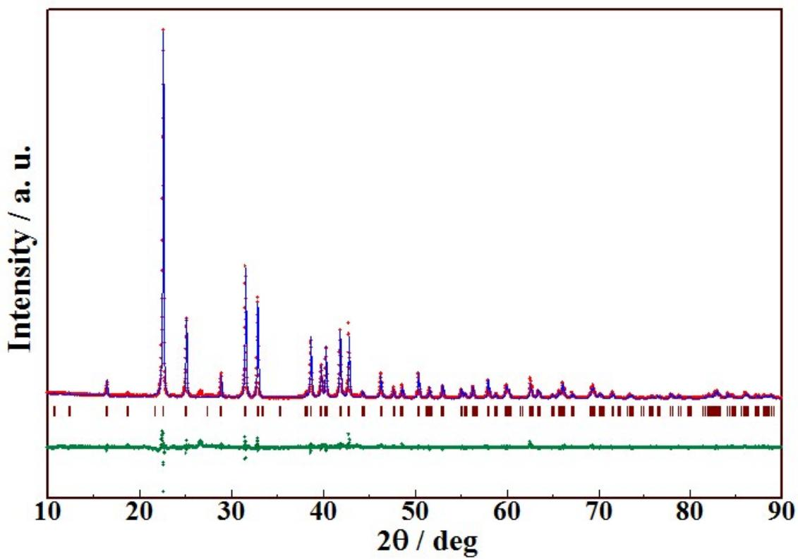
**Figure S2.** Observed (red + symbol), calculated (blue solid line) and difference (green solid line) patterns for the Rietveld refinement from the X-ray powder diffraction data of the synthesized  $\sigma$ –(Ba<sub>0.97</sub>Eu<sub>0.03</sub>)<sub>2</sub>P<sub>2</sub>O<sub>7</sub>.
