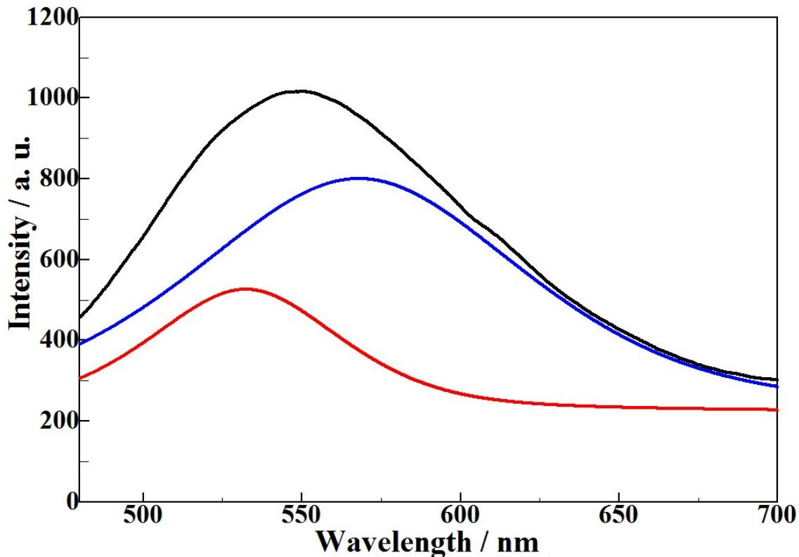
**Figure S4.** Observed (black line), calculated (red and blue line) patterns for the Fit Peak refinement from emission spectrum data of the synthesized  $\sigma$ - $(\text{Ba}_{0.72}\text{Eu}_{0.03}\text{Mg}_{0.30})_2\text{P}_2\text{O}_7$ . Calculated emission spectra corresponding to  $\text{BaO}_9$  and  $\text{BaO}_7$  polyhedral states are plotted by red or blue solid line, respectively.
