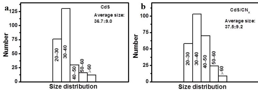
Fig. S4. The bar charts of the size distributions of (a) CdS and (b) CdS/CN<sub>x</sub> based on 260 CdS nanorods.
