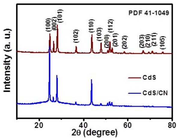
**Fig. S2.** XRD pattern for CdS nanorods and CdS/CN<sub>x</sub>.
