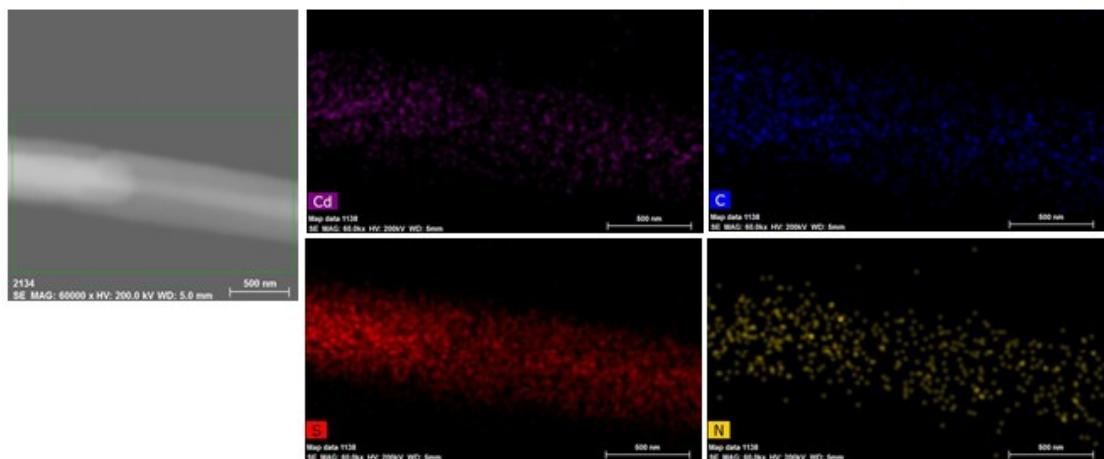
**Fig. S7.** EDS mapping of CdS/CNx: Cd (purple), S (red), C (blue) and N (yellow). Scale bare is 500 nm for all images.
