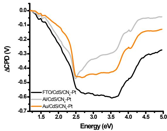
**Fig. S17.** Surface photovoltage spectra of CdS/CN<sub>x</sub>-Pt (solid lines) on gold, aluminum and FTO substrates.
