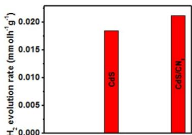
**Fig. S11.**Photocatalytic H<sub>2</sub>-production rate of CdS and CdS/CN<sub>x</sub> catalysts.
