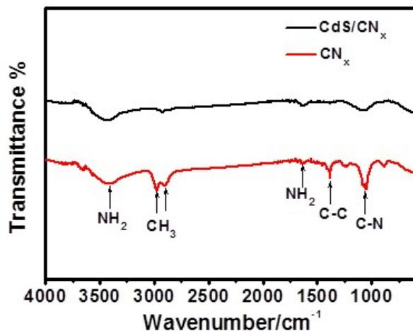
**Fig. S5.** FTIR spectra of CN<sub>x</sub> and CdS/CN<sub>x</sub>.
