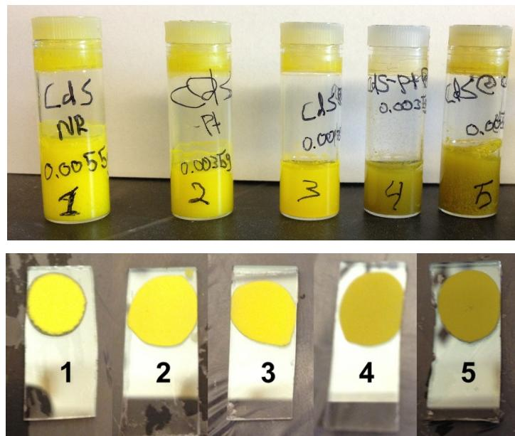
**Fig. S13. (Top)** 2 mg/mL sample dispersions after 1 hour of ultrasonication. **(Bottom)** Films of CdS nanorod samples on FTO coated glass. Thicknesses ranged from 2.2 - 4  $\mu\text{m}$  based on profilometry measurements.
