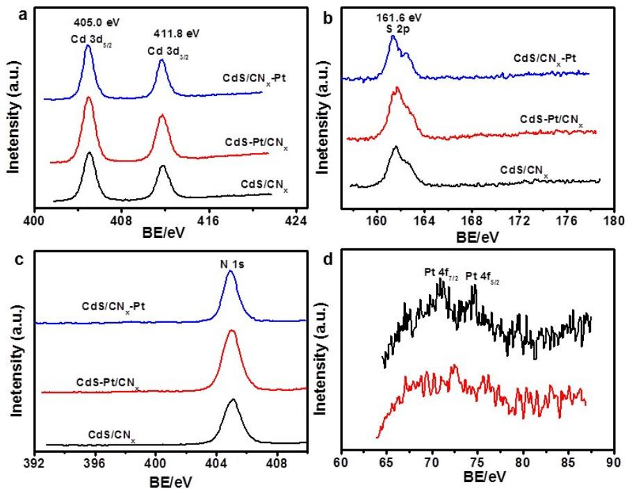
**Fig.S6.** XPS spectra of the as-obtained sample (a) Cd3d; (b) S2p; (c) N1s; (d) Pt4f.
