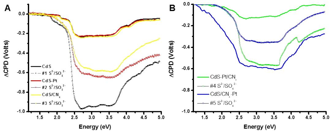
**Fig. S16.** Photovoltage spectra before (solid lines) and after (circles) addition of 0.35 M Na<sub>2</sub>S and 0.25 M Na<sub>2</sub>SO<sub>4</sub>.
