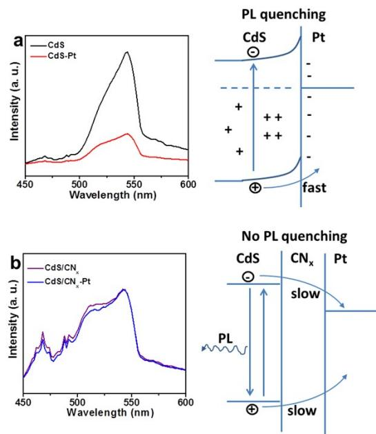
**Fig. S18.** Photoluminescence spectra of CdS, CdS-Pt, CdS/CNx and CdS/CNx-Pt at room temperature with an excitation wavelength of 400 nm and the schematic diagram for PL of CdS-Pt and CdS/CNx-Pt, respectively.
