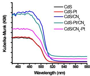
**Fig. S10.**UV-vis spectra of CdS, CdS-Pt, CdS/CN<sub>x</sub>, CdS-Pt/CN<sub>x</sub> and CdS/CN<sub>x</sub>-Pt catalysts.
